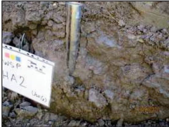
Figure 3.2 Soil Sampling of distinct soil layer using Push Tube
