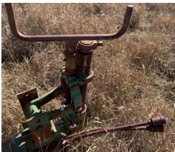
Figure 69. A close-up view of the hydraulic fixings of the disc plough (WS20).
