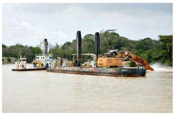
Figure C.2.3.4 Typical backhoe dredge (mechanically excavates material using a bucket at the end of the excavator arm and places it in a self-propelled hopper barges which are moored alongside for transport of the dredged material to the DMPA. The dredger is anchored using spud piles and manoeuvred by a tug).
