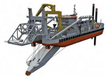
Figure C.2.3.3 Typical cutter suction dredger (rotating cutter head loosens material which is drawn up a pipe located as slurry. The slurry is pumped through floating/submerged pipeline to the placement area. The dredger is manoeuvred using the spud piles at the bow and an anchor and wire system from the stern).
