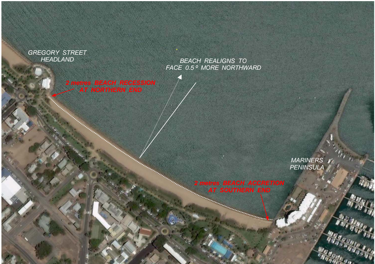
Figure 5.4 : Predicted Impact on the Beach between Mariners Peninsula & Gregory Street (Beach re-alignment is drawn conceptually and rotation is not necessarily to scale)
