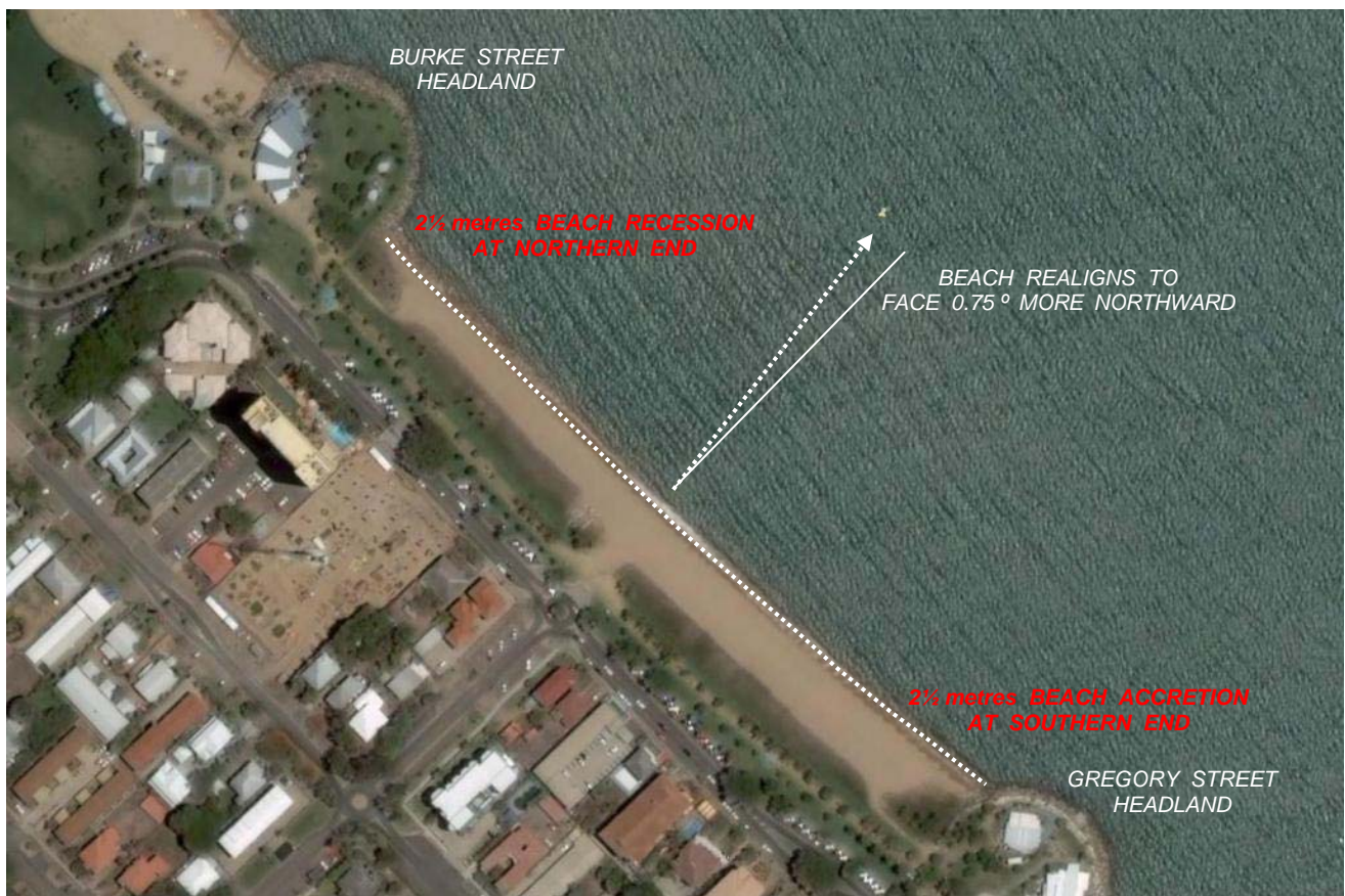
Figure 5.5 : Predicted Impact on the Beach between Gregory Street & Burke Street (Beach re-alignment is drawn conceptually and rotation is not necessarily to scale)
