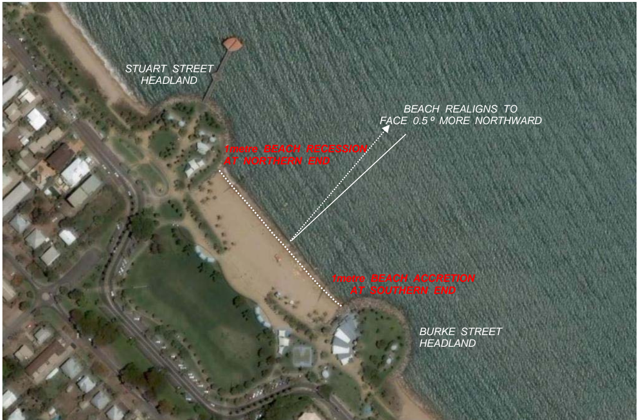
Figure 5.6 : Predicted Impact on the Beach between Burke Street & Stuart Street (Beach re-alignment is drawn conceptually and rotation is not necessarily to scale)
