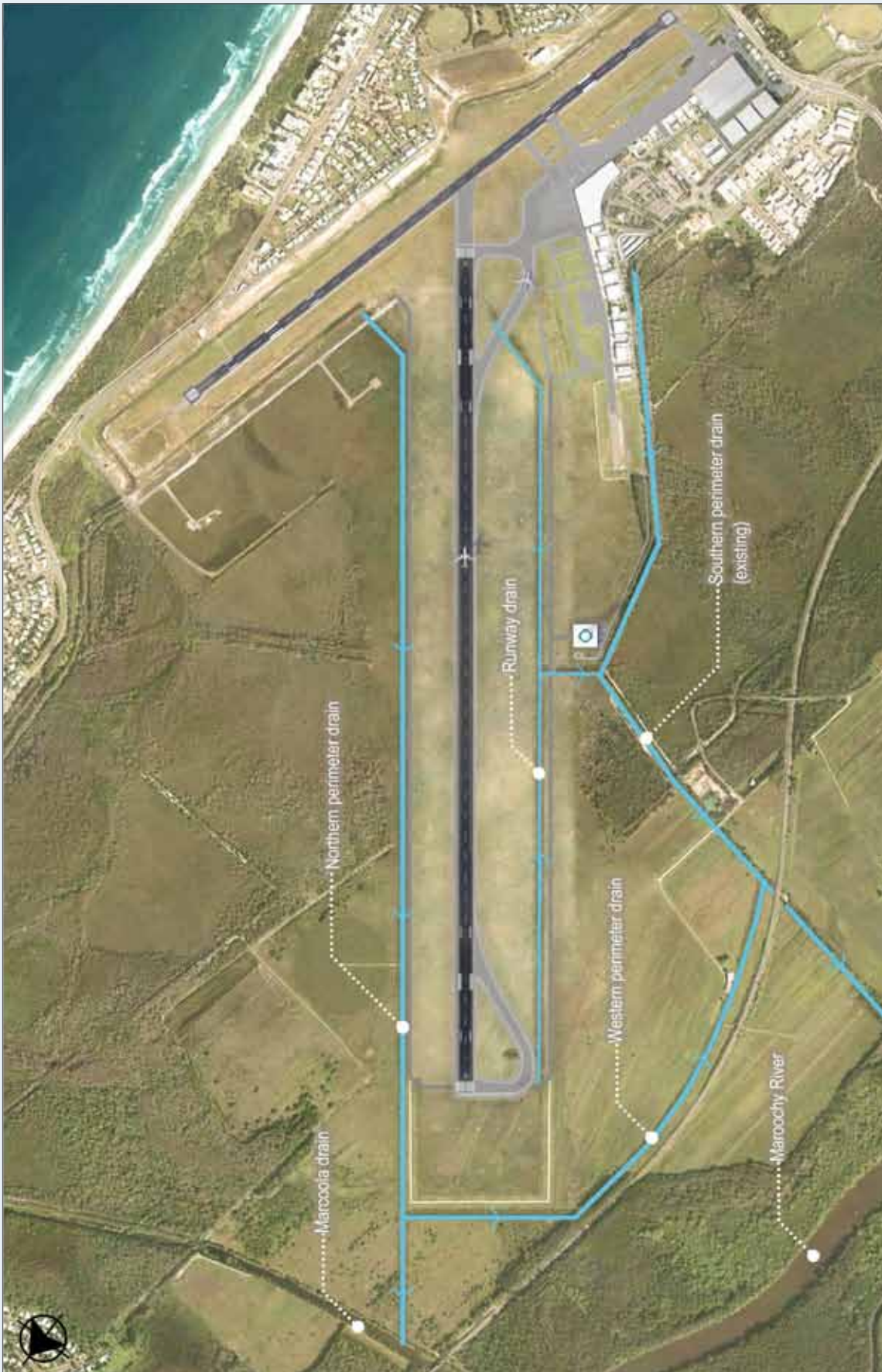
Figure 5.1g: Proposed drainage infrastructure
