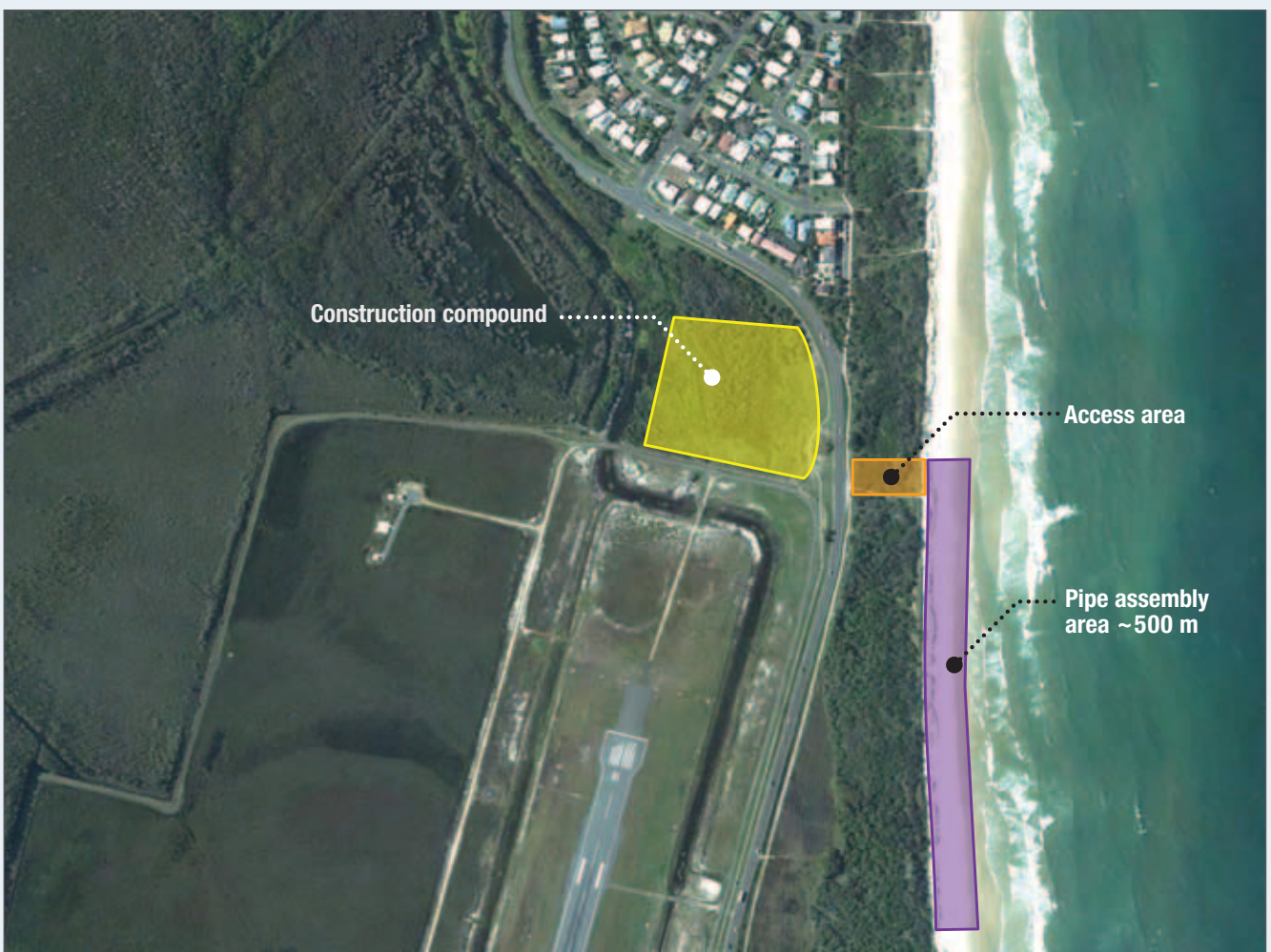
Figure 15.5a: Indicative areas for the dredge pipe assembly
