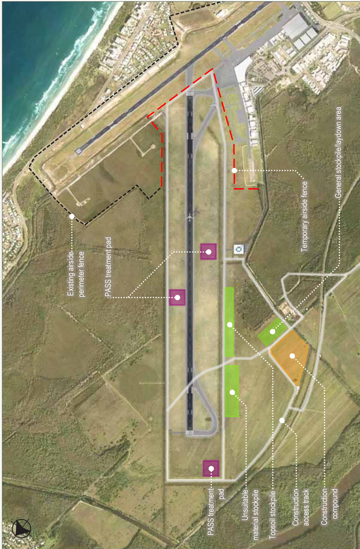
Figure 5.3d: PASS treatment pads and stockpile areas
