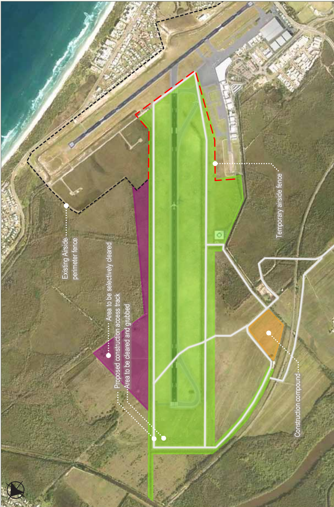
Figure 5.3c: On-site construction access roads and clearing areas
