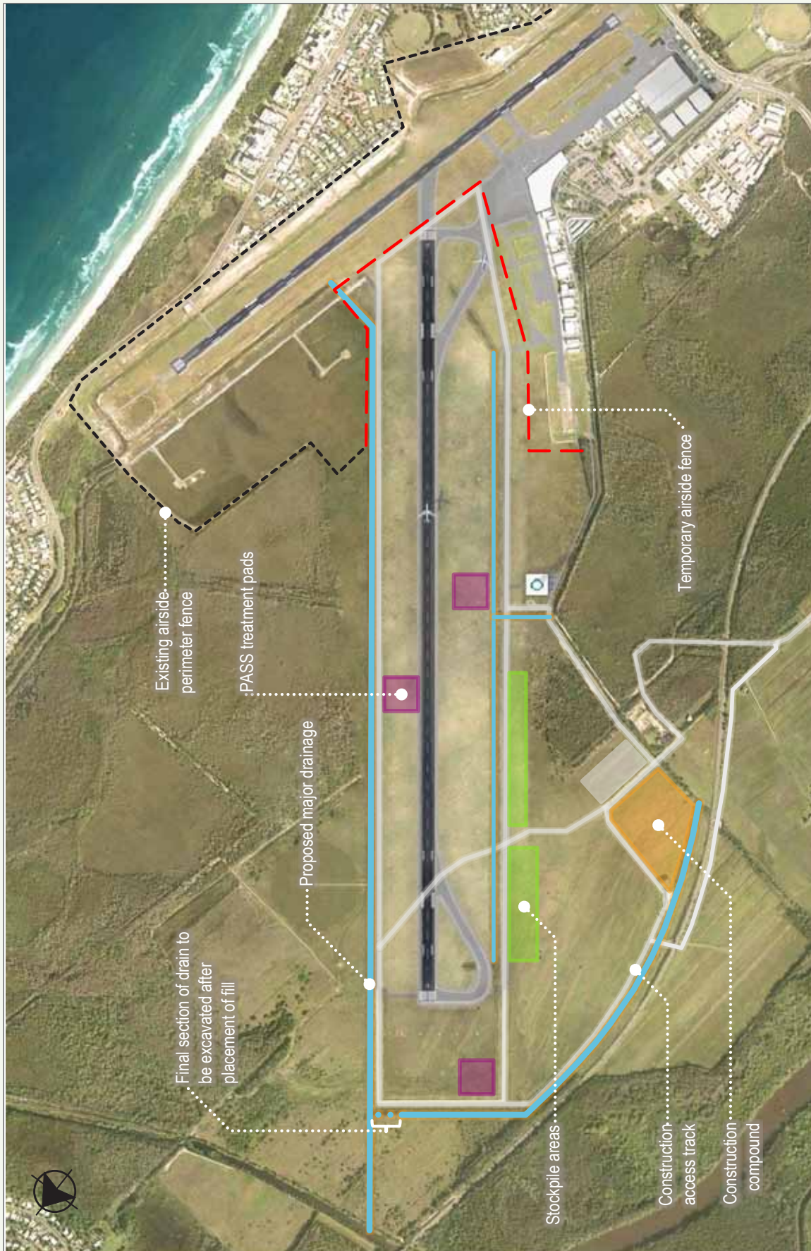
Figure 5.3e: Major drainage layout
