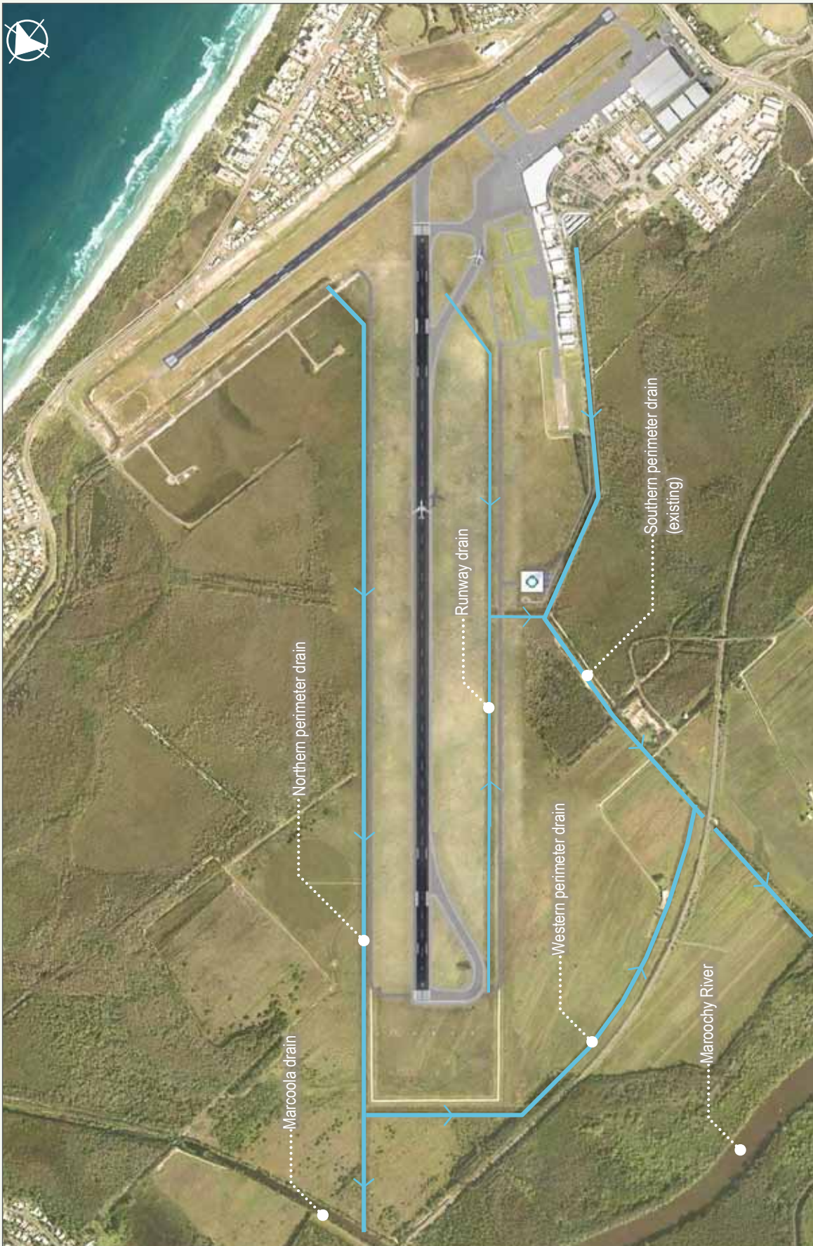
Figure 4.9a: Indicative drainage layout for the Project
