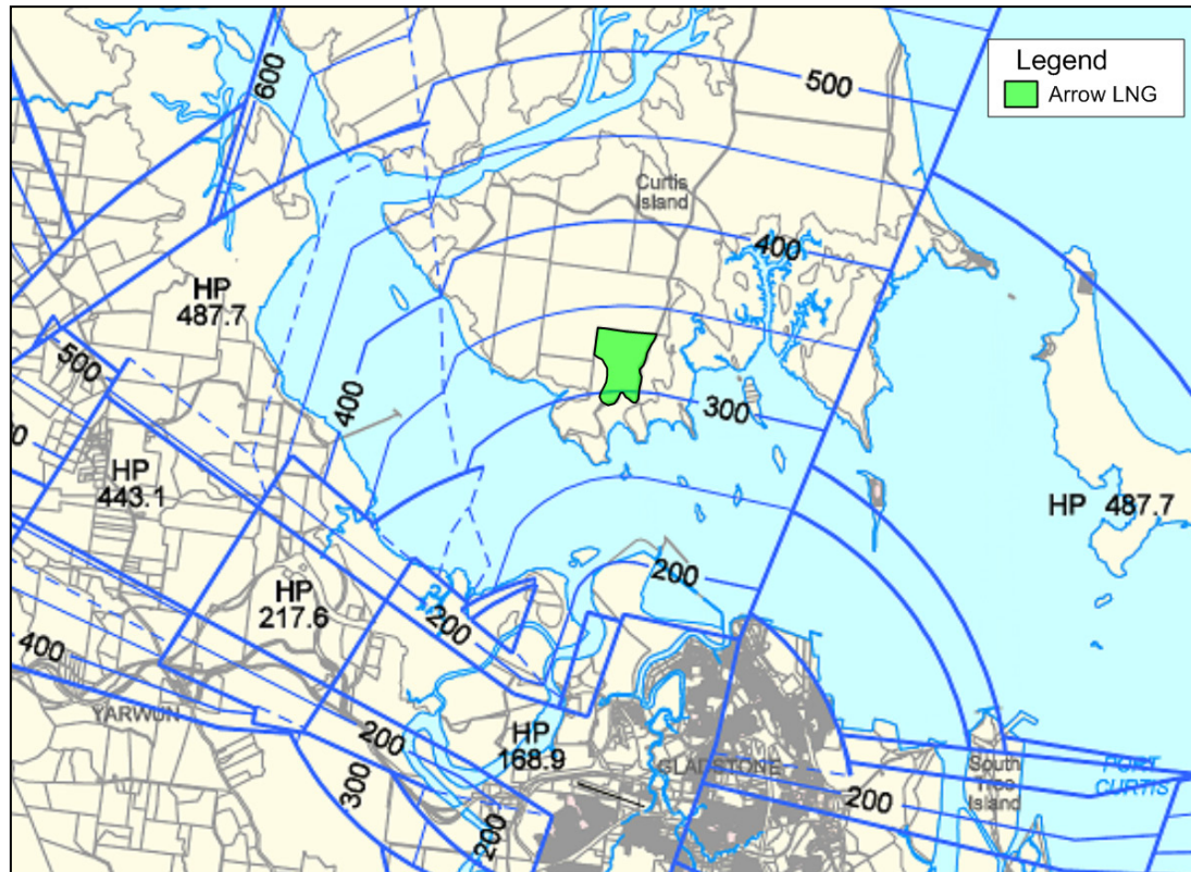
Figure 2 PANS-OPS surface for Arrow LNG Plant site
