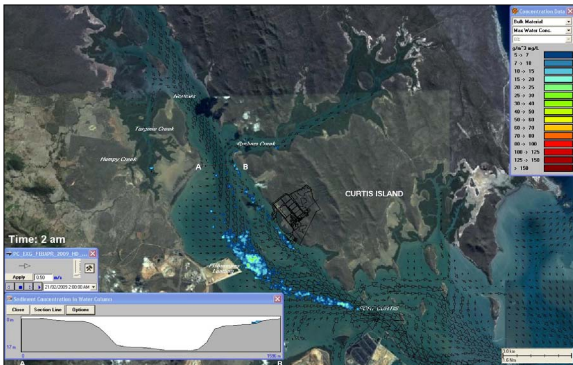
Figure 19: Snapshot of the maximum predicted suspended sediment concentration (above background) at any depth level generated from losses by the BHD when trenching on the east side of the Narrows section during a sample February 2009 flood (top) and ebb (bottom) spring tide.
