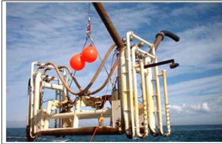
Figure 8: Photograph of the “Sumartran Tiger” Bi-directional jet trenching machine (20” – 42” outer diameter pipeline burials) (Source: Xodus Group Pty. Ltd., 2009).
