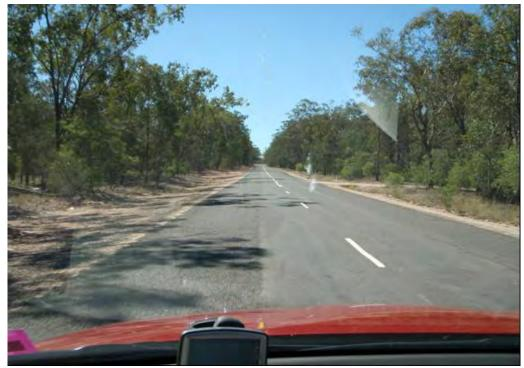
Figure 2.4 Kogan-Condamine Road – unsealed shoulders (state controlled)
