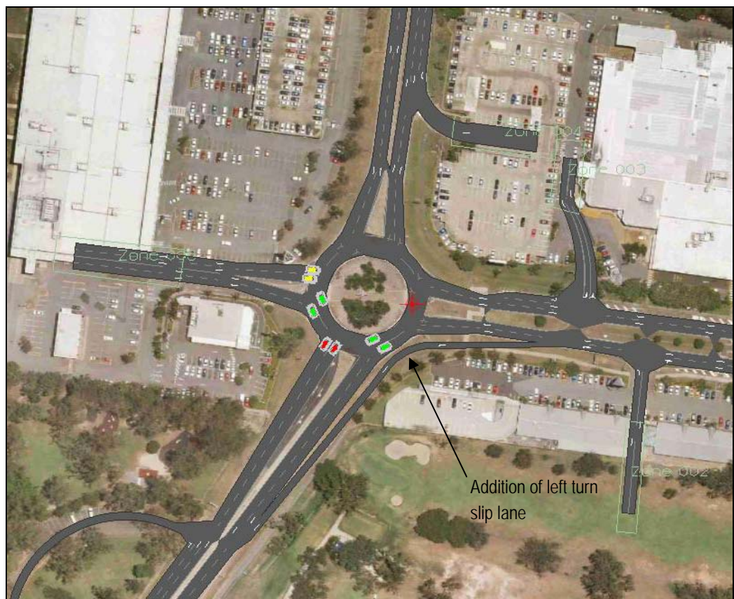
Figure 4-2 Model 2 – Upgraded Roundabout
