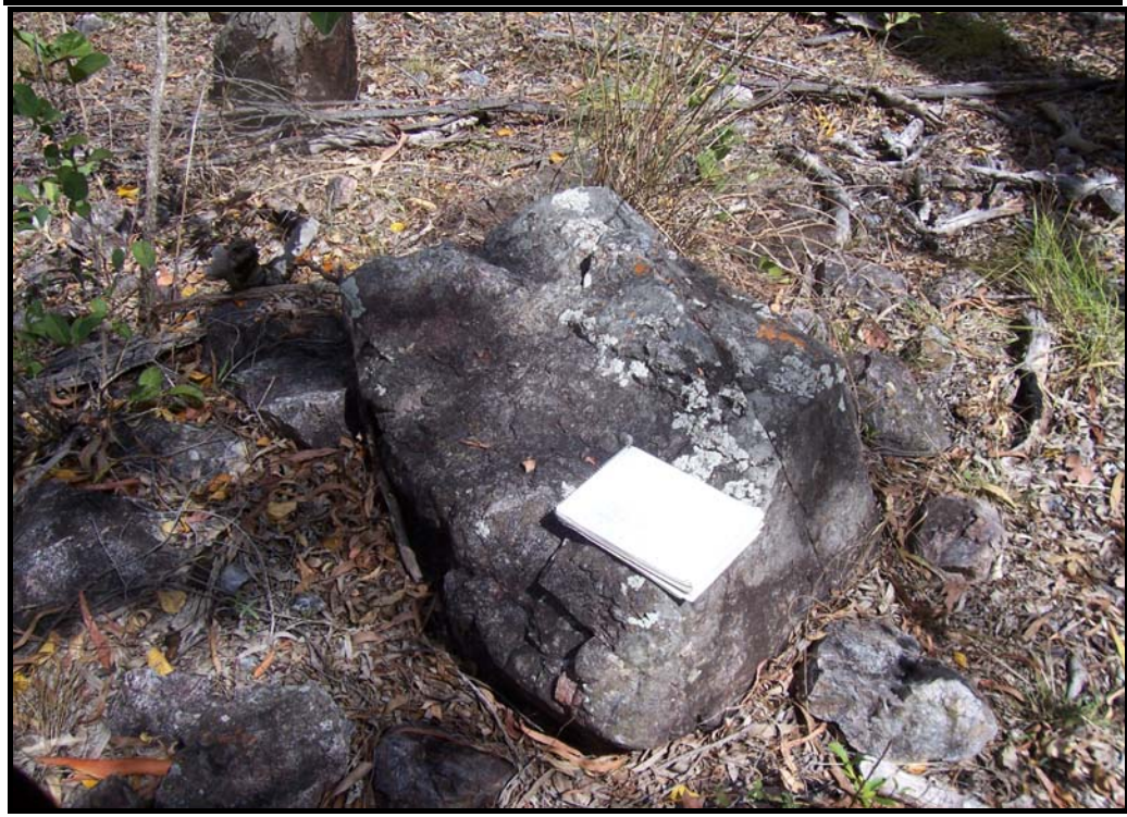
Plate 5.3.3 Outcrop of Dark Grey Blocky Indurated Mudstone of the Wandilla Formation, Curtis Island
