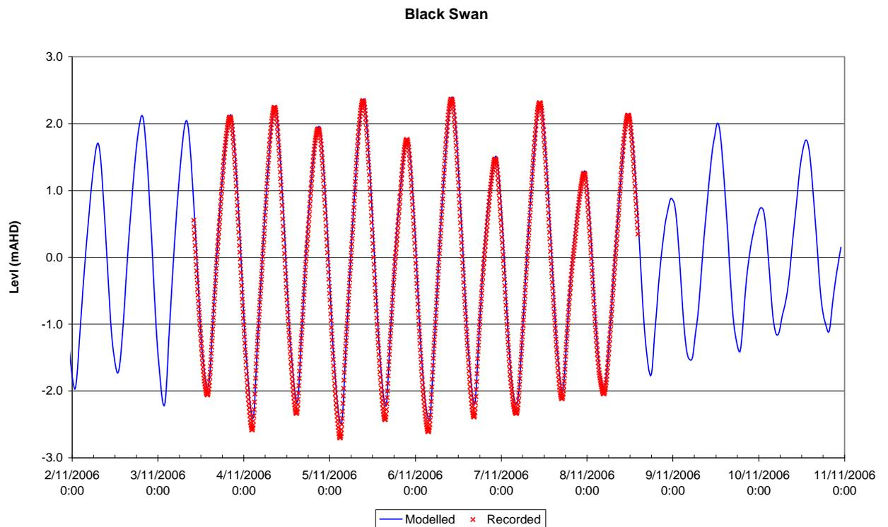
Figure 2-19 Water Level Calibration – Black Swan Inlet, November 2006
