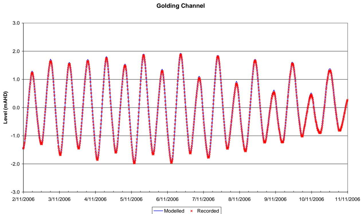
**Figure 2-23 Water Level Calibration – Golding Channel, November 2006**
