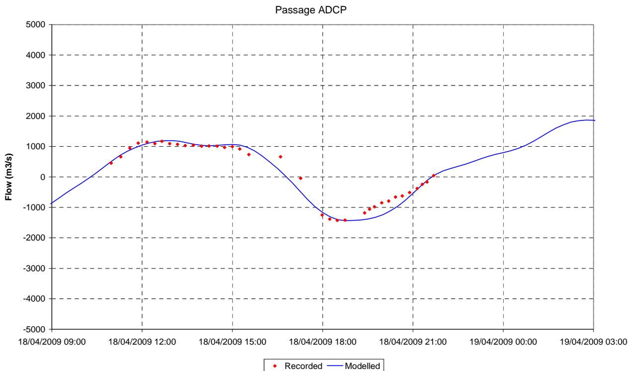
**Figure 2-51 Flow Validation – “Curtis” Channel, April 2009 (Neap Tide)**
