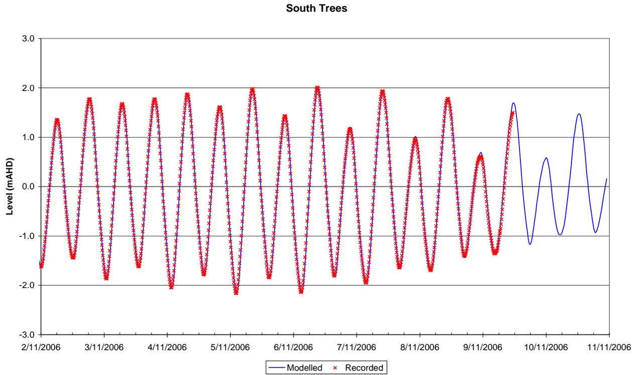
Figure 2-20 Water Level calibration – South Trees, November 2006
