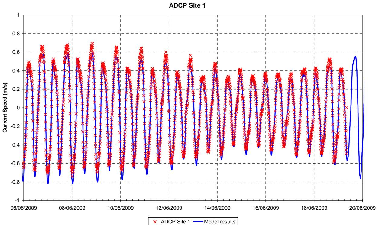
Figure 2-57 Current Speed – GHD ADCP Site 1, June 2009
