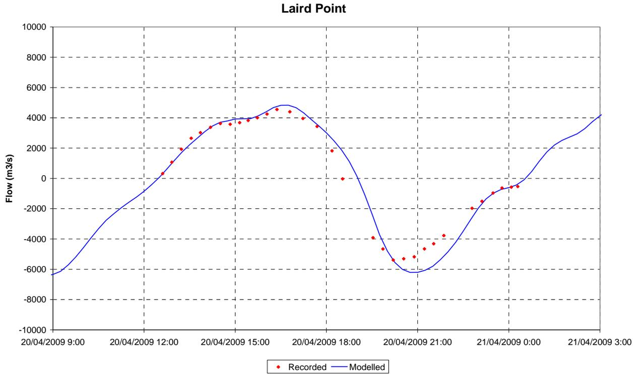
**Figure 2-50 Flow Validation – Laird Point, April 2009 (Neap Tide)**
