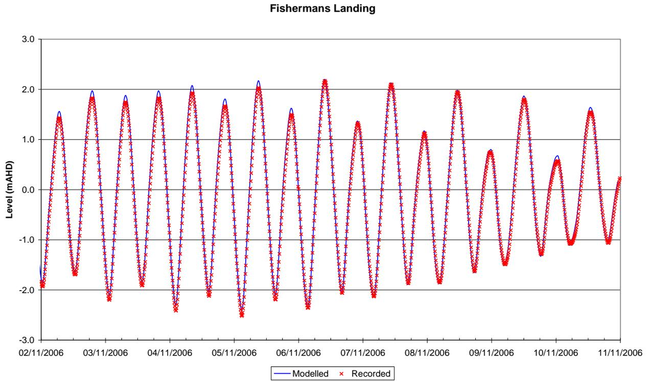
Figure 2-18 Water Level Calibration – Fisherman’s Landing, November 2006
