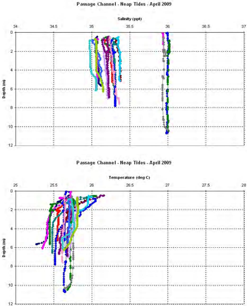
Figure A-1 "Curtis" Channel Salinity and Temperature Profiles (18-19 April 2009)
