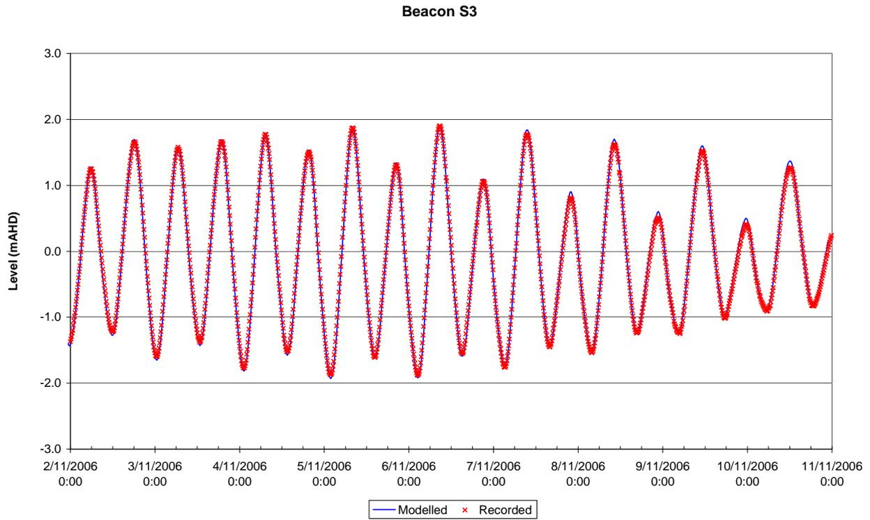
**Figure 2-26 Water Level Calibration – Beacon S3, November 2006**
