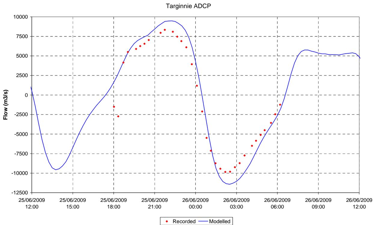
Figure 2-55 Flow Validation – Targinnie Channel, June 2009
