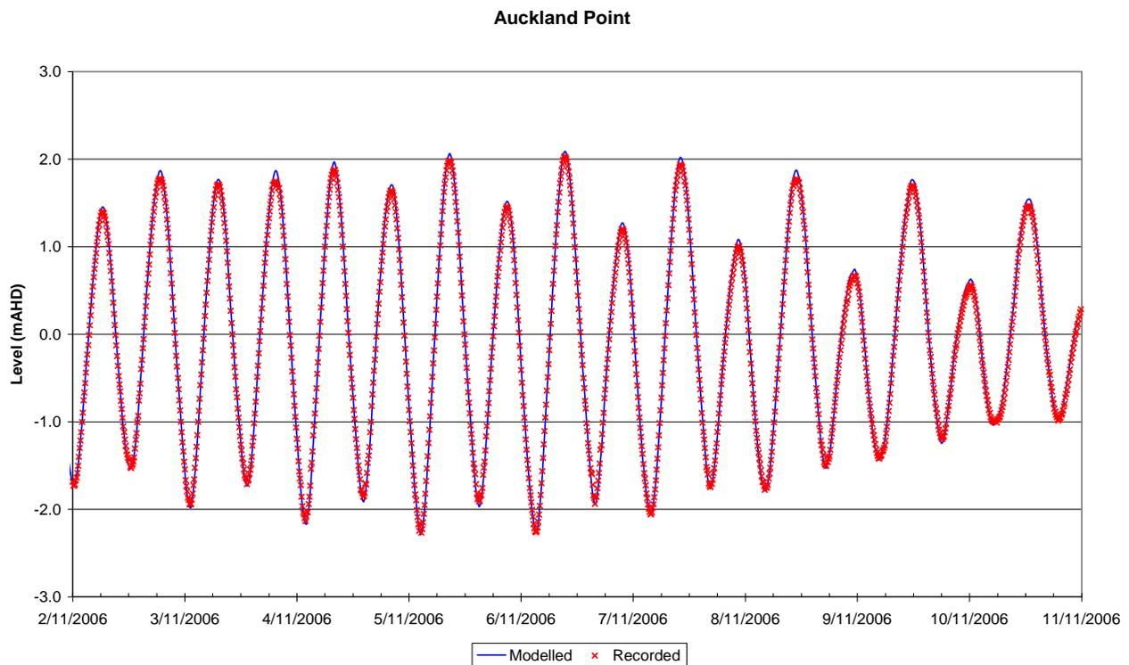
Figure 2-21 Water Level calibration – Auckland Point, November 2006
