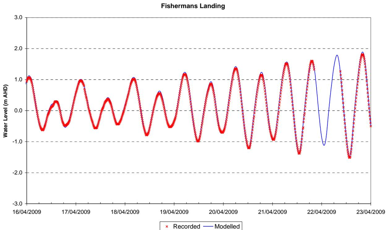
**Figure 2-39 Water Level Validation – Fisherman’s Landing, April 2009 (Neap Tide)**
