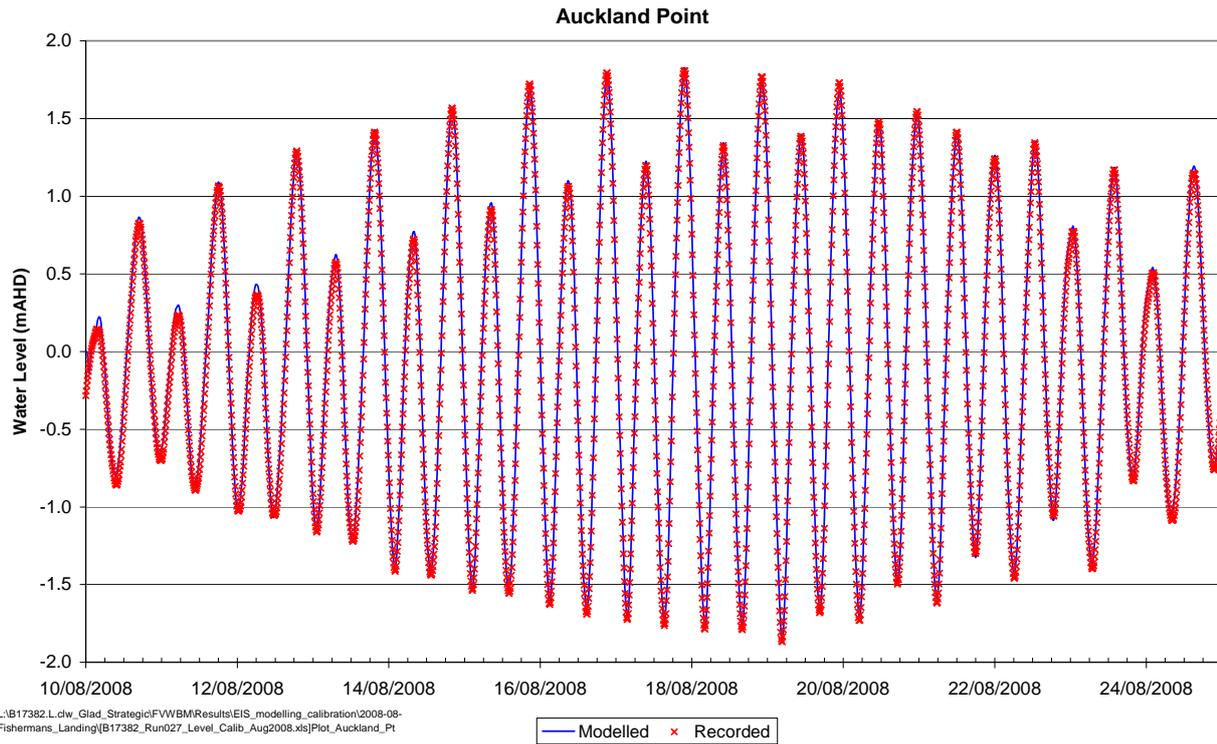
Figure 2-37 Water Level Validation – Auckland Point, August 2008
