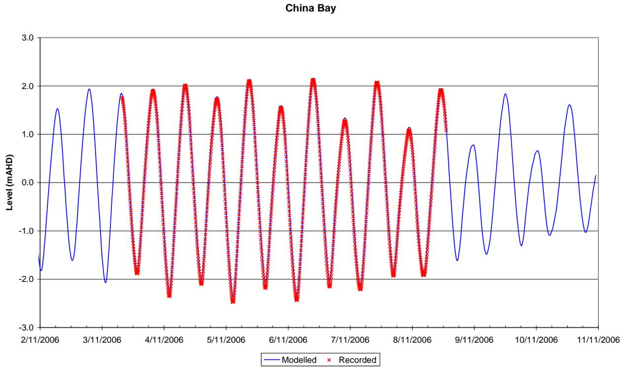
**Figure 2-22 Water Level Calibration – China Bay, November 2006**
