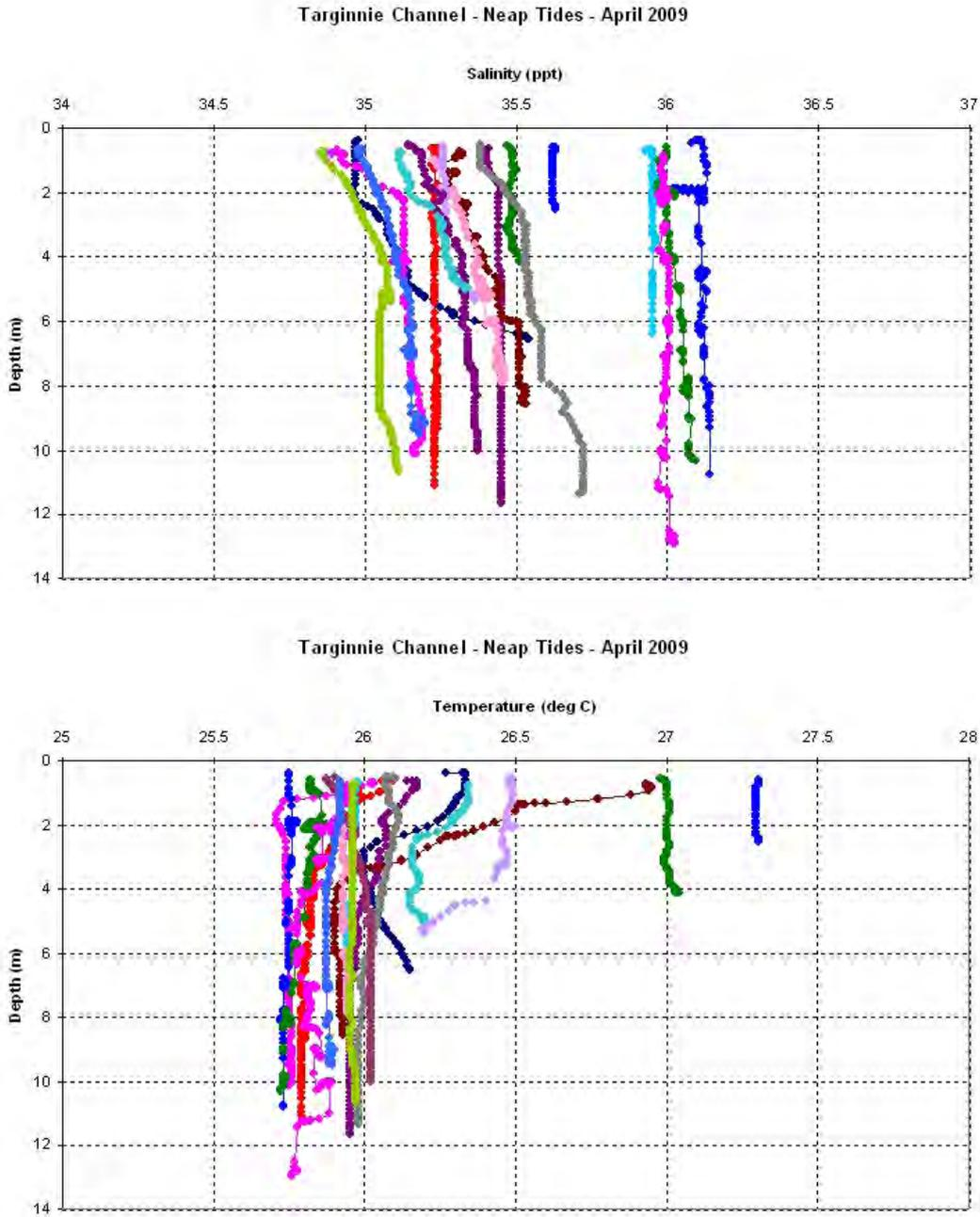
Figure A-2 Targinnie Channel Salinity and Temperature Profiles (19-20 April 2009)
