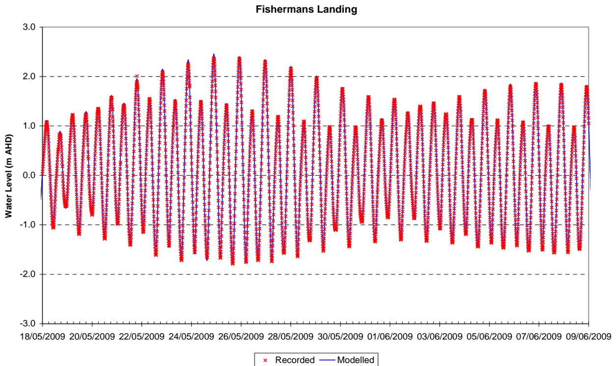
Figure 2-43 Water Level Validation – Fisherman's Landing, May 2009
