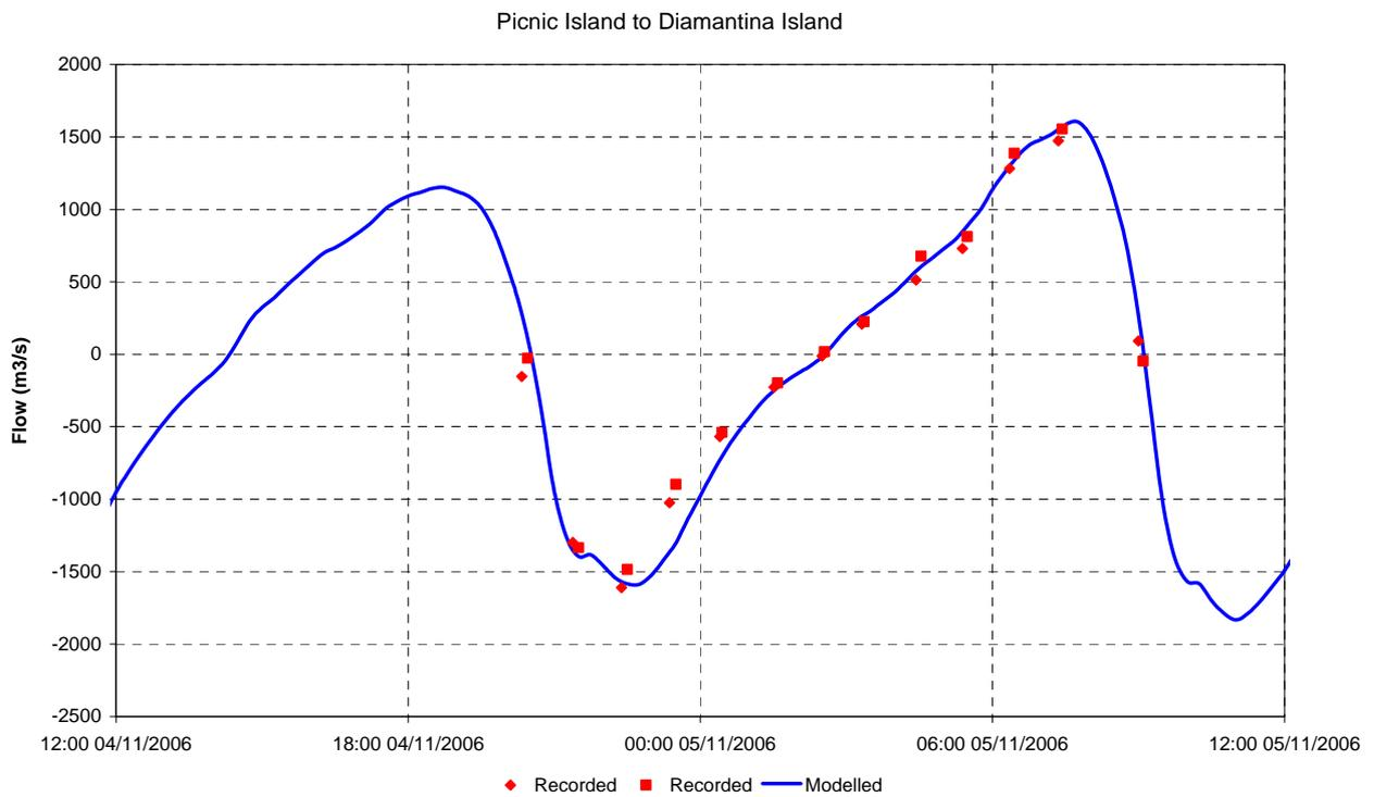
Figure 2-31 Flow Calibration – Picnic Island to Diamantina Island, November 2006
