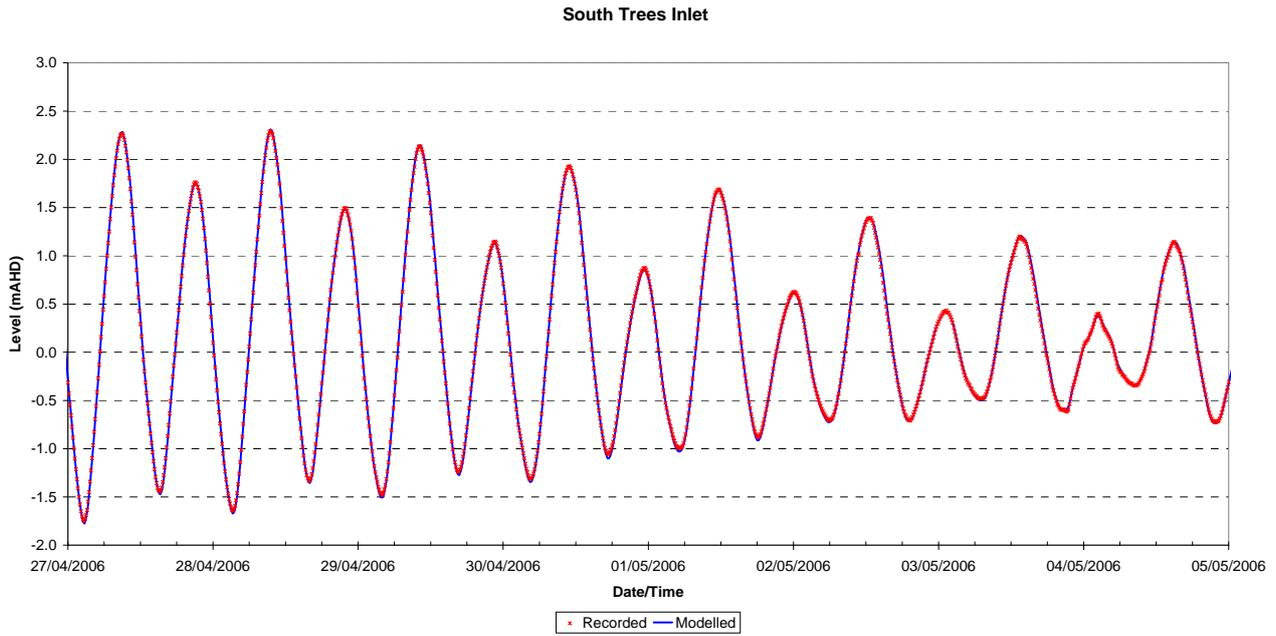
**Figure 2-7 Water Level Calibration – South Trees, April 2006**
