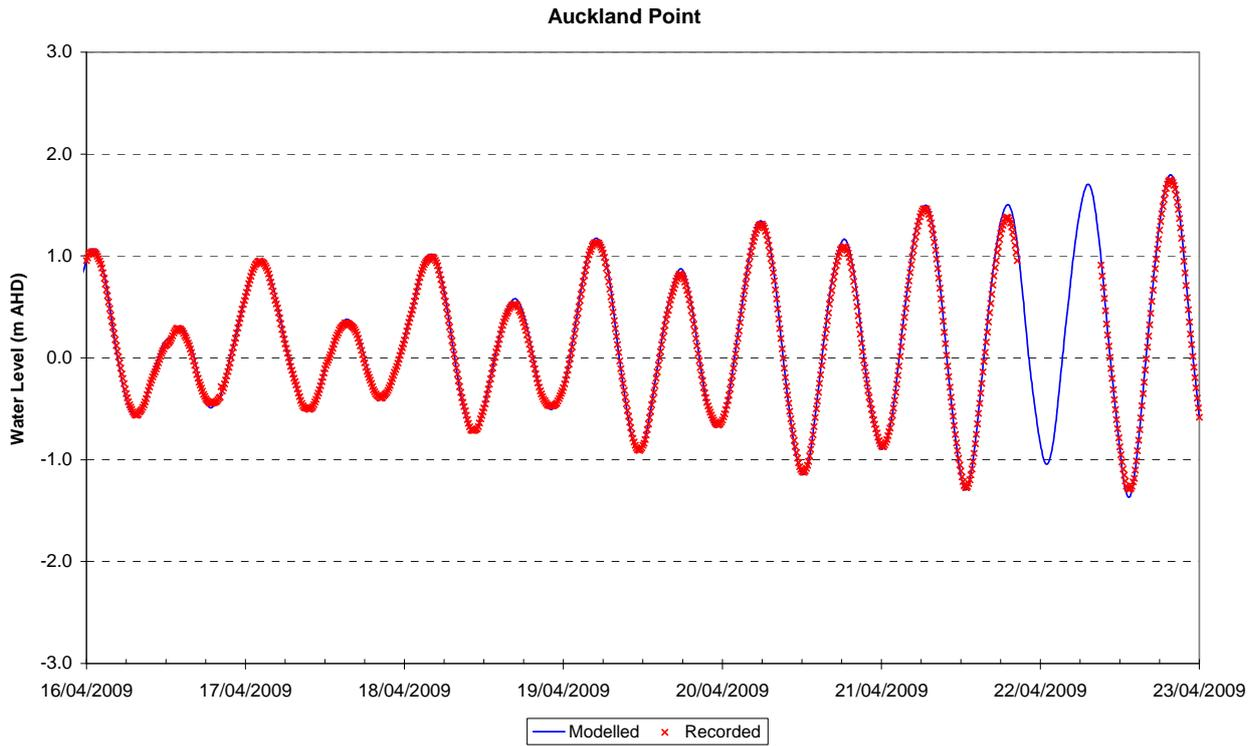
Figure 2-40 Water Level Validation – Auckland Point, April 2009 (Neap Tide)
