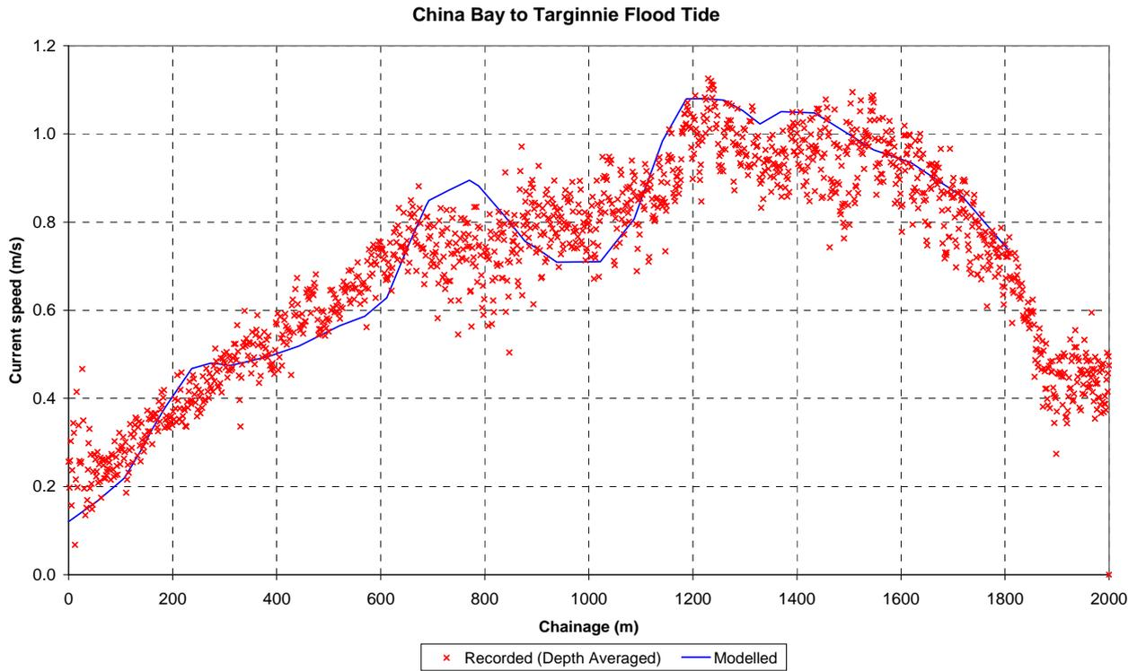
Figure D-3 Current Speed – China Bay to Targinnie, November 2006: Flood Tide
