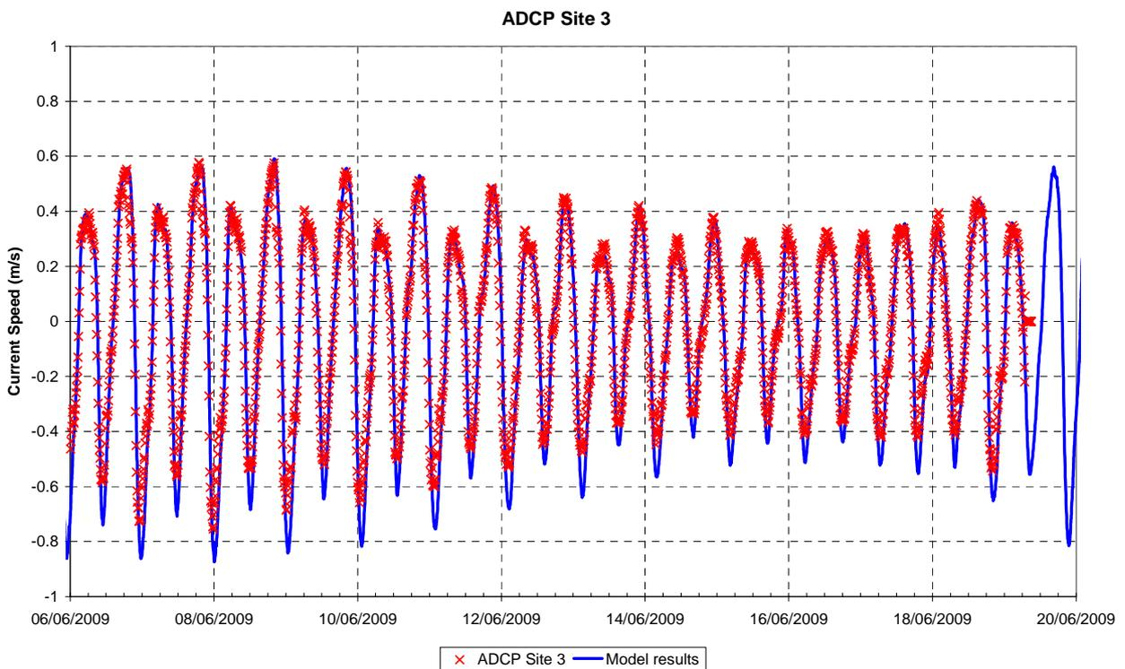
**Figure 2-61 Current Speed – GHD ADCP Site 3, June 2009**
