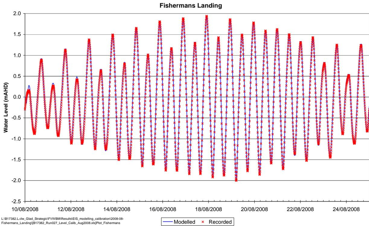
Figure 2-35 Water Level Validation – Fisherman’s Landing, August 2008
