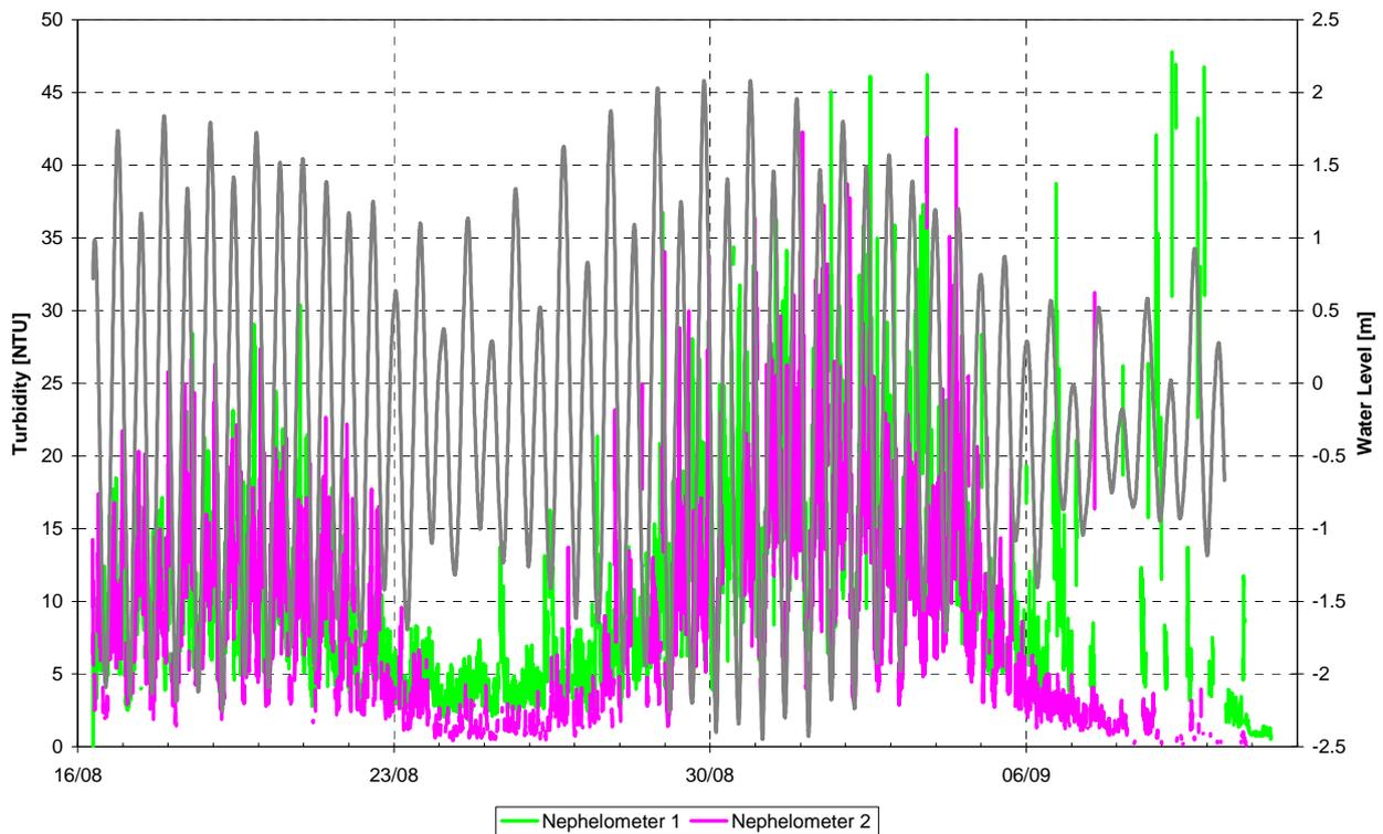
Figure 5-1 Turbidity time series collected by BMT WBM
