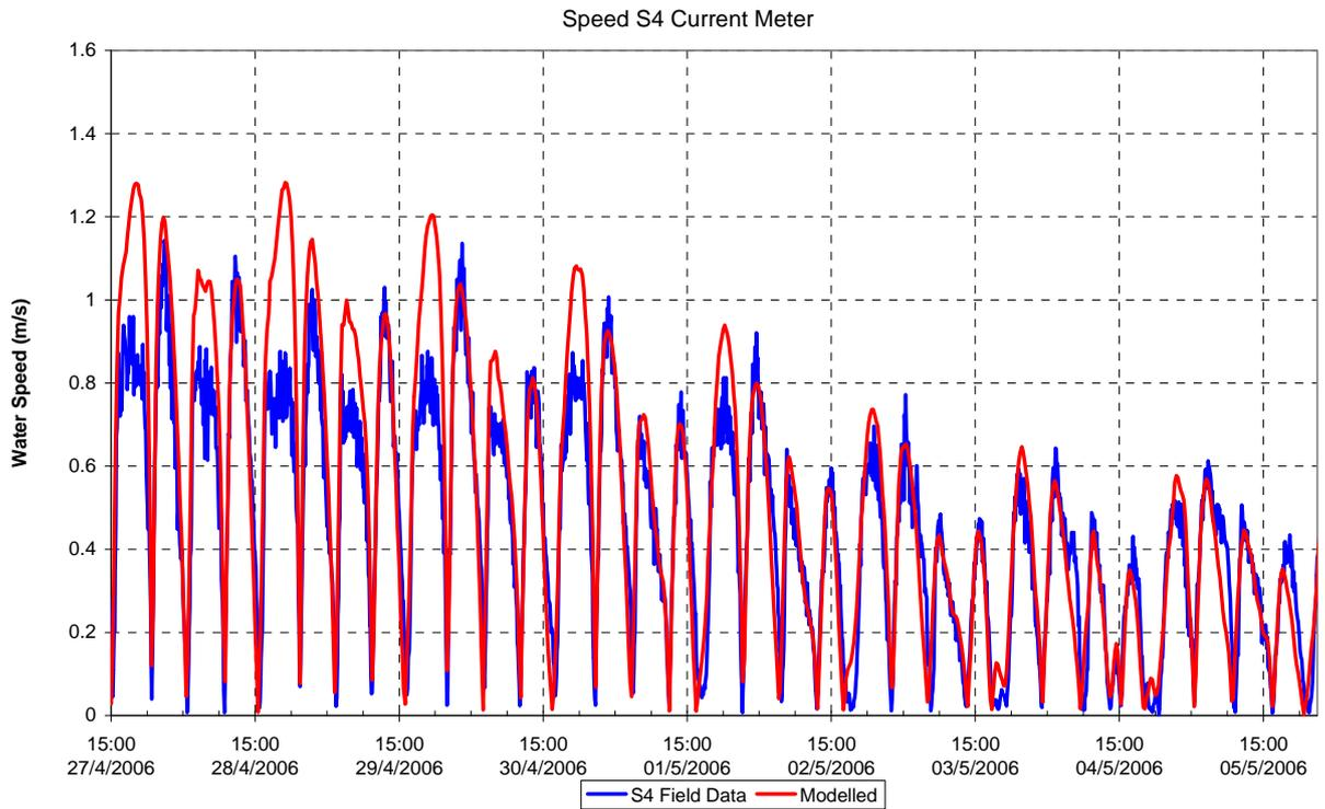
Figure 2-16 Current Speed – S4 Current Meter, April 2006
