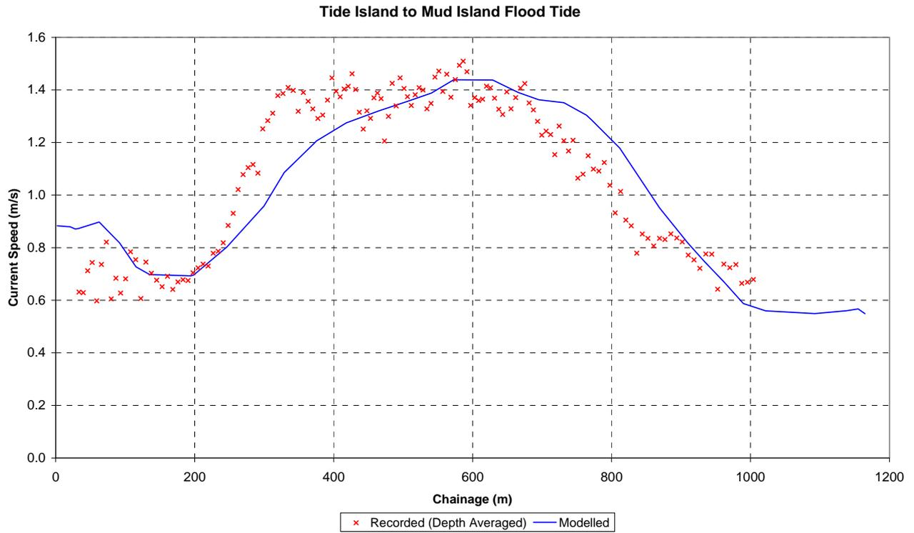
Figure C-3 Current Speed – Tide Island to Mud Island, April 2006: Flood Tide
