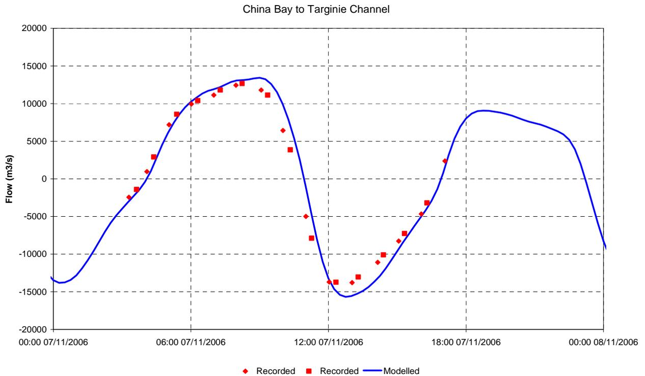
**Figure 2-27 Flow Calibration – China Bay to Targinie Channel, November 2006**
