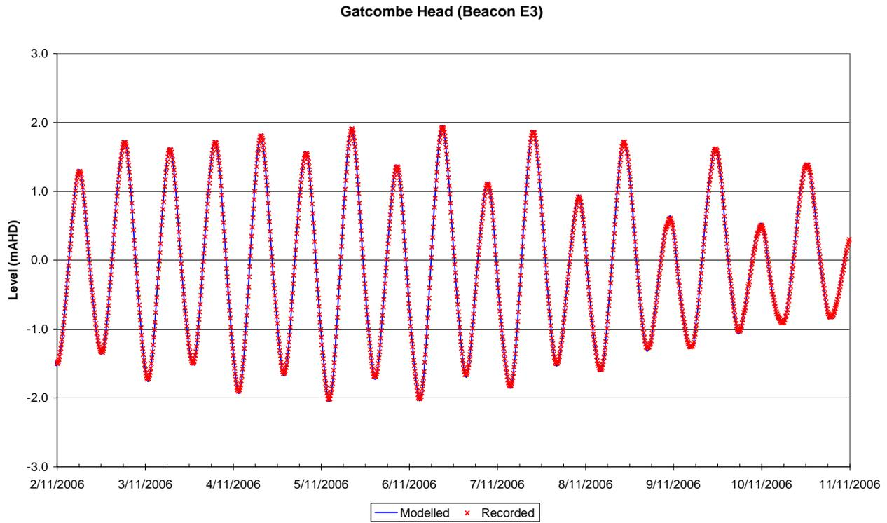
**Figure 2-24 Water Level calibration – Gatcombe Head, November 2006**
