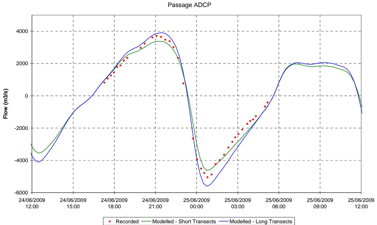
Figure 2-54 Flow Validation – “Curtis” Channel, June 2009
