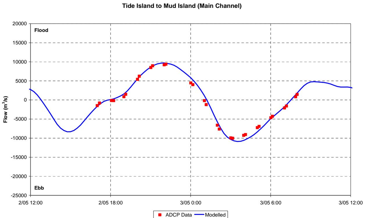
**Figure 2-14 Flow Calibration – Tide Island to Mud Island, May 2006 (Neap Tide)**
