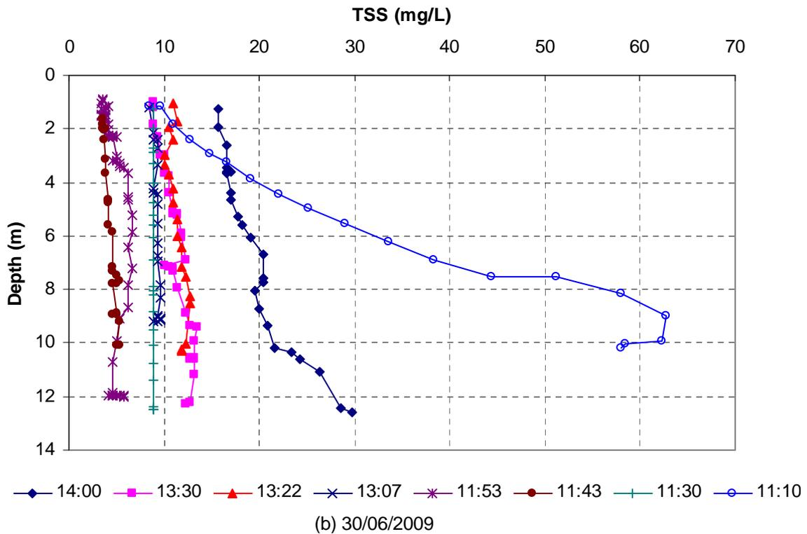
**Figure G-1 Profiles of TSS Derived from Turbidity Measurements:**
