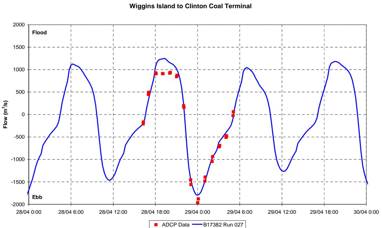
Figure 2-12 Flow Calibration – Wiggins Island to RG Tanna Coal Terminal, April 2006
