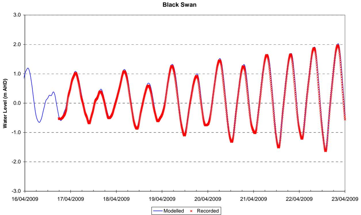
Figure 2-42 Water Level Validation – Black Swan Inlet, April 2009 (Neap Tide)
