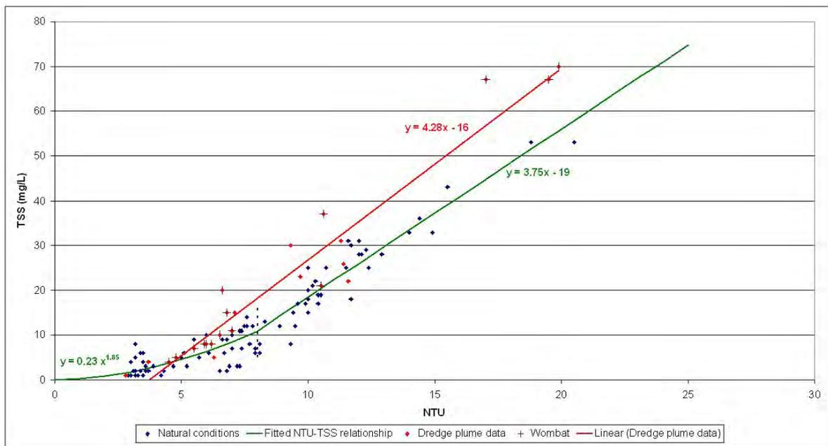
**Figure 5-3 NTU-TSS Relationship Derived for Both Natural and Dredge Plume Sampling**
