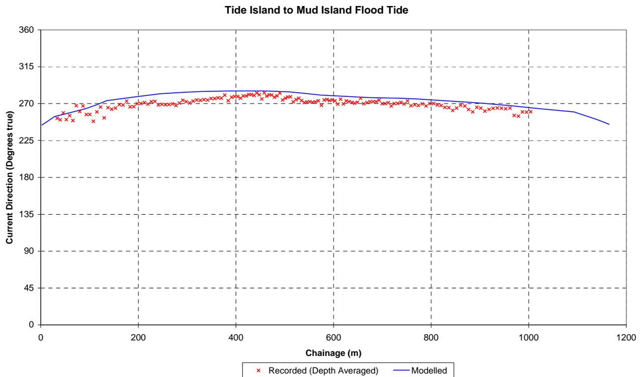
Figure C-4 Current Direction – Tide Island to Mud Island, April 2006: Flood Tide
