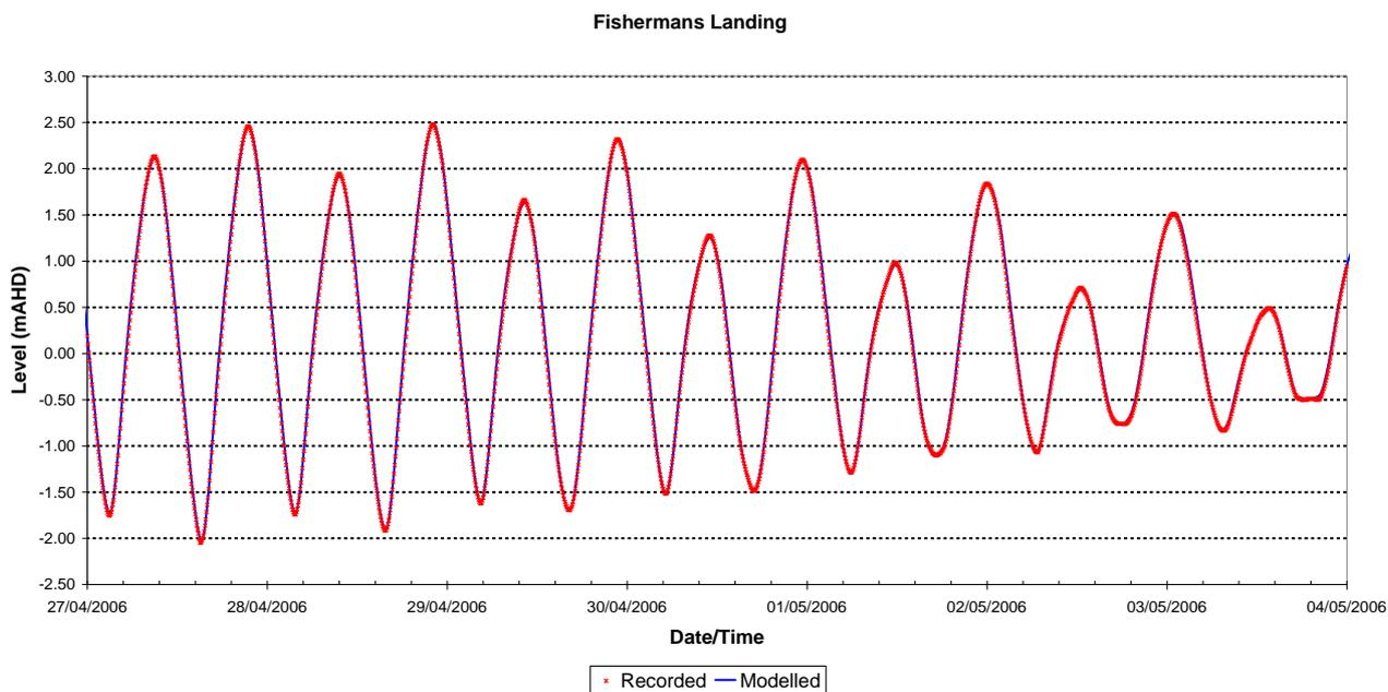
Figure 2-5 Water Level Calibration - Fisherman's Landing, April 2006
