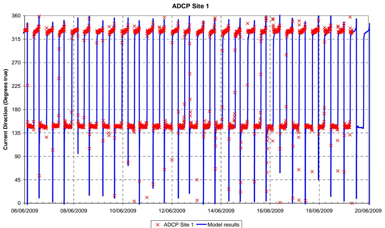
**Figure 2-63 Current Direction – GHD ADCP Site 1, June 2009**
