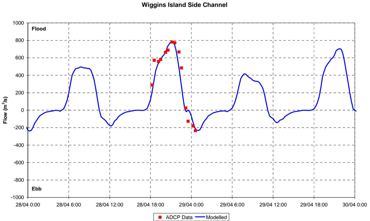
Figure 2-11 Flow Calibration – Wiggins Island Side Channel, April 2006
