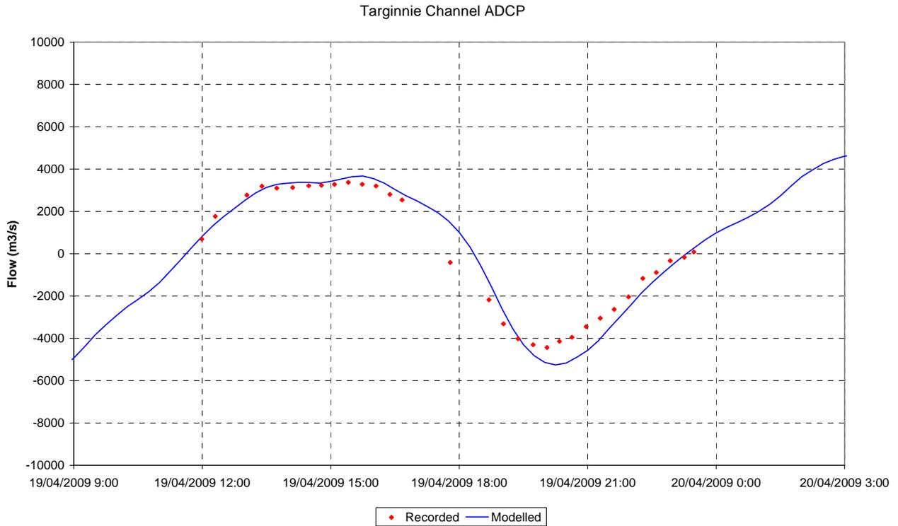
**Figure 2-52 Flow Validation – Targinnie Channel, April 2009 (Neap Tide)**
