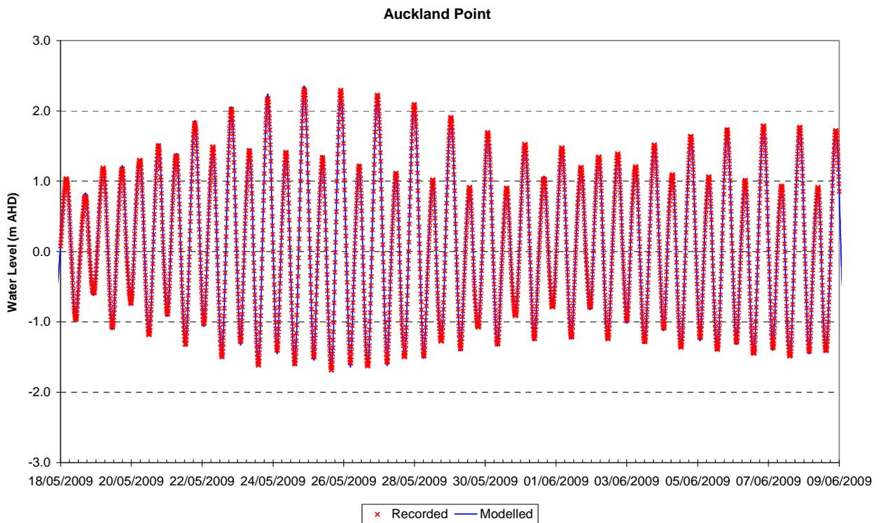
Figure 2-45 Water Level Validation – Auckland Point, May 2009
