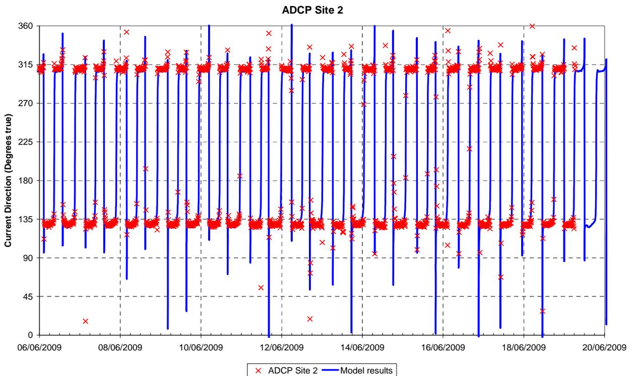
**Figure 2-65 Current Direction – GHD ADCP Site 2, June 2009**
