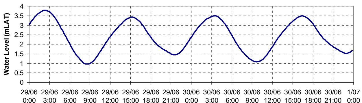
**Figure 5-2 Water level at Fisherman’s Landing (MSQ)**
