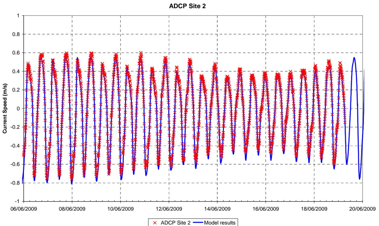
**Figure 2-59 Current Speed – GHD ADCP Site 2, June 2009**
