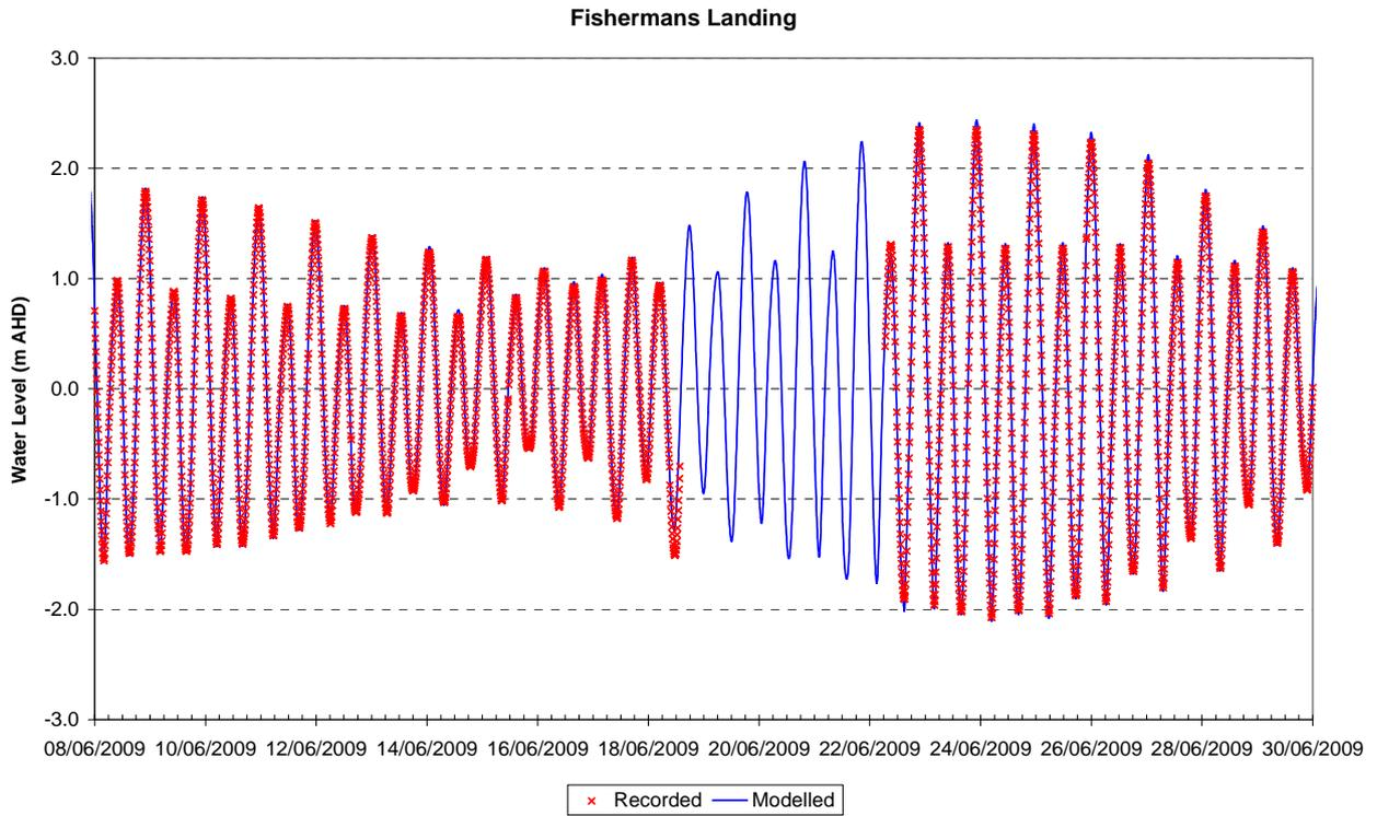
Figure 2-44 Water Level Validation – Fisherman's Landing, June 2009
