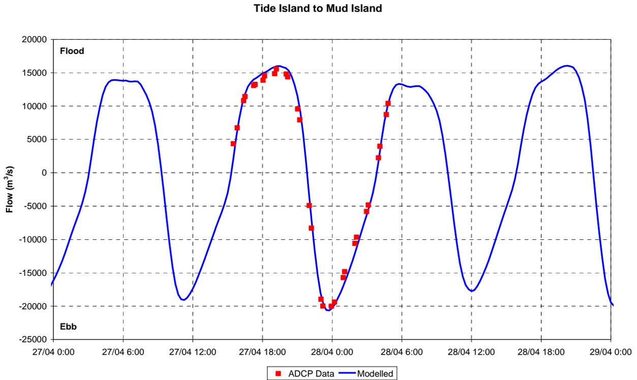
Figure 2-9 Flow Calibration – Tide island to Mud Island, April 2006
