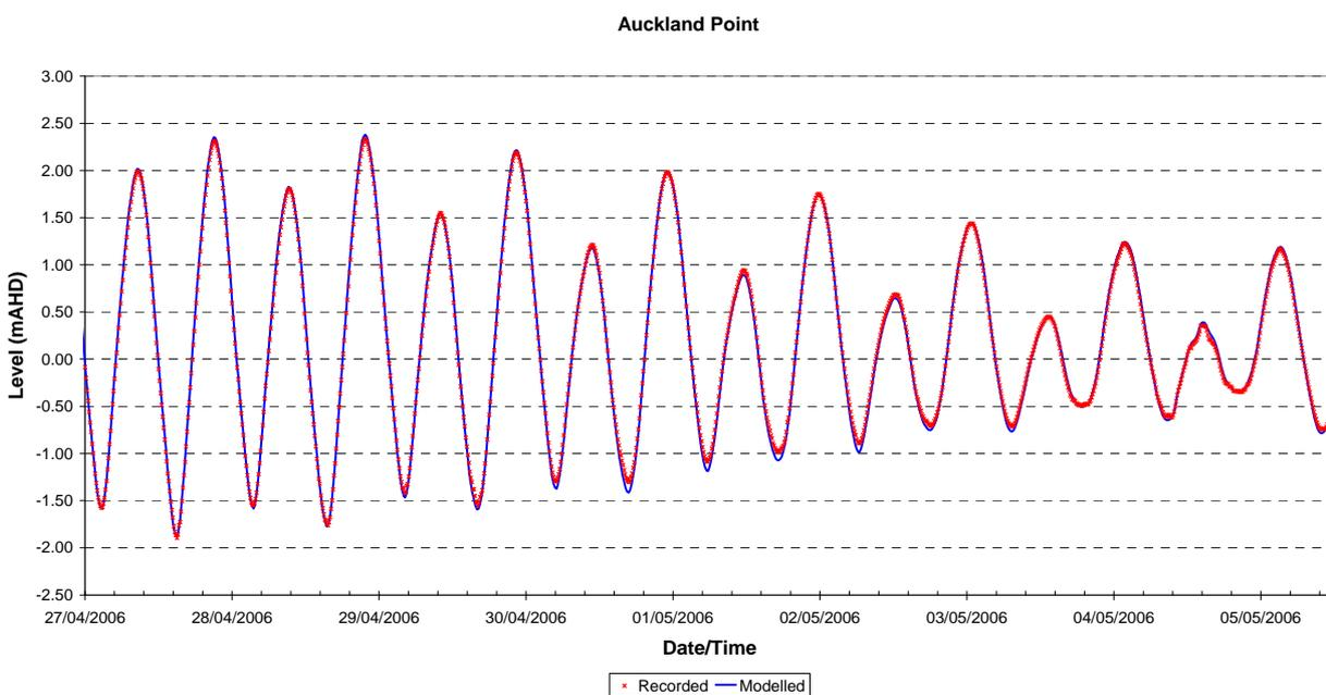
Figure 2-6 Water Level Calibration – Auckland Point, April 2006
