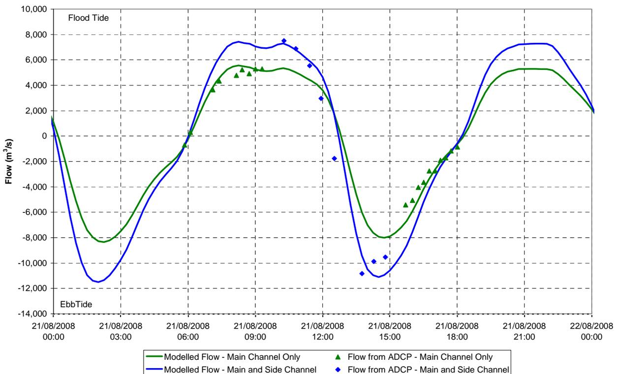
Figure 2-38 Flow Validation – Fisherman’s Landing, August 2008
