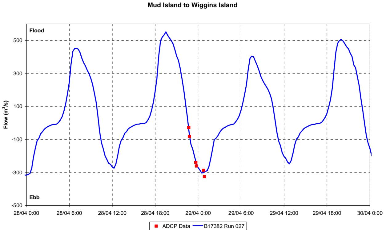
**Figure 2-13 Flow Calibration – Mud Island to Wiggins Island, April 2006**
