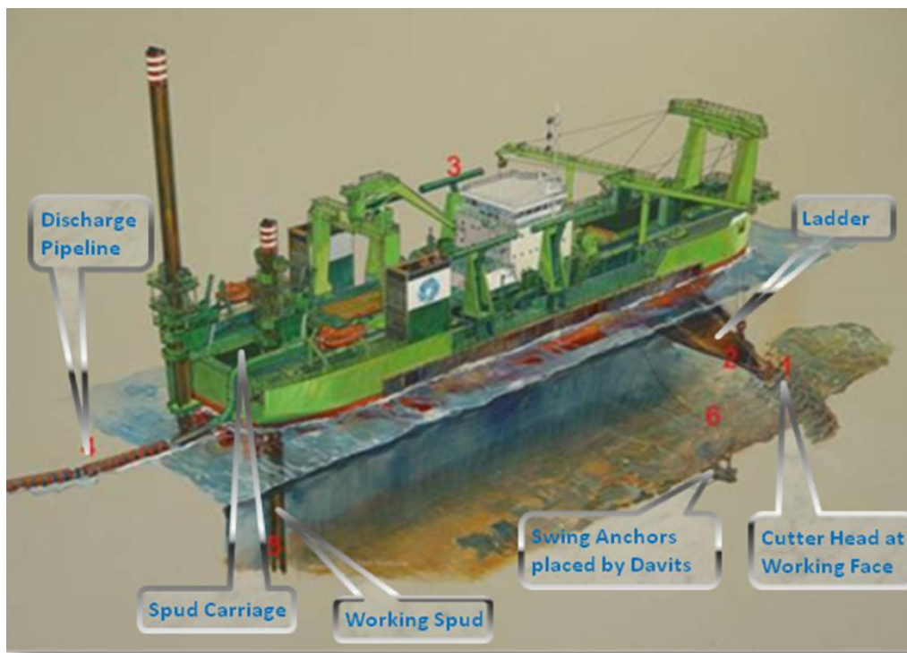
Figure 2-12 Key Operational Components of a Cutter Suction Dredger
