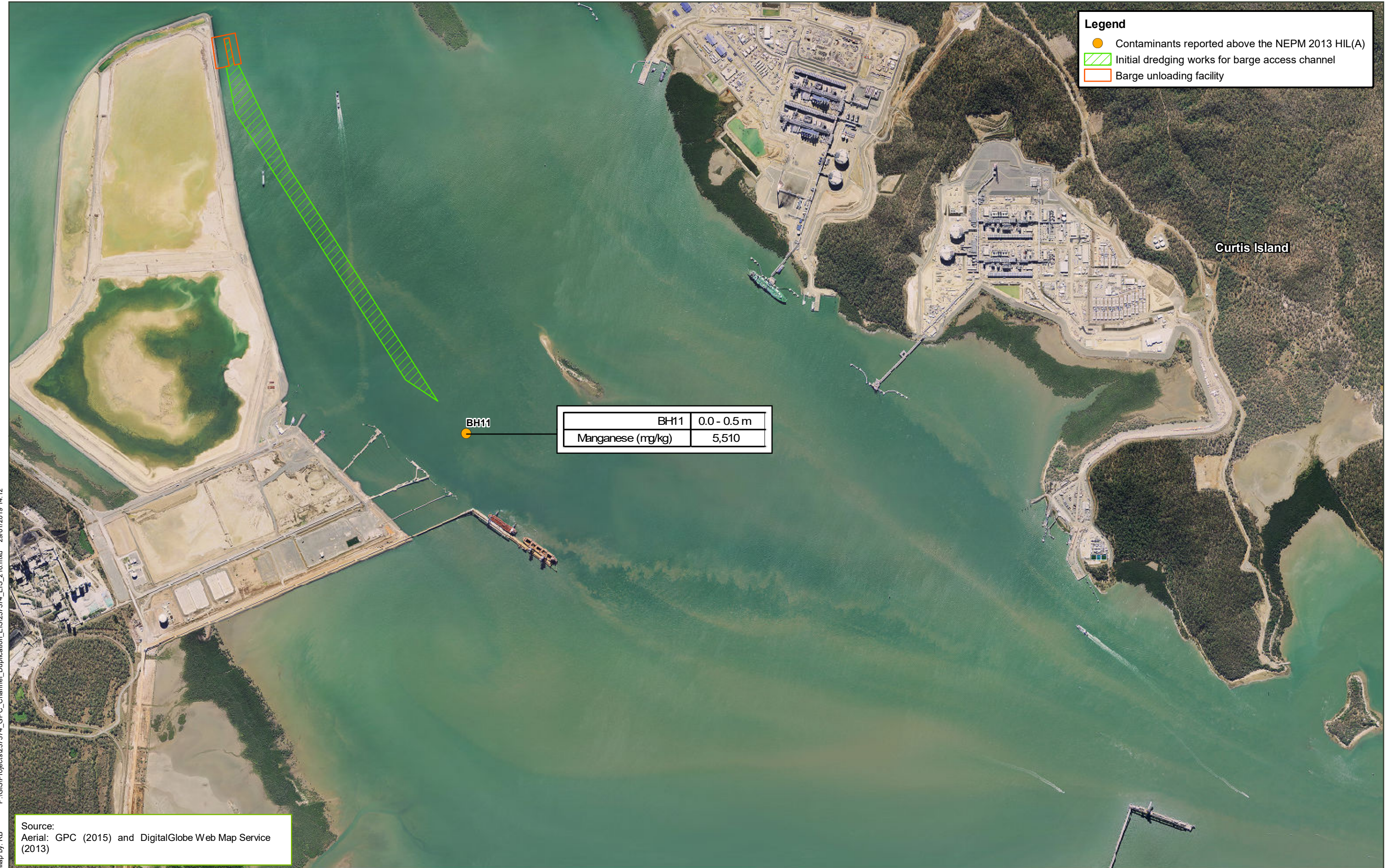
Figure 6.6: Contaminants reported above the NEPM 2013 HIL(A) within the barge access channel
