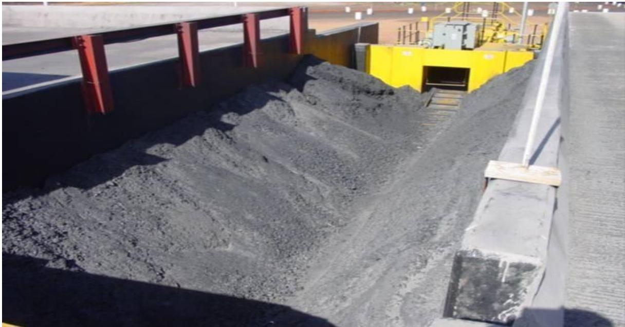
**Photograph 3-1 Example Reclaim Bunker**
