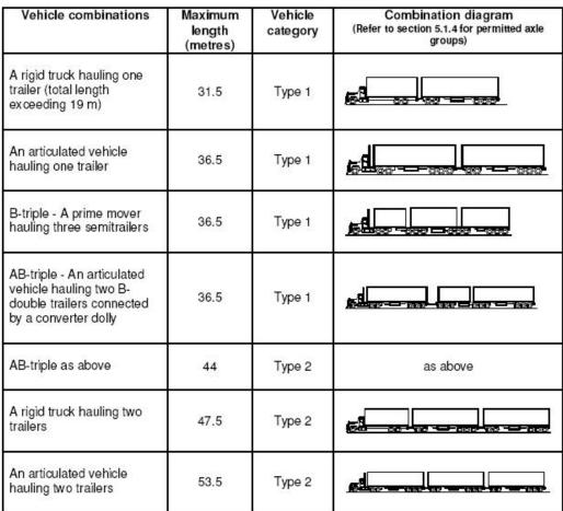
Figure 1: Typical Vehicle Combinations
