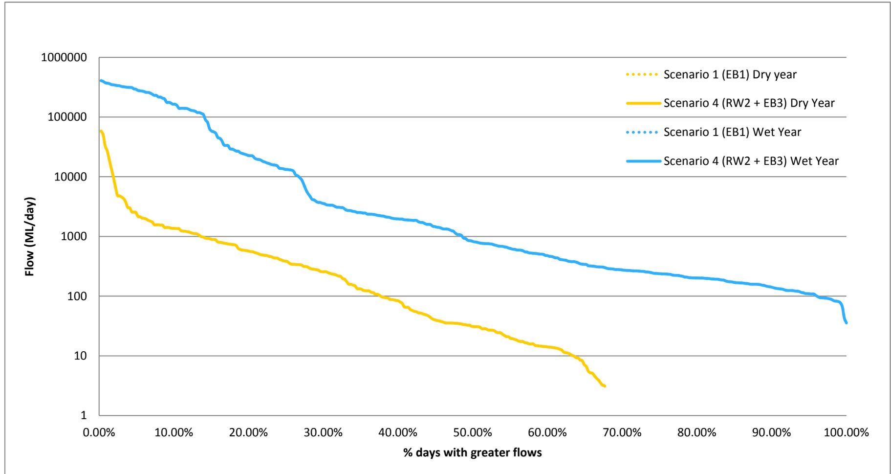
At data location IQQM5 (Riverslea; Node 003) flow data represents inflows to the system. As Rookwood Weir does not impact on inflows it is expected that pre- and post-project flows are the same as is reflected on the flow duration curves above.
