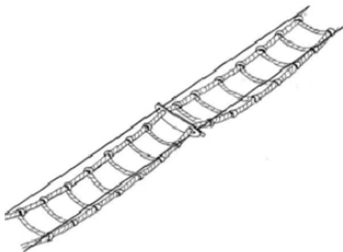
**Figure 2.4** Rope ladder style canopy bridge overpass (from DTMR Design Manual Volume 2 (2010)
