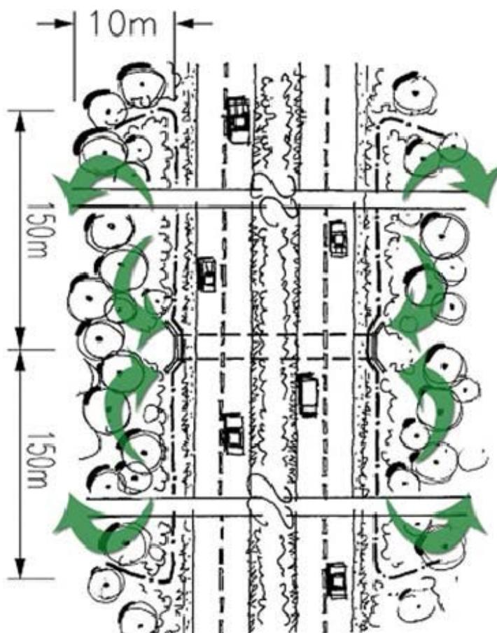
Figure 2.2 Optimal design of fauna exclusion fencing on either side of a crossing structure with incorporated returns at both ends (from DTMR Design Manual Volume 2 (2010))
