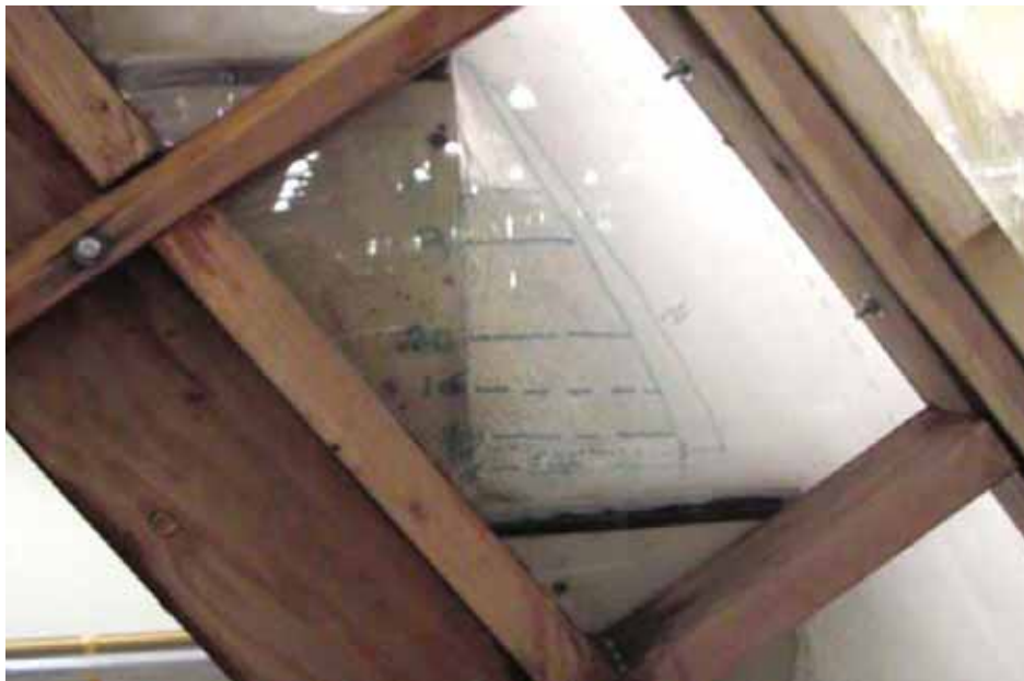
Plate 10.B.21: Prototype (Section View) Flow = 3.28 m 3 /s/m
