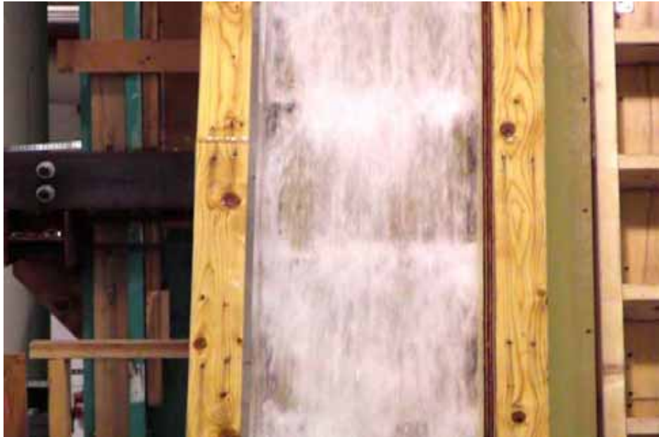
Plate 10B.6: Prototype (Elevation View) Flow = 0.2 \text{ m}^3/\text{s}/\text{m}
