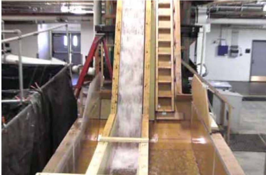
Plate 10B.10: Prototype (Elevation View) Flow = 0.45 \text{ m}^3/\text{s}/\text{m}
