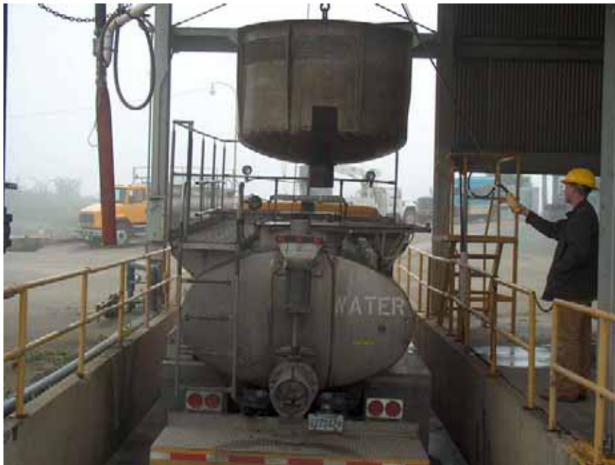
Plate 10A:1: View of fish in a transfer hopper being loaded into a fish truck at the Tracy Fish Collection Facility
