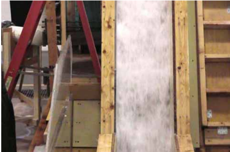
Plate 10B.12: Prototype (Elevation View) Flow = 0.61 m 3 /s/m
