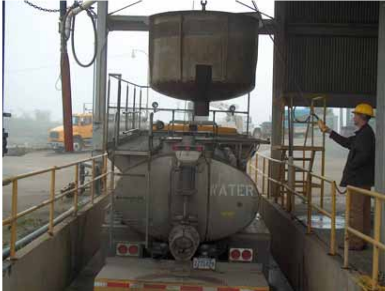
Plate 10:7: Example of a Fish Transfer Hopper
