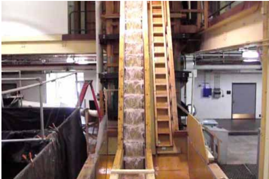
Plate 10B.4: Prototype (Elevation View) Flow = 0.1 \text{ m}^3/\text{s}/\text{m}
