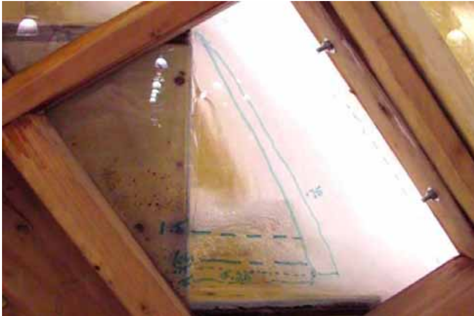
Plate 10B.18: Prototype (Section View) Flow = 1.22 m 3 /s/m
