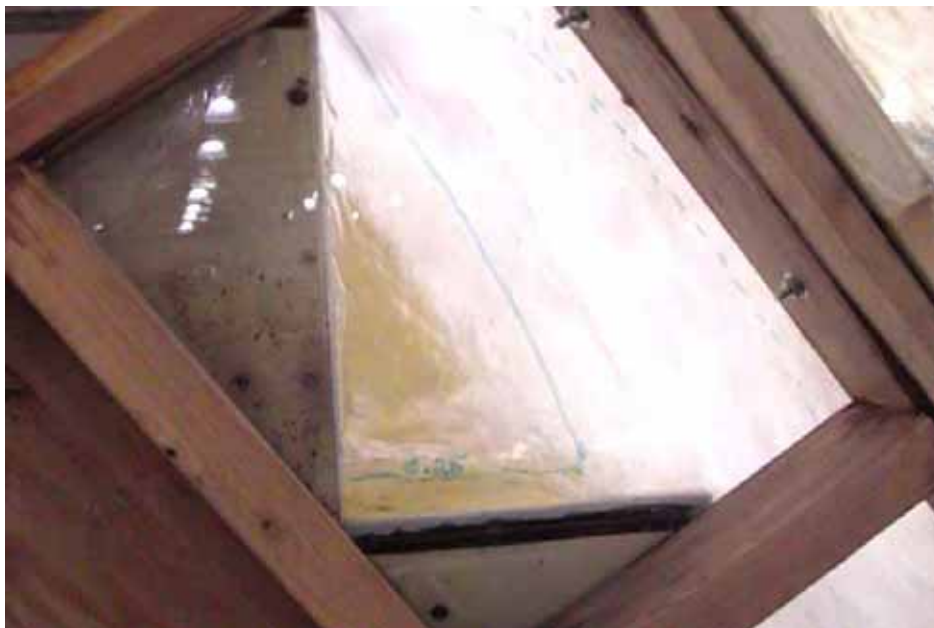
Plate 10B.11: Prototype (Section View) Flow = 0.45 \text{ m}^3/\text{s}/\text{m}
