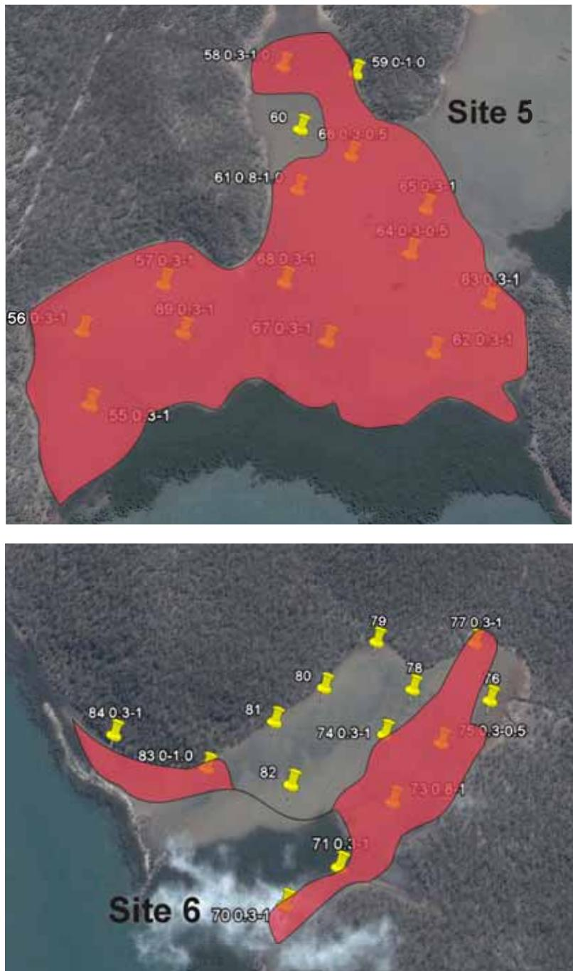
Figure D-1 Distribution of low but actionable levels of AASS (>0.03%S or 18 mol H<sup>+</sup>/t) within the top 1 metre.
