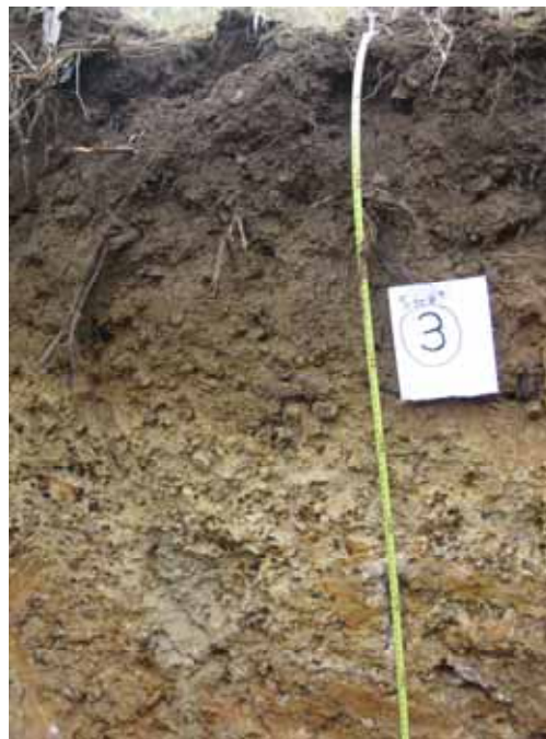
Plate A-2 Site #3, Group 4 soil - shallow uniform gravelly loam in terrain unit Cw4/4-7
