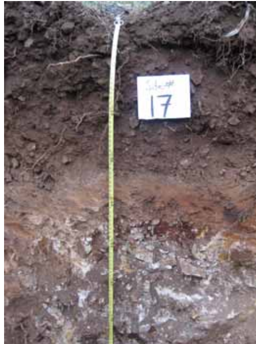
Plate A-9 Site #17, Group 7 soil (Type 7.1) – shallow gradational gravelly clay soil in terrain unit Cw7/4-7
