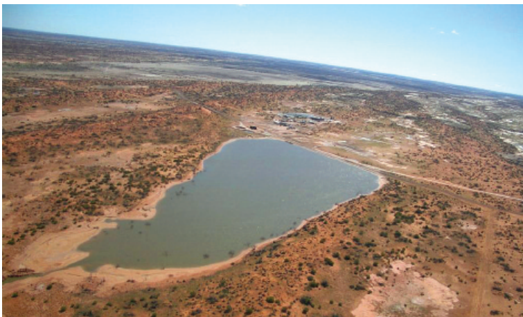
One of the freeform evaporation ponds at Limestone Creek satellite in the Cooper Basin.
