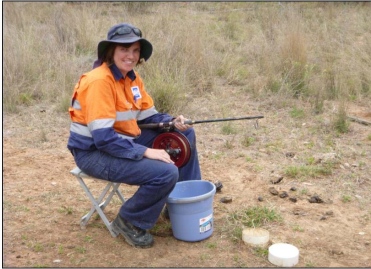
Plate 2-1: Stygofauna sampling of a Waratah GCP groundwater bore in September 2012 (Photo: GHD Water Sciences).
