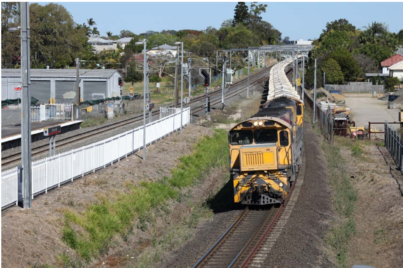
Coal train in Queensland demonstrating use of covers similar to those proposed for use by Waratah Coal
