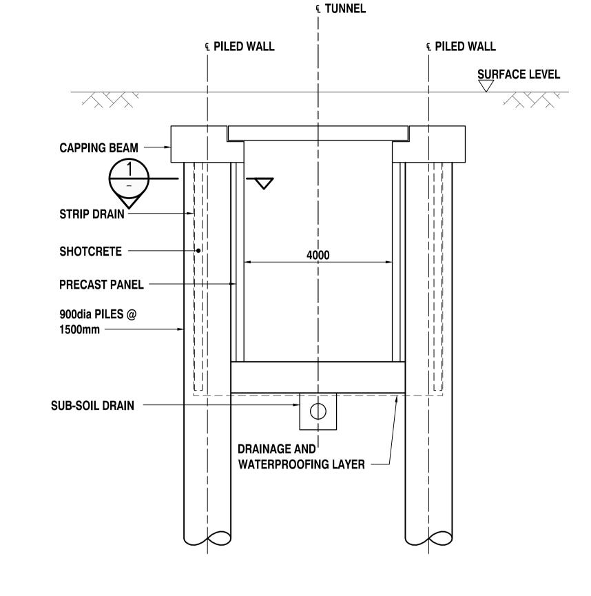
**CANTILEVERED PILE** TROUGH STRUCTURE TYPICAL SECTION
