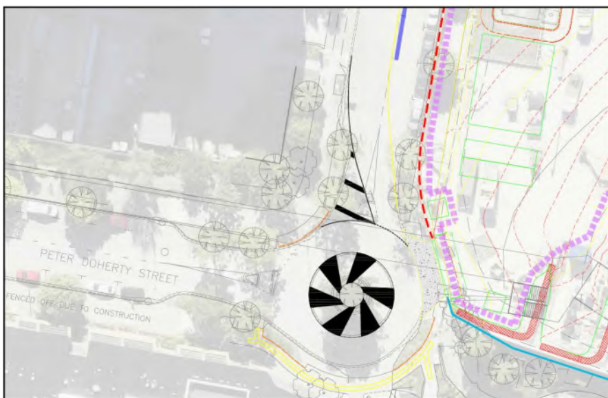
Figure 3: Joe Baker/Peter Doherty guidance scheme – island/roundabout modifications
