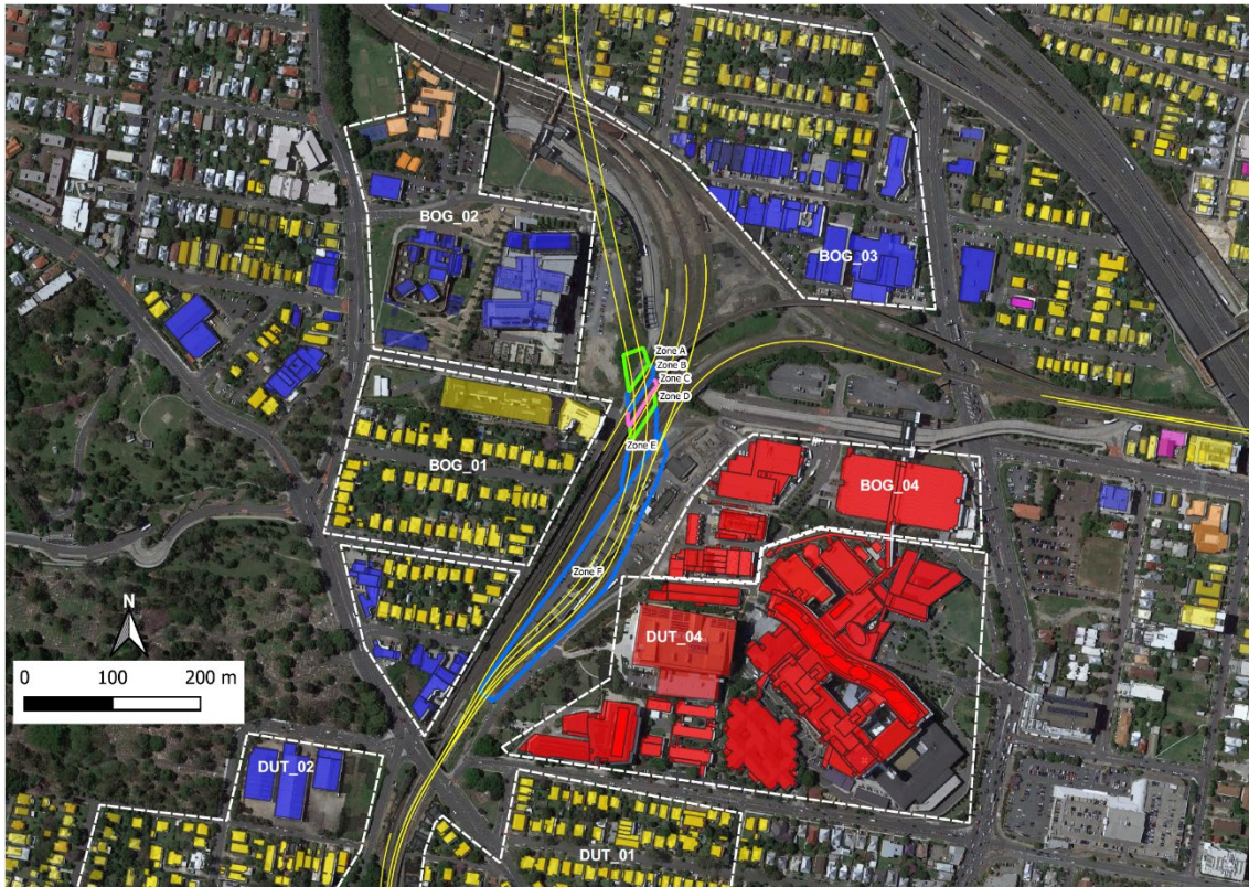
Figure 4.2 Noise Catchment Areas and Worksite Zones within the Southern Portal Area worksite zones
