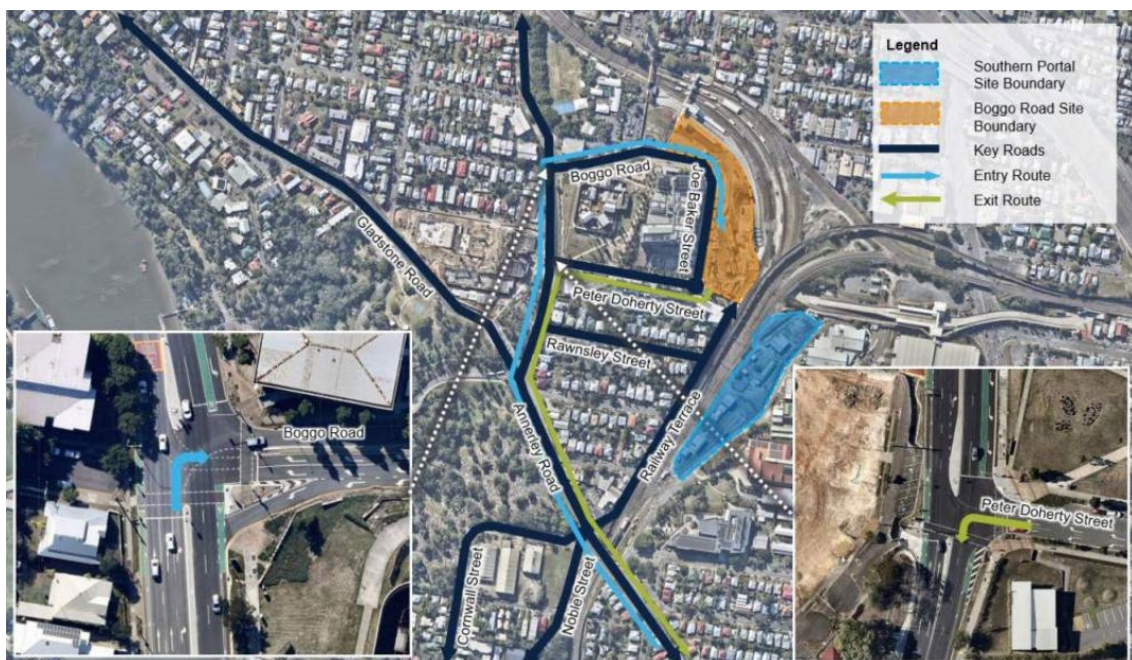
Figure 4.1 Existing heavy vehicle access route
