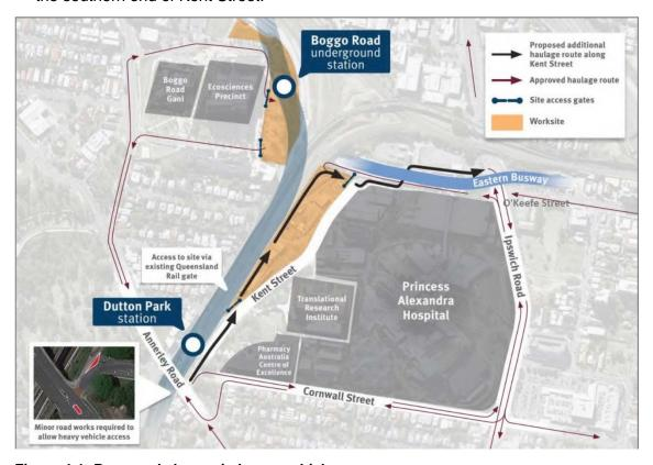
Figure 4-1: Proposed change in heavy vehicle access
