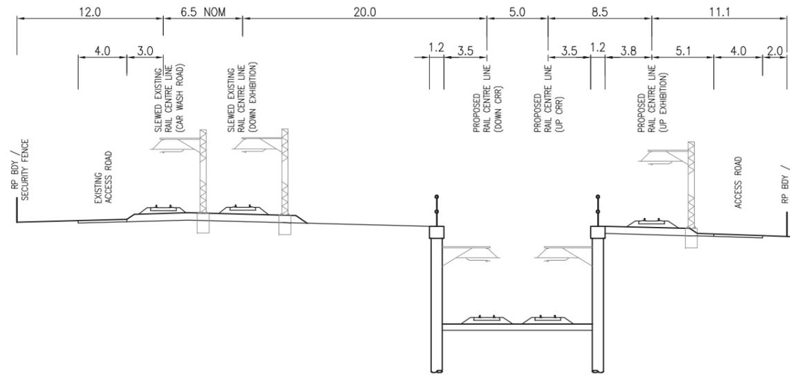
TYPICAL RAIL CROSS SECTION – NORTH TUNNEL PORTAL/DIVE STRUCTURE
