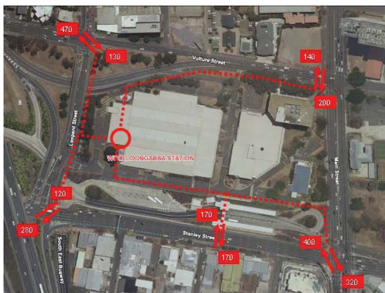
Figure 6-33 Forecast 2021 Gabba Station and busway passenger movements in the morning peak hour
