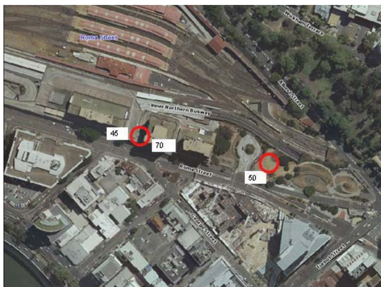
Figure 6-29 Forecast maximum accumulation of rail alighters on footways in 2021 AM peak 2 minutes
