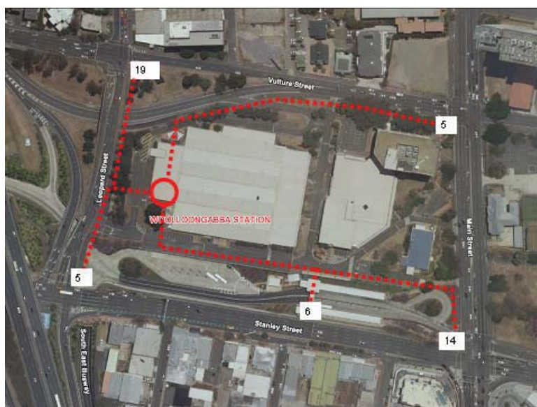
Figure 6-34 Forecast 2021 Gabba Station and busway passengers accumulating at pedestrian crossings over peak 2 minutes in the morning peak hour
