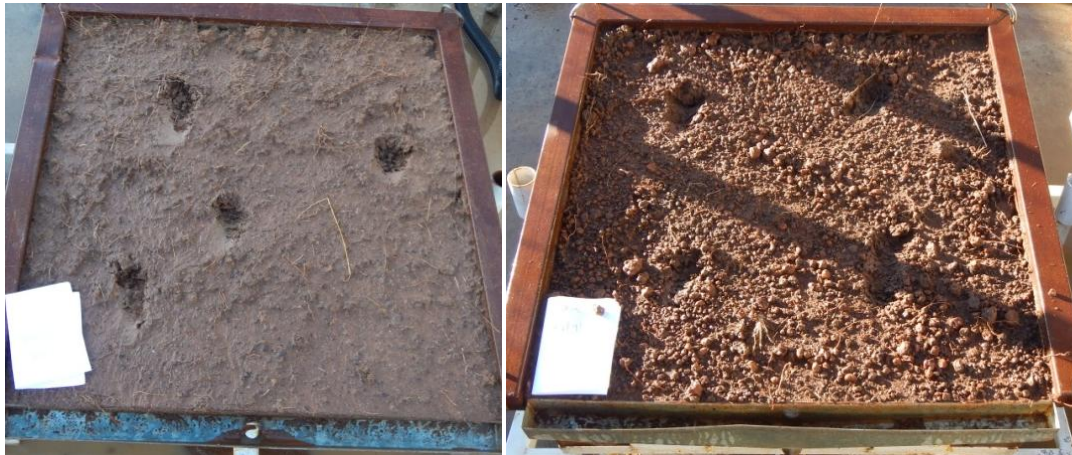
Figure 6: Rainfall simulator plots of Sample 1 (left) and Sample 2 (right) following application of simulated rain, showing indents where samples were taken post-rain for water content measurement.
