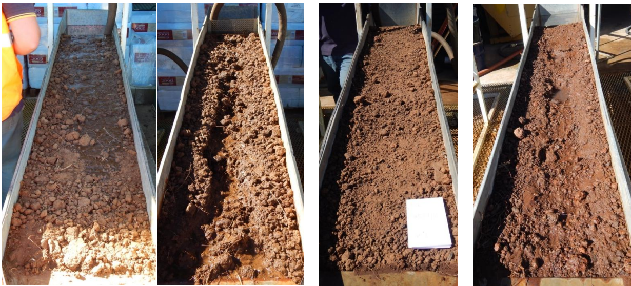
Figure 5: Flumes of (from left) cloddy Sample 1 on initial application of flow and after application of overland flows, and the gravelly Sample 2 prior to and after application of flows.
