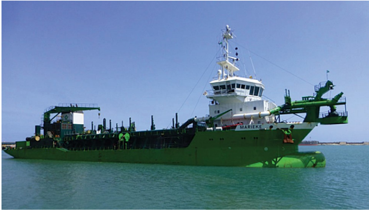
Photo C3-2 Example of a medium size TSHD.
