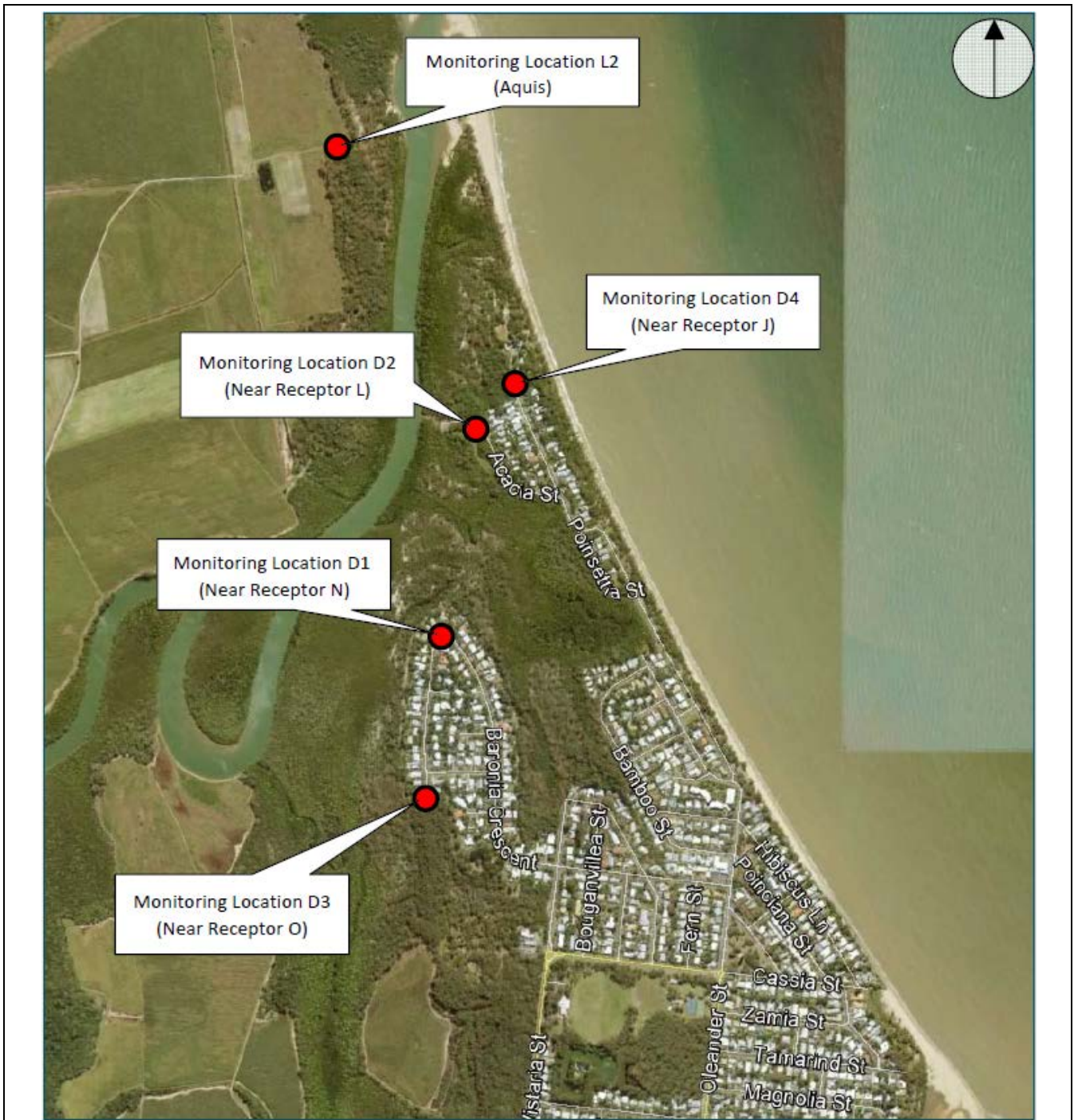
Figure B10-4 Northern Sands Project Area (delivery pipeline) key sensitive receptors and noise monitoring locations. Source: Appendix AU (Figure 5.2).
