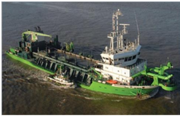
Photo A3-1 Example of TSHD (TSHD Marieke ).
