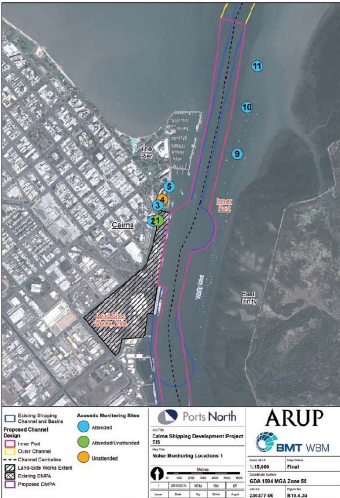
Figure 5.5 ARUP Noise Monitoring Locations - Wharf Street Area (Figure B.10.4.3a of Draft EIS)
