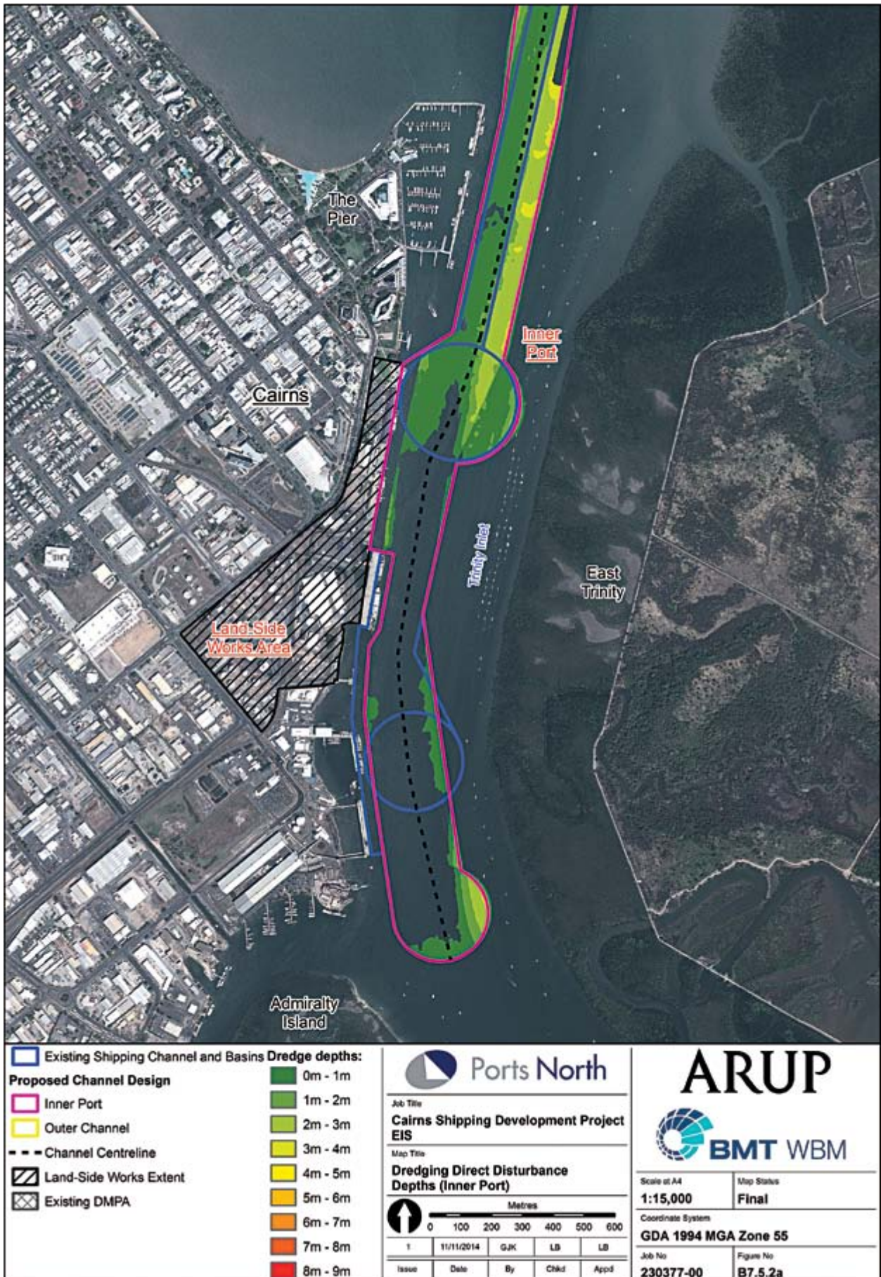
Figure B7.5.2a Capital Dredging Direct Disturbance Footprint for the Inner Port, Wharf Upgrade Works and Nearshore Sections of the Outer Channel
