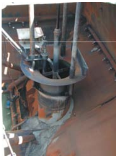
Figure B5.5.4.1a Overflow Funnel in a TSHD Hopper – Photo (top) and Schematic (bottom)
