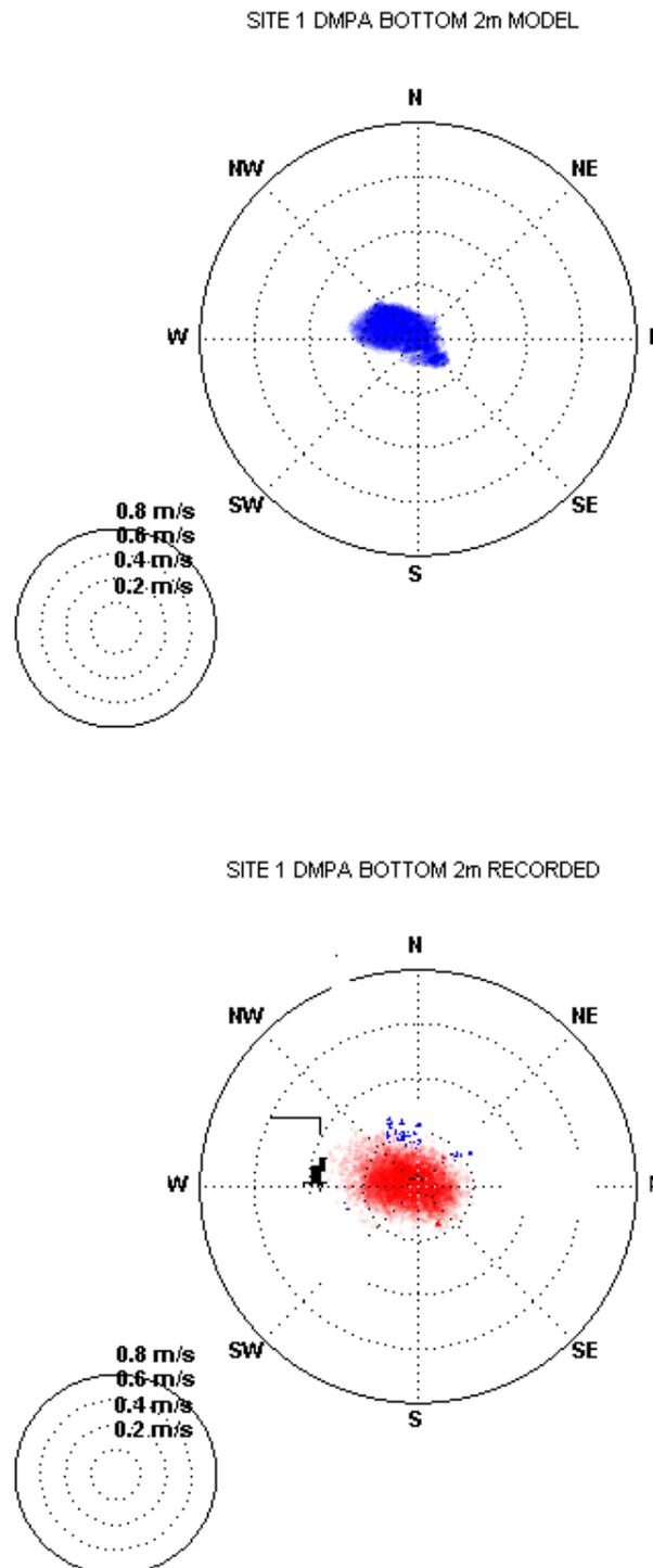
Figure D-2 Current Polar Plot Calibration – DMPA Bottom 2m of Water Column
