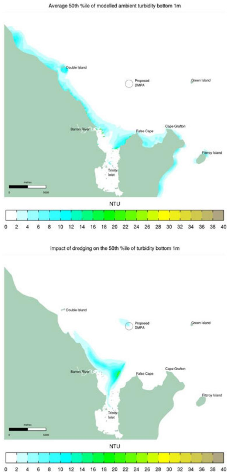
Figure 6-24 “Worst Case” Stiff Material Dredging 50<sup>th</sup> Percentile Bottom 1m Turbidity: Average Ambient Turbidity (top), Impact of Dredging (bottom)
