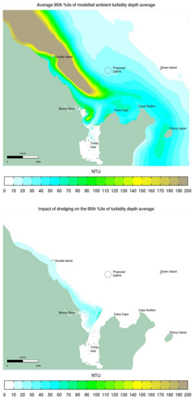
Figure 6-21 “Worst Case” Stiff Material Dredging 95<sup>th</sup> Percentile Depth Average Turbidity: Average Ambient Turbidity (top), Impact of Dredging (bottom)
