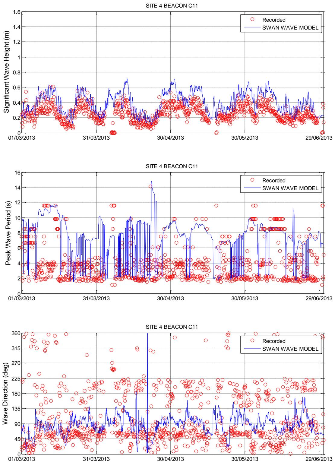
Figure 3-32 SWAN Wave Model Calibration – Site 4 Beacon C11
