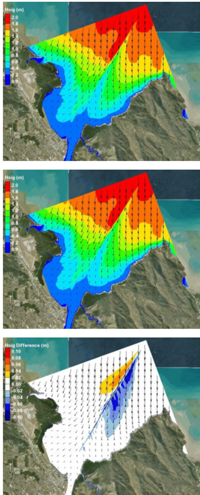
Figure 7-21 25m Grid Northerly Wave Case: Base case (top); Developed case (middle); Difference (bottom)
