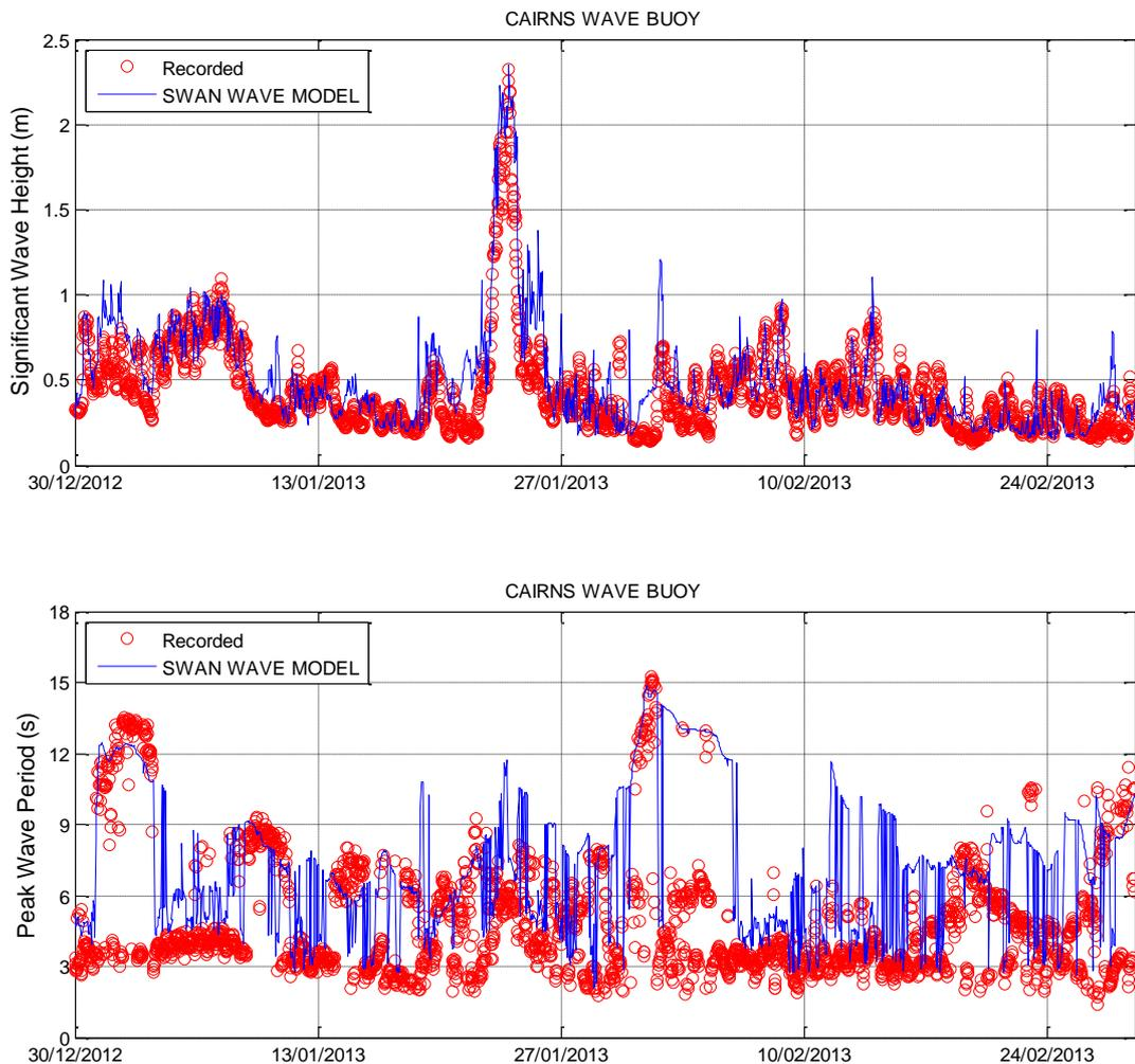
**Figure 3-28 SWAN Wave Model Calibration – Cairns Wave Buoy**
