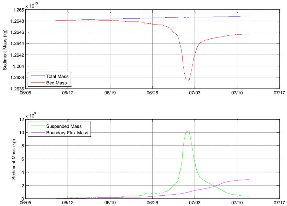
Figure 4. Sediment Mass Balance Checks - Worst Case Soft Material Dredging
