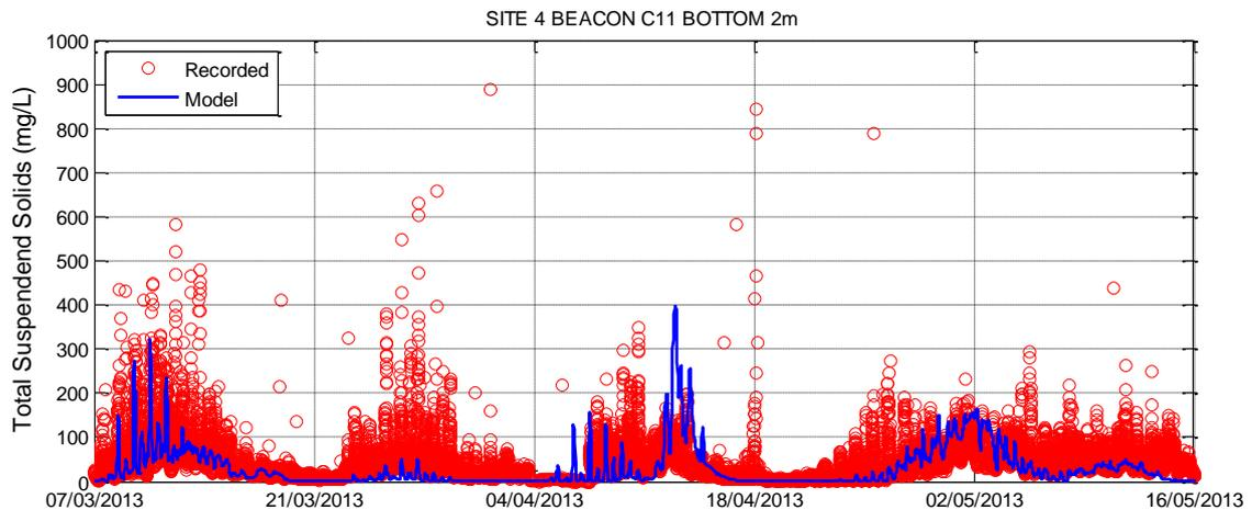
**Figure 3-39 Sediment Re-suspension Calibration – Beacon C11**
