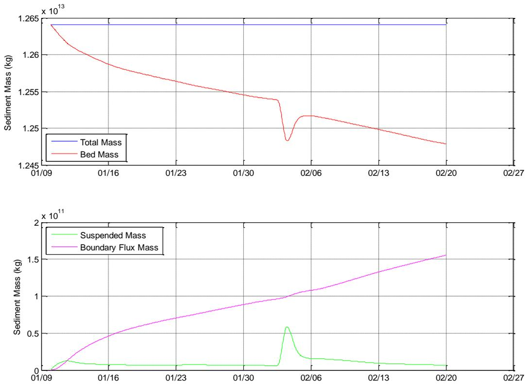
Figure 6. Sediment Mass Balance Checks - Worst Case DMPA Re-suspension
