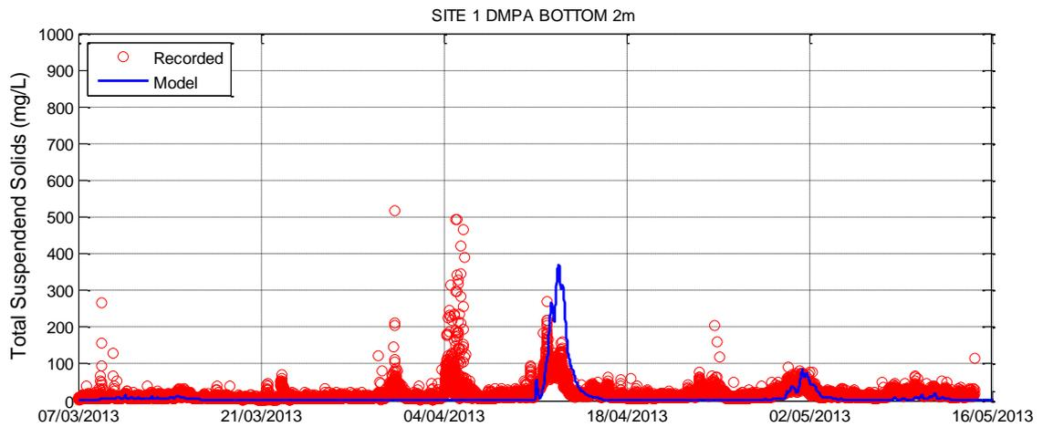
Figure 3-36 Sediment Re-suspension Calibration – DMPA
