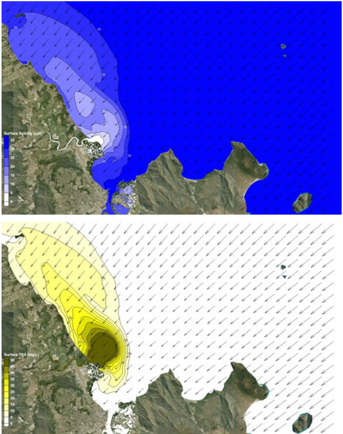
Figure 5-26 Barron River Flood Plume with North-Easterly Winds - Surface Salinity (top) and Surface TSS (bottom)
