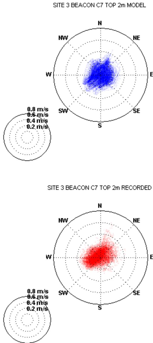
Figure G-4 Current Polar Plot Calibration – Site 3 Top 2m of Water Column
