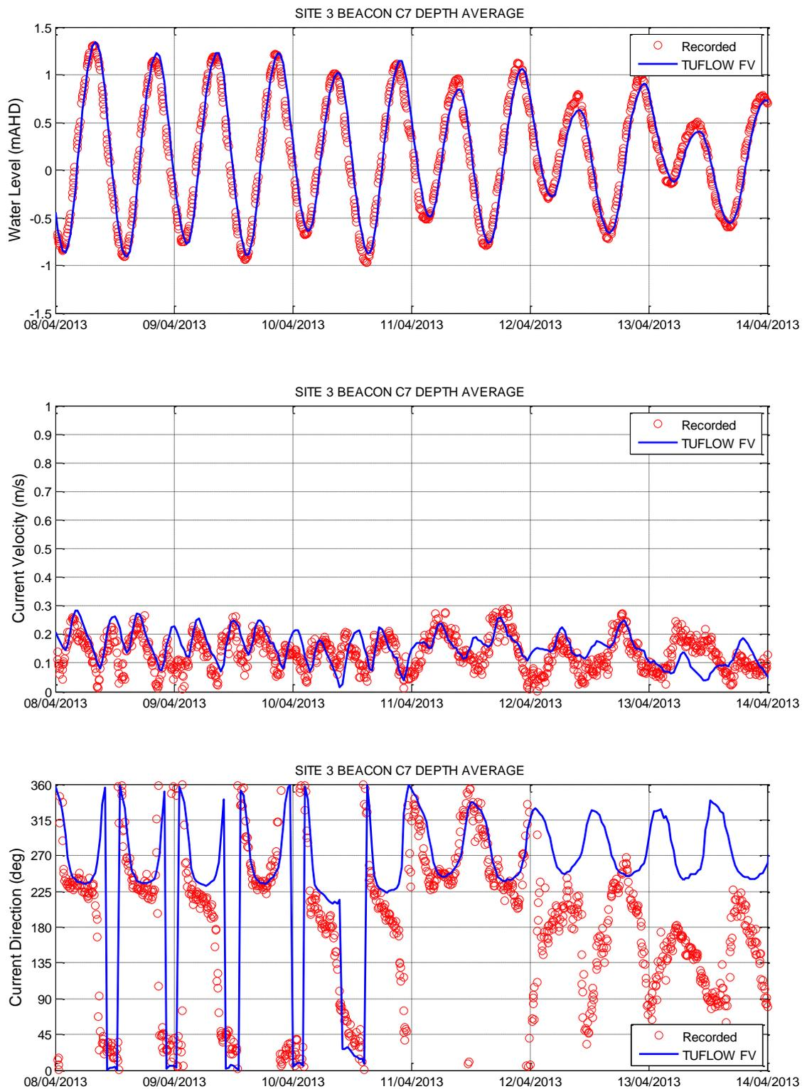
Figure 3-15 Hydrodynamic Model Calibration 3D Depth Average – Site 3 Beacon C7
