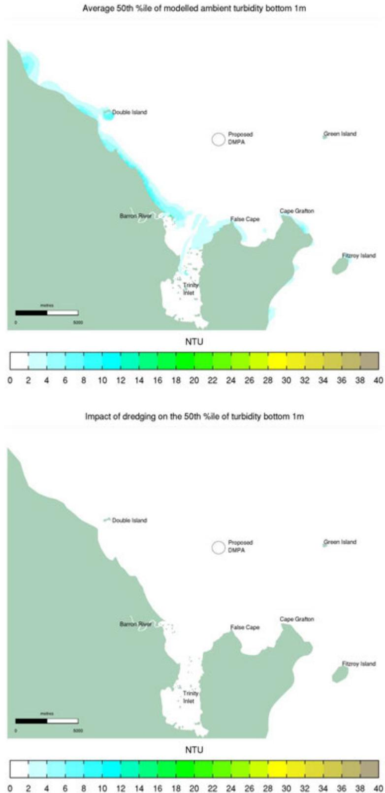
Figure 6-34 “Worst Case” Re-suspension Period 95<sup>th</sup> Percentile Bottom 1m Turbidity: Average Ambient Turbidity (top), Impact of Dredging (bottom)
