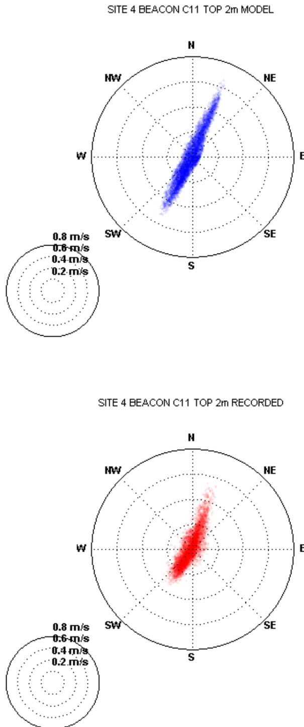
Figure D-7 Current Polar Plot Calibration – Beacon C11 Top 2m of Water Column
