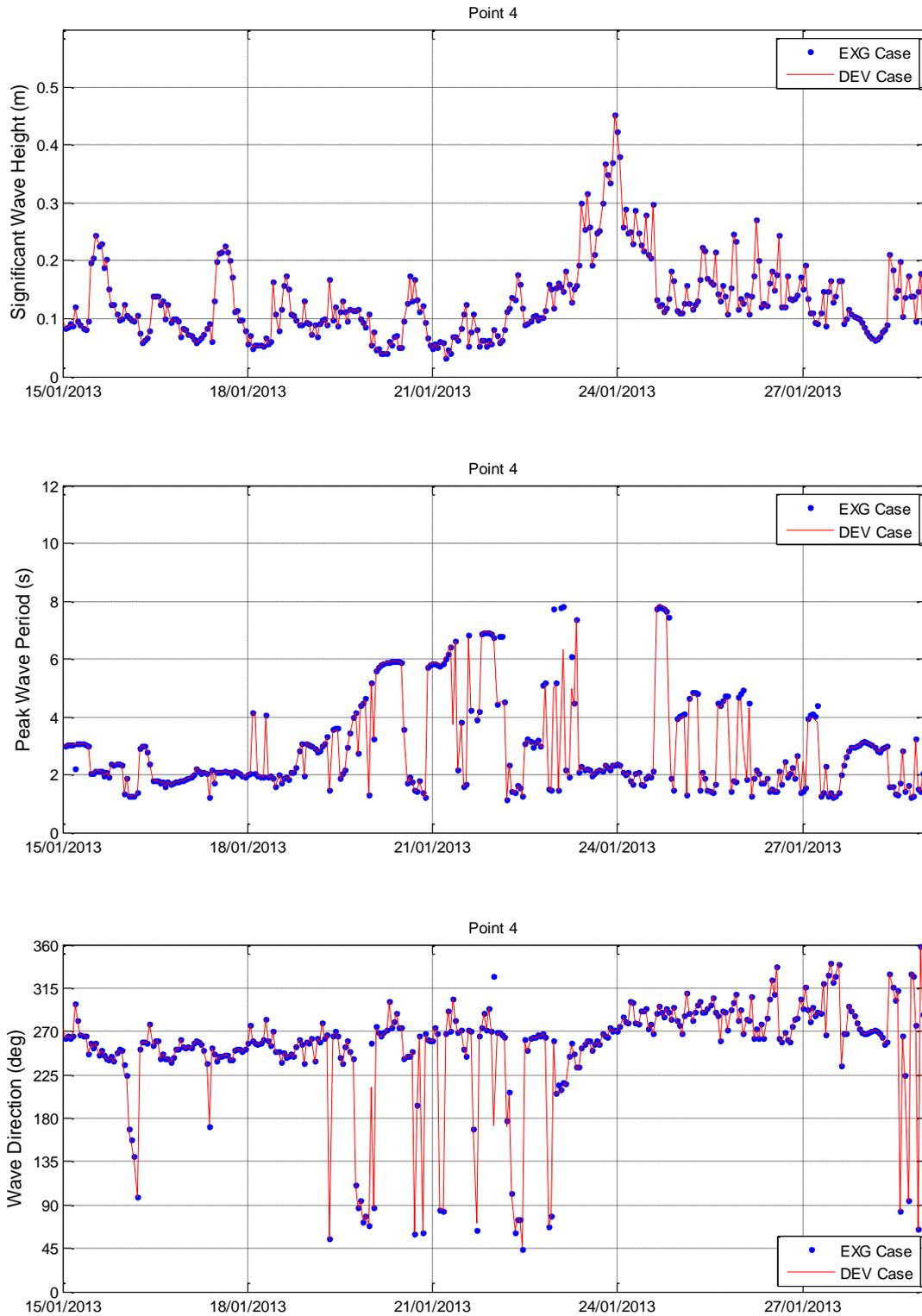
Figure 7-23 Existing Case and Developed Case Wave Parameter Timeseries Comparison (Nearshore Location Point 4 in Figure 7-2)
