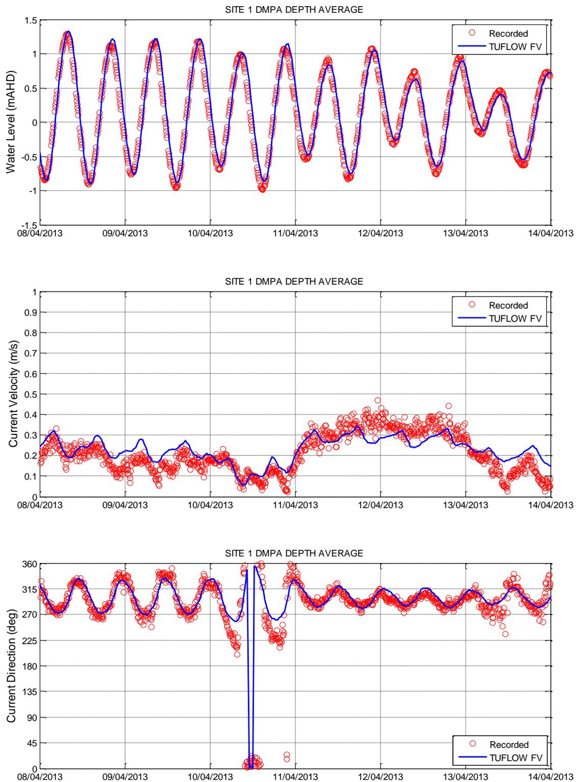
Figure 3-7 Hydrodynamic Model Calibration 3D Depth Average – Site 1 DMPA
