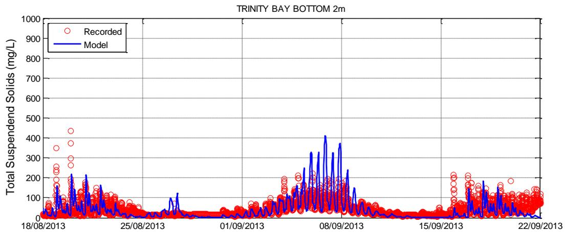
Figure 5-19 Sediment Re-suspension Validation – Trinity Bay
