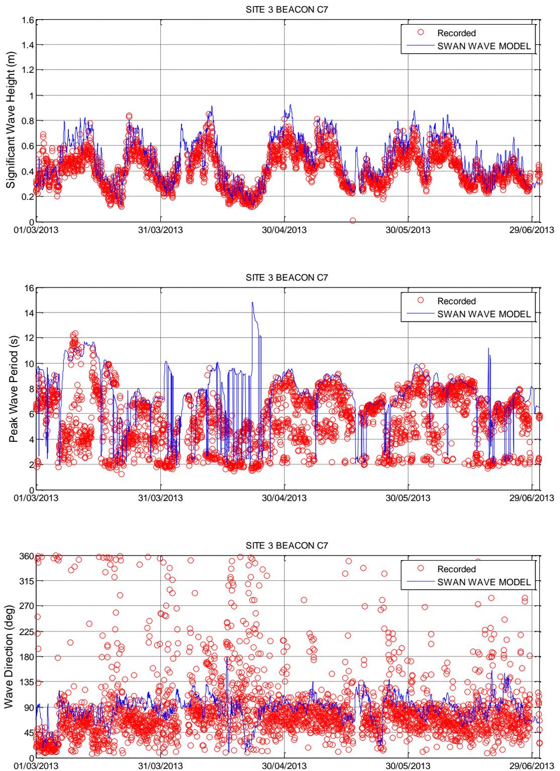
Figure 3-31 SWAN Wave Model Calibration – Site 3 Beacon C7
