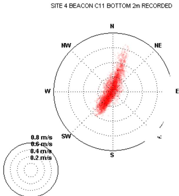
Figure D-8 Current Polar Plot Calibration – Beacon C11 Bottom 2m of Water Column
