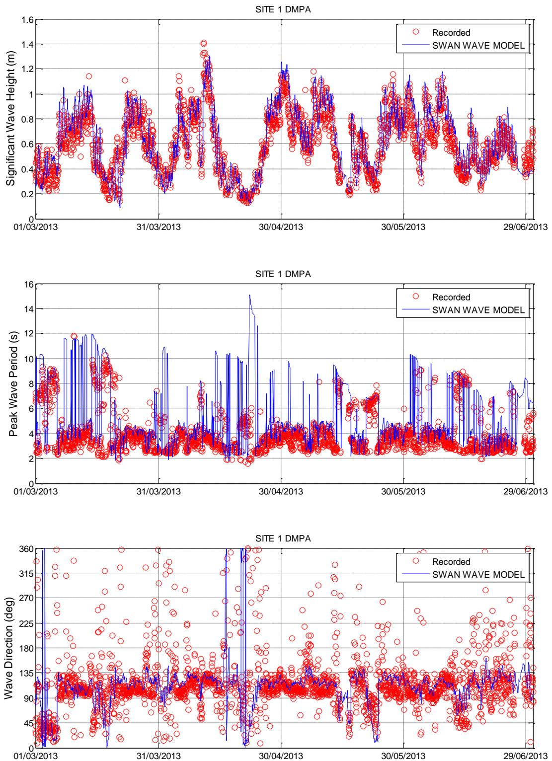
Figure 3-29 SWAN Wave Model Calibration – Site 1 DMPA
