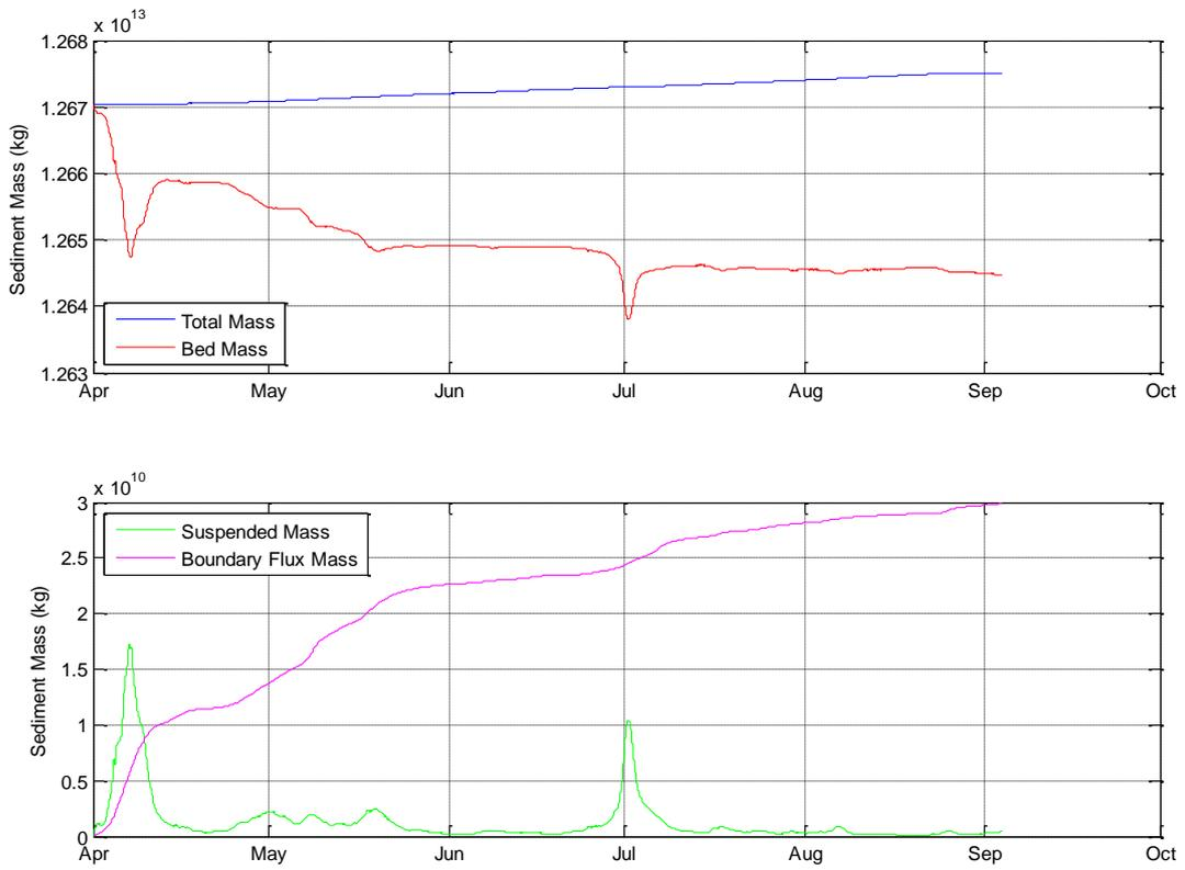
Figure 2. Sediment Mass Balance Checks - Capital Alternative Case
