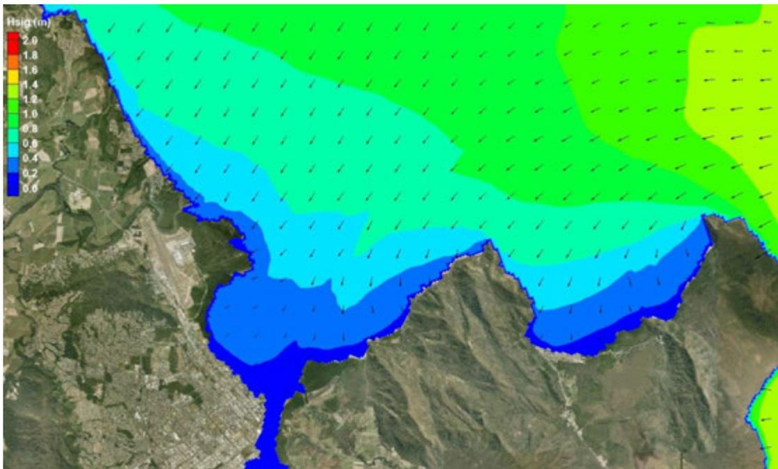
Figure 7-18 100m Grid Modelled Typical South-Easterly Wave Case (09/04/2013 13:00)
