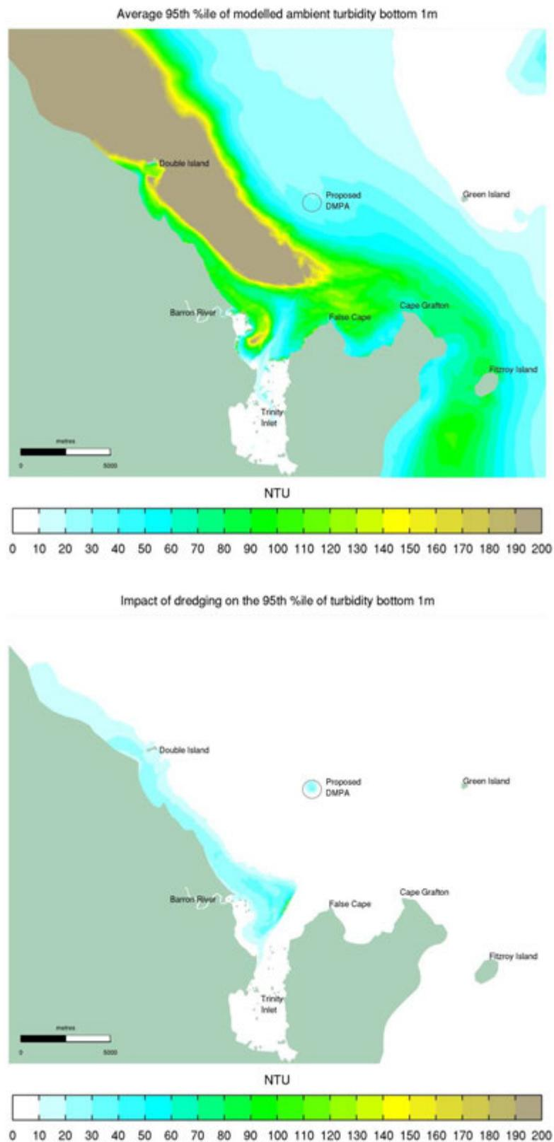
Figure 6-22 “Worst Case” Stiff Material Dredging 95<sup>th</sup> Percentile Bottom 1m Turbidity: Average Ambient Turbidity (top), Impact of Dredging (bottom)
