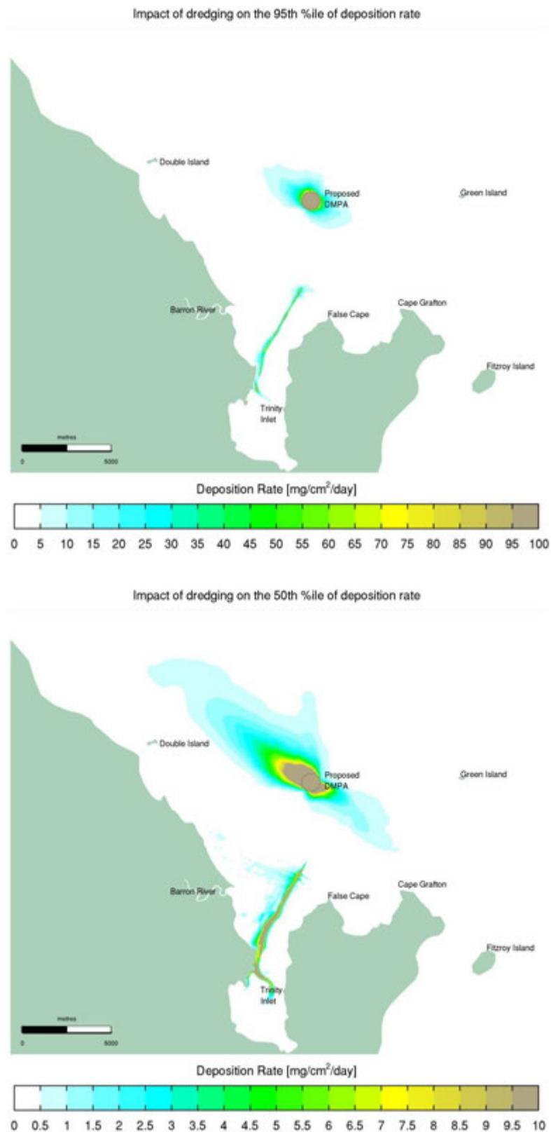
Figure 6-15 Alternative Case Capital Program Impact to Sediment Deposition Rate: 95th Percentile (top) and 50th Percentile (Bottom)
