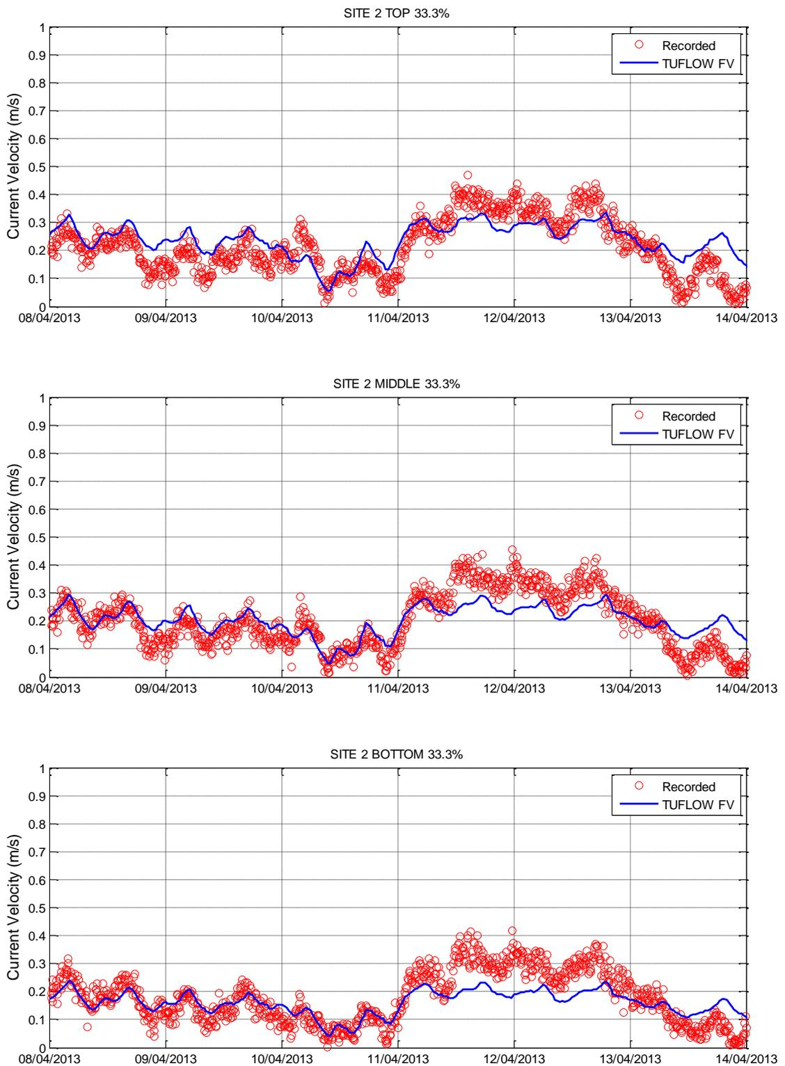
Figure 3-12 Hydrodynamic Model Calibration Current Velocity Layers – Site 2
