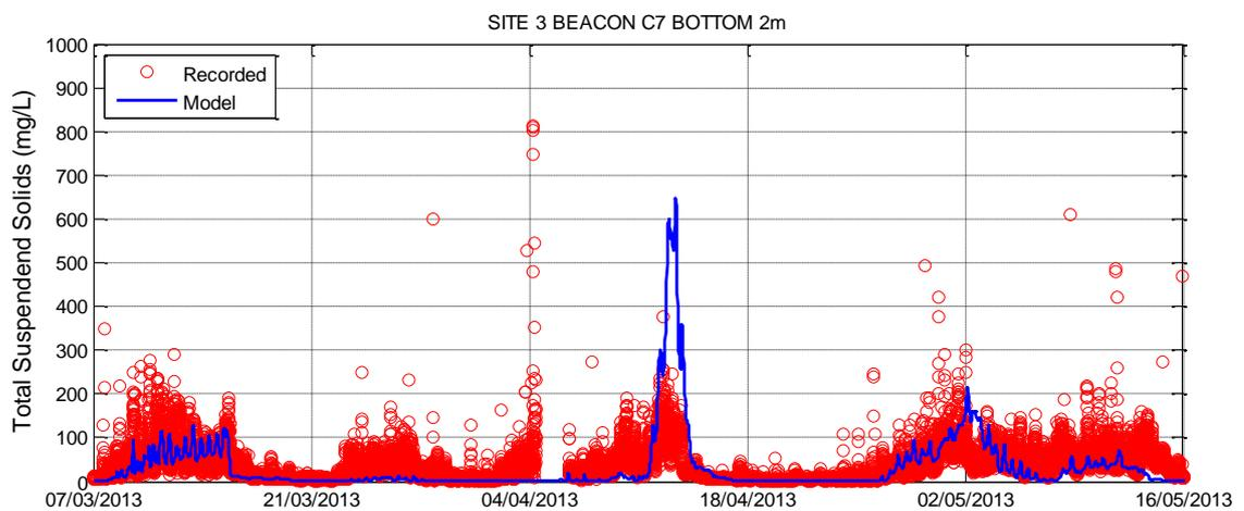
Figure 3-38 Sediment Re-suspension Calibration – Beacon C7
