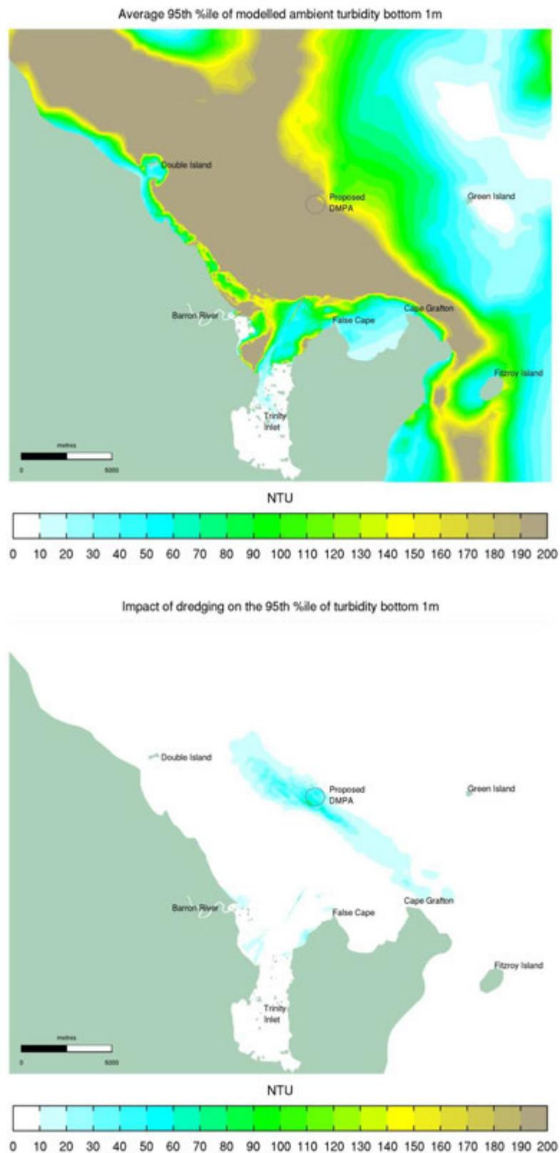
Figure 6-32 “Worst Case” Re-suspension Period 95<sup>th</sup> Percentile Bottom 1m Turbidity: Average Ambient Turbidity (top), Impact of Dredging (bottom)
