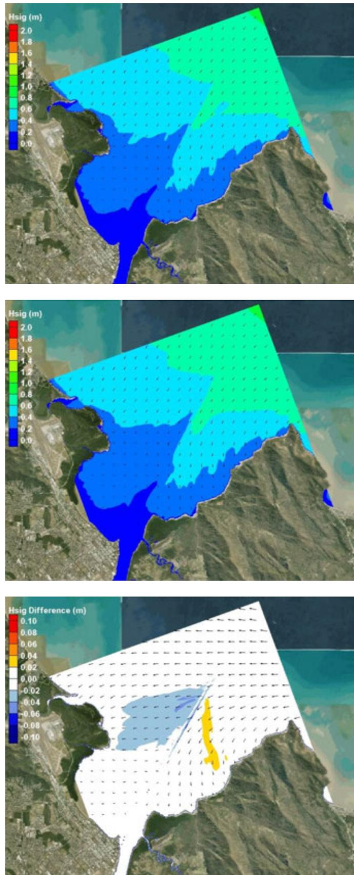
Figure 7-20 25m Grid Typical South-Easterly Wave Case: Base case (top); Developed case (middle); Difference (bottom)
