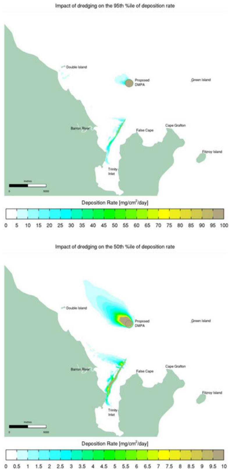
Figure 6-25 "Worst Case" Stiff Material Dredging Impact to Sediment Deposition Rate: 95th Percentile (top) and 50th Percentile (Bottom)
