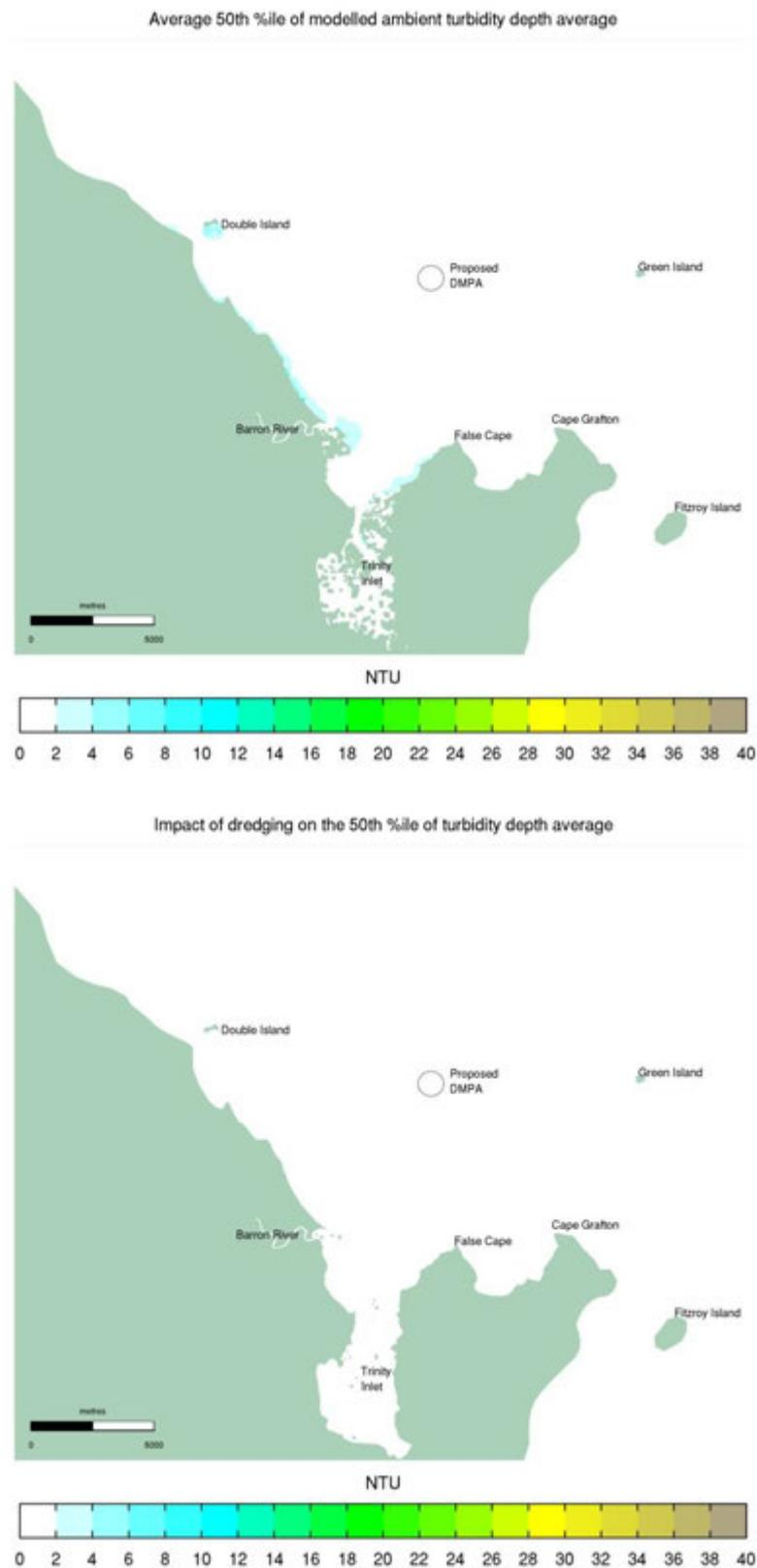
Figure 6-28 12mo Re-suspension Period 50<sup>th</sup> Percentile Depth Average Turbidity: Average Ambient Turbidity (top), Impact of Dredging (bottom)
