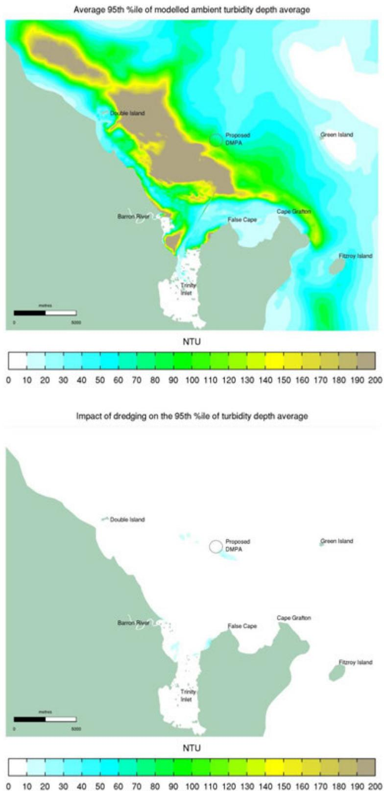
Figure 6-31 “Worst Case” Re-suspension Period 95<sup>th</sup> Percentile Depth Average Turbidity: Average Ambient Turbidity (top), Impact of Dredging (bottom)
