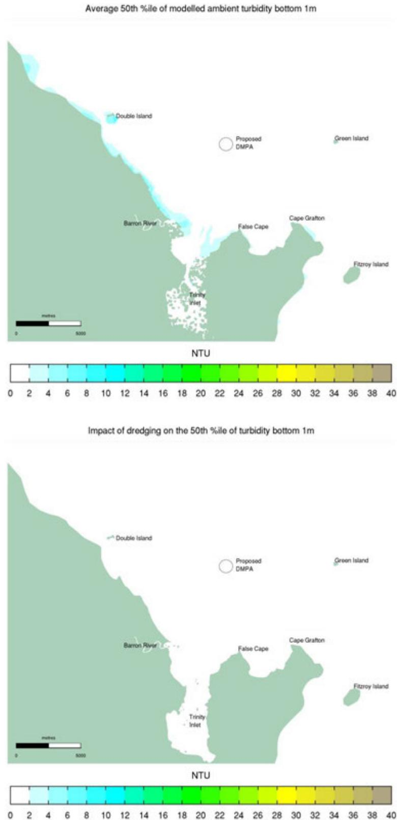
Figure 6-29 12mo Re-suspension Period 50<sup>th</sup> Percentile Bottom 1m Turbidity: Average Ambient Turbidity (top), Impact of Dredging (bottom)
