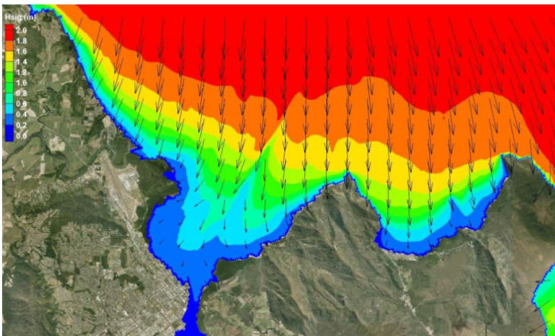
Figure 7-19 100m Grid Modelled Typical Northerly Wave Case (24/01/2013 07:00)
