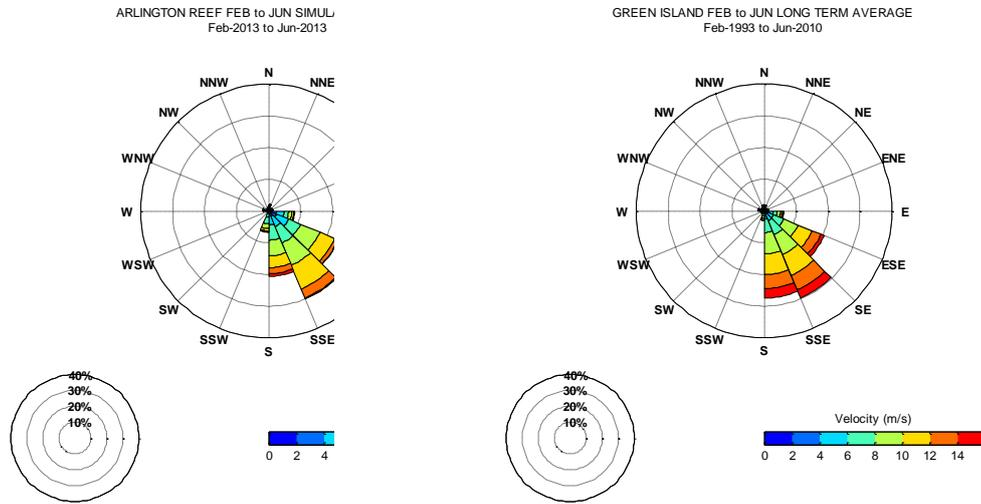
Figure 3-3 Offshore Wind Roses – February to June 2013 Simulation Period (top) and February to June Long Term Average (bottom)
