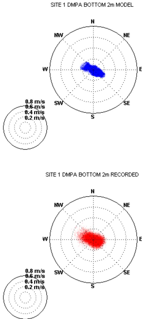
Figure G-1 Current Polar Plot Calibration – Site 1 Bottom 2m of Water Column
