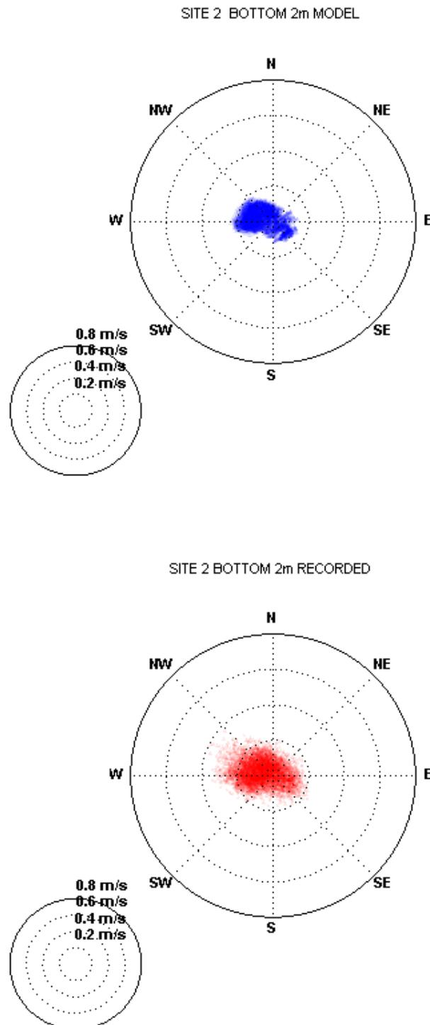
Figure D-4 Current Polar Plot Calibration – Site 2 Bottom 2m of Water Column
