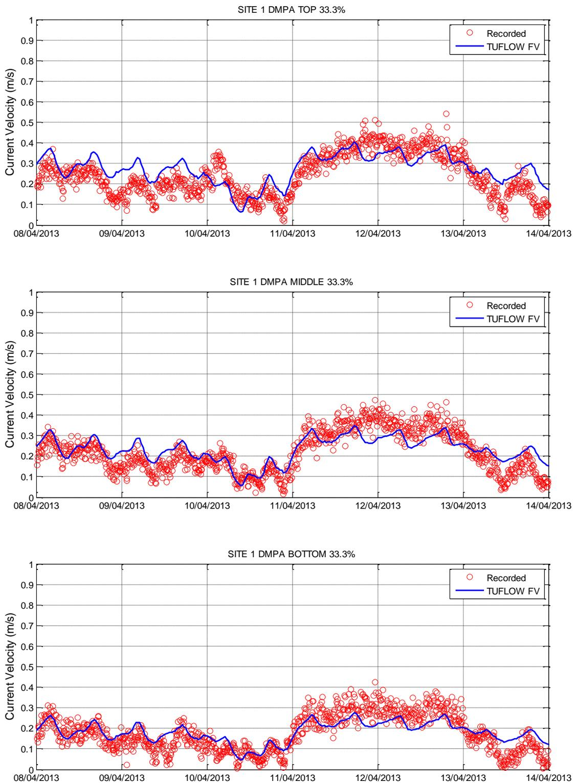
Figure 3-8 Hydrodynamic Model Calibration Current Velocity Layers – Site 1 DMPA
