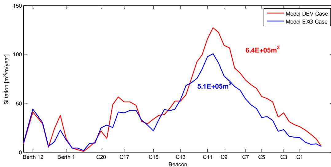
Figure 7-25 Modelled Existing Case and Developed Case Channel Siltation
