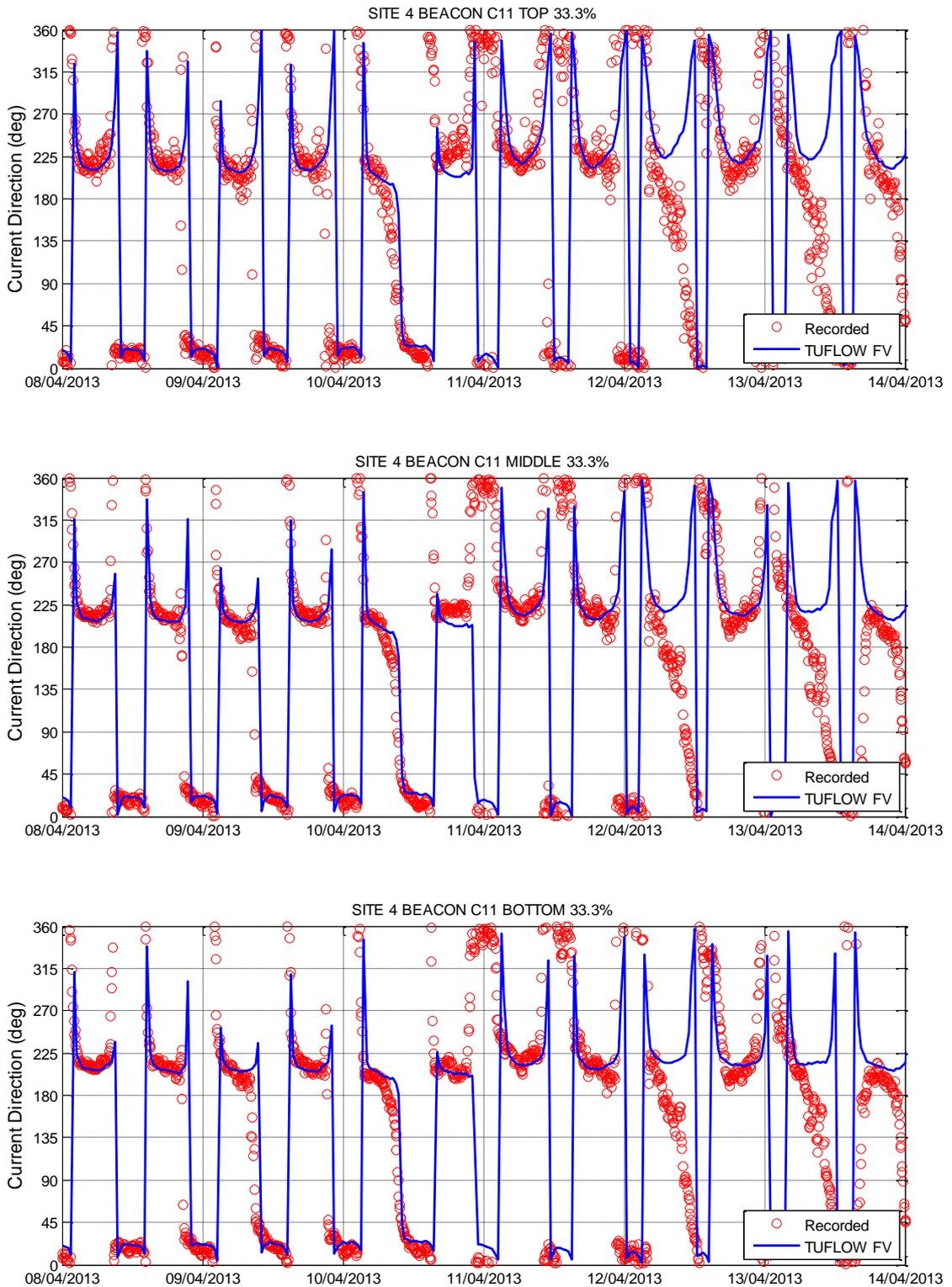
Figure 3-21 Hydrodynamic Model Calibration Current Direction Layers – Site 4 Beacon C11
