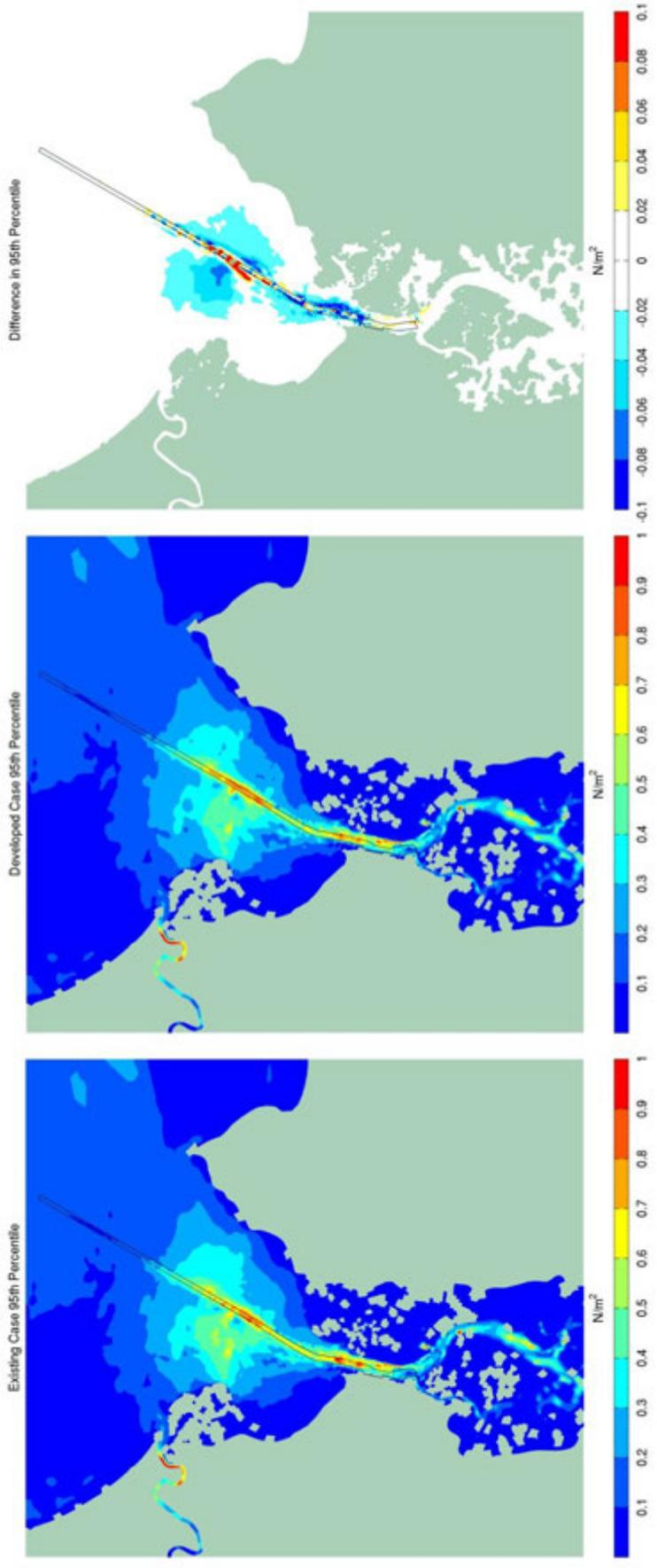
Figure 7-14 Modelled 95th Percentile Current Related Bed Shear Stress ( $N/m^2$ ) and Impacts. Existing case (left); Developed case (middle) and Impacts (right)
