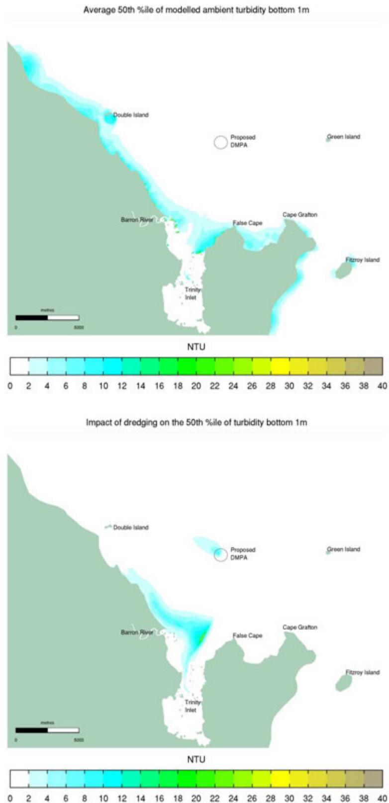
Figure 6-19 “Worst Case” Soft Material Dredging 95<sup>th</sup> Percentile Bottom 1m Turbidity: Average Ambient Turbidity (top), Impact of Dredging (bottom)
