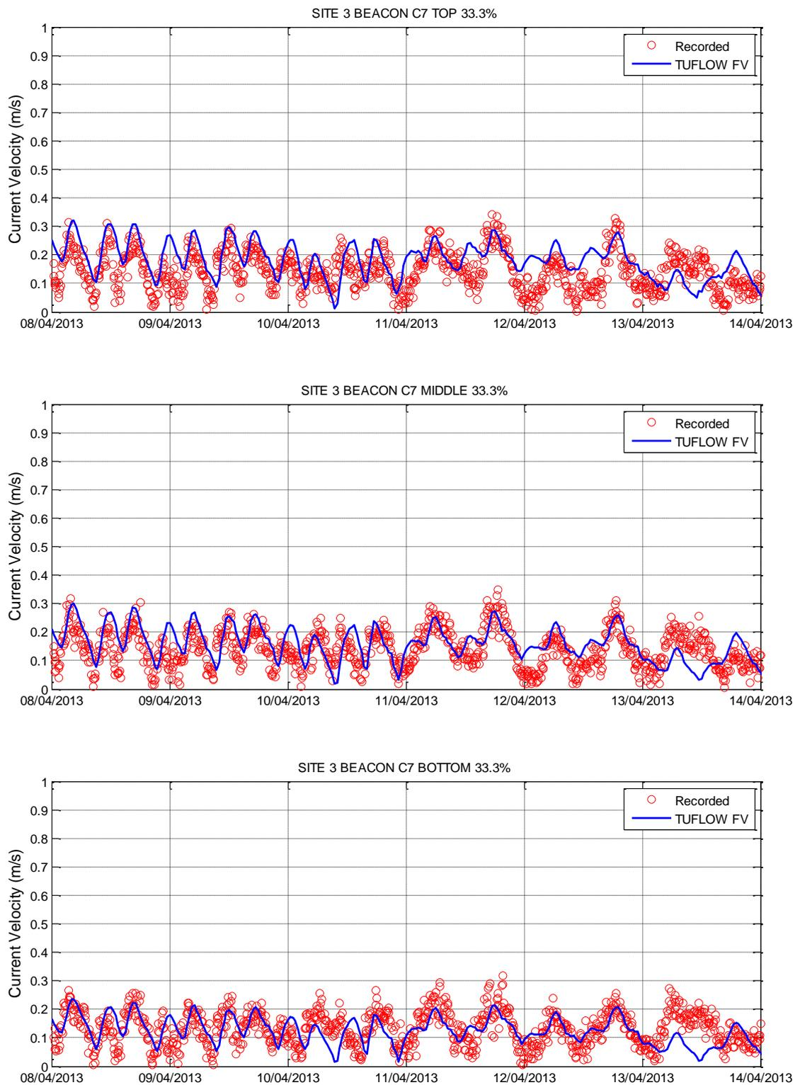
Figure 3-16 Hydrodynamic Model Calibration Current Velocity Layers – Site 3 Beacon C7
