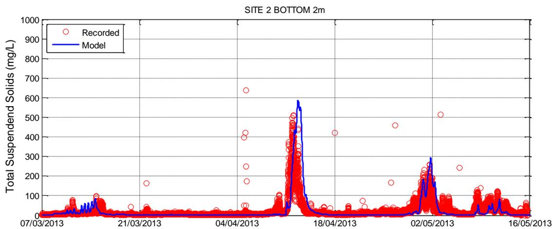
Figure 3-37 Sediment Re-suspension Calibration – Site 2
