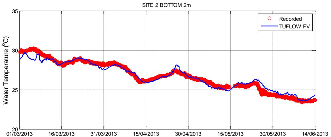
Figure 3-24 Hydrodynamic Model Calibration Near Bed Temperature – Site 2
