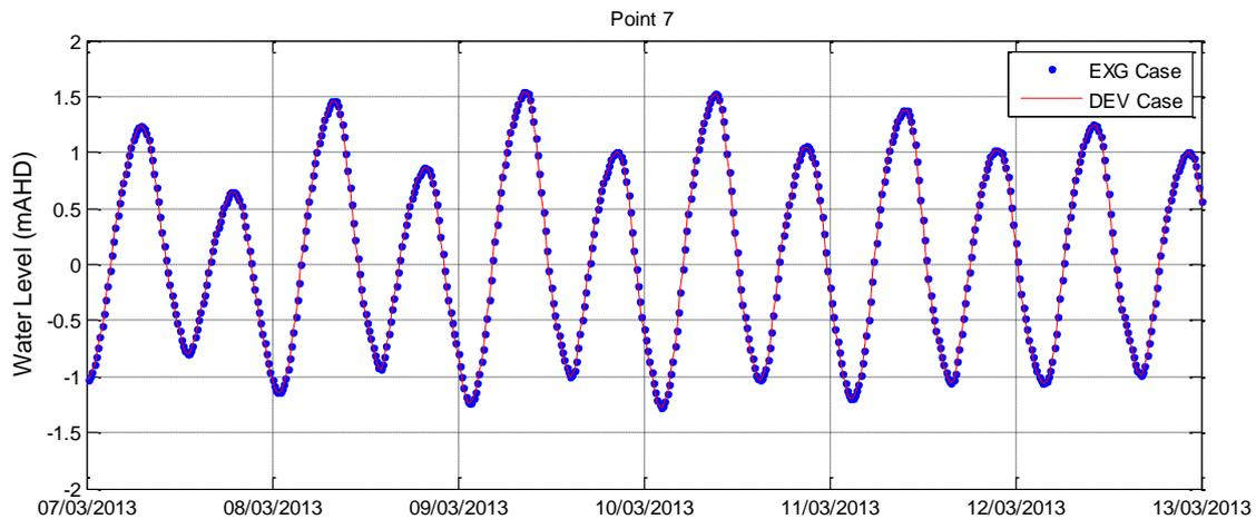
Figure 7-12 Existing and Developed Case Water Level Timeseries (Point 7).
