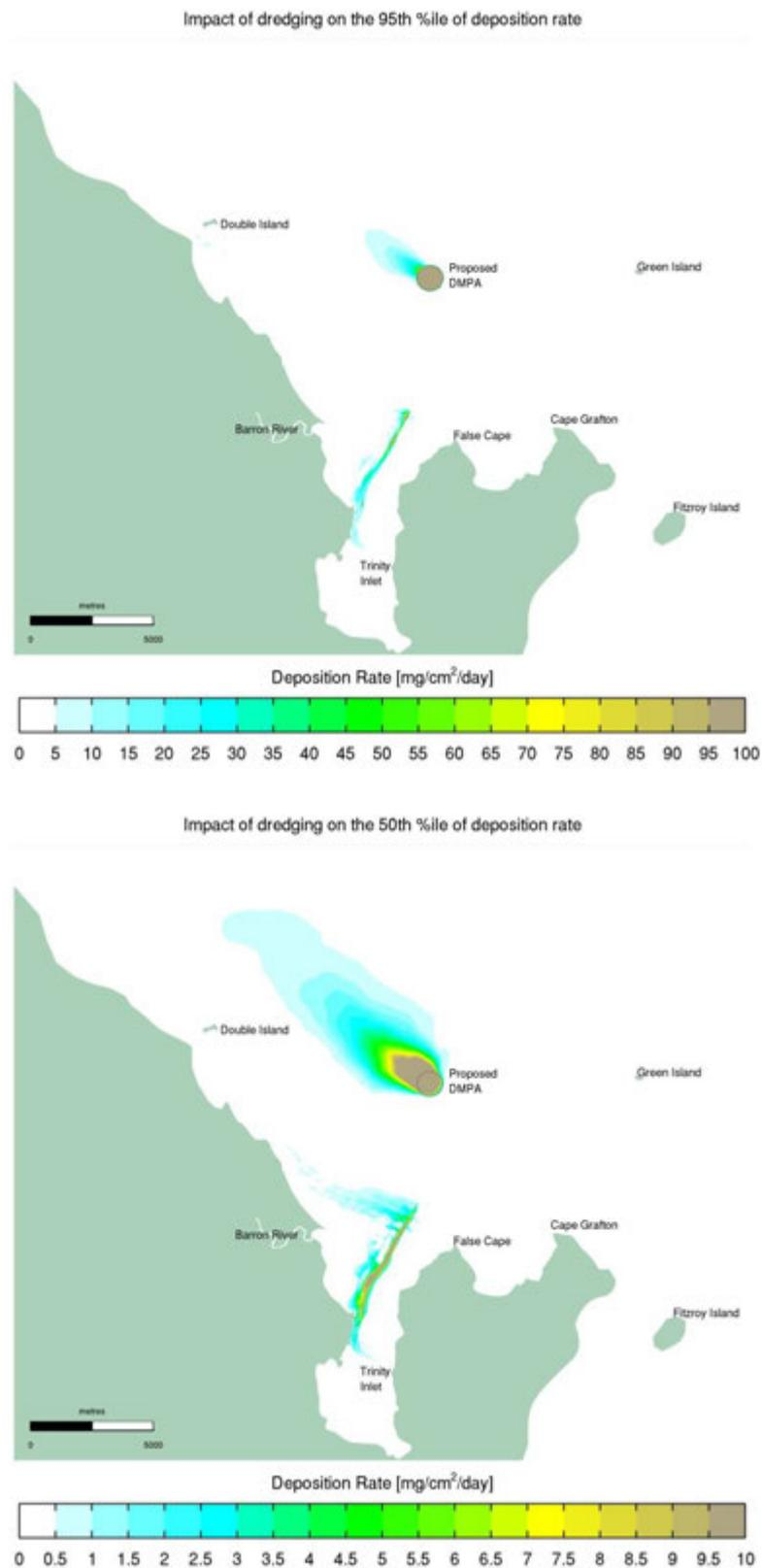
Figure 6-20 “Worst Case” Soft Material Dredging Impact to Sediment Deposition Rate: 95th Percentile (top) and 50th Percentile (Bottom)
