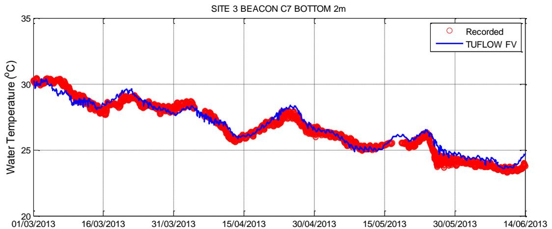
Figure 3-25 Hydrodynamic Model Calibration Near Bed Temperature – Site 3 Beacon C7
