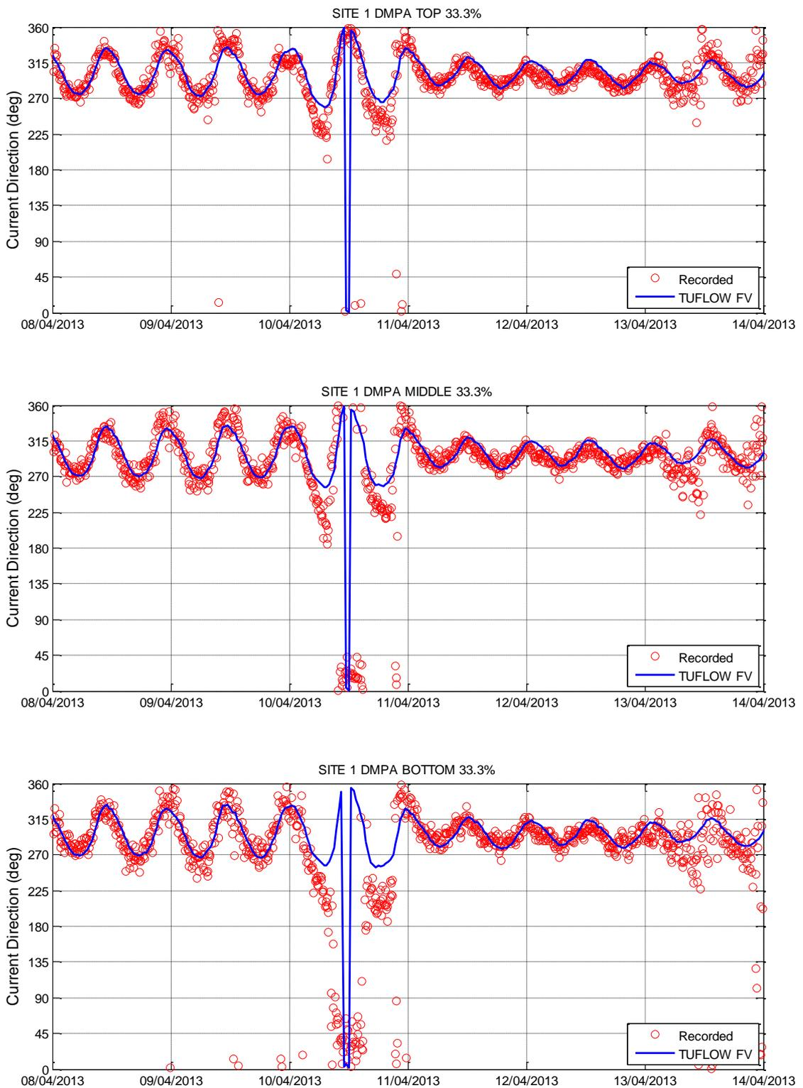
Figure 3-9 Hydrodynamic Model Calibration Current Direction Layers – Site 1 DMPA
