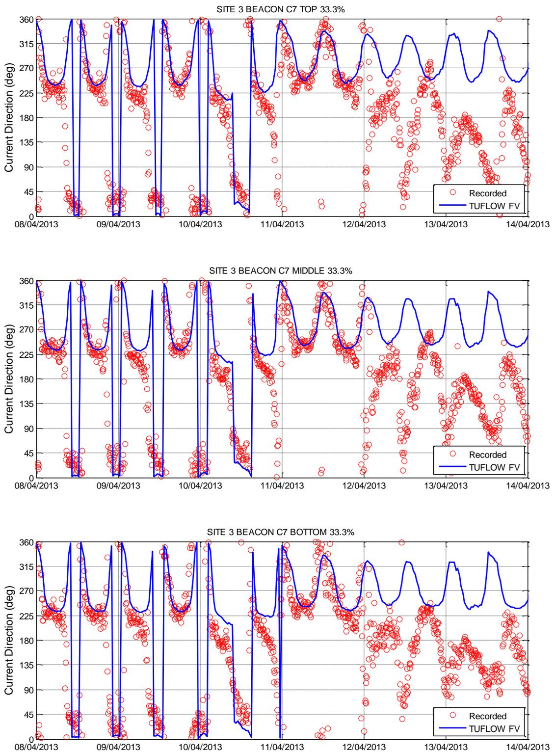
Figure 3-17 Hydrodynamic Model Calibration Current Direction Layers – Site 3 Beacon C7
