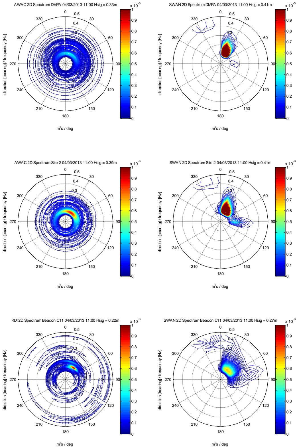
Figure 3-33 Recorded (left) and Predicted (right) 2D Wave Energy Spectrum: Dominant Swell State
