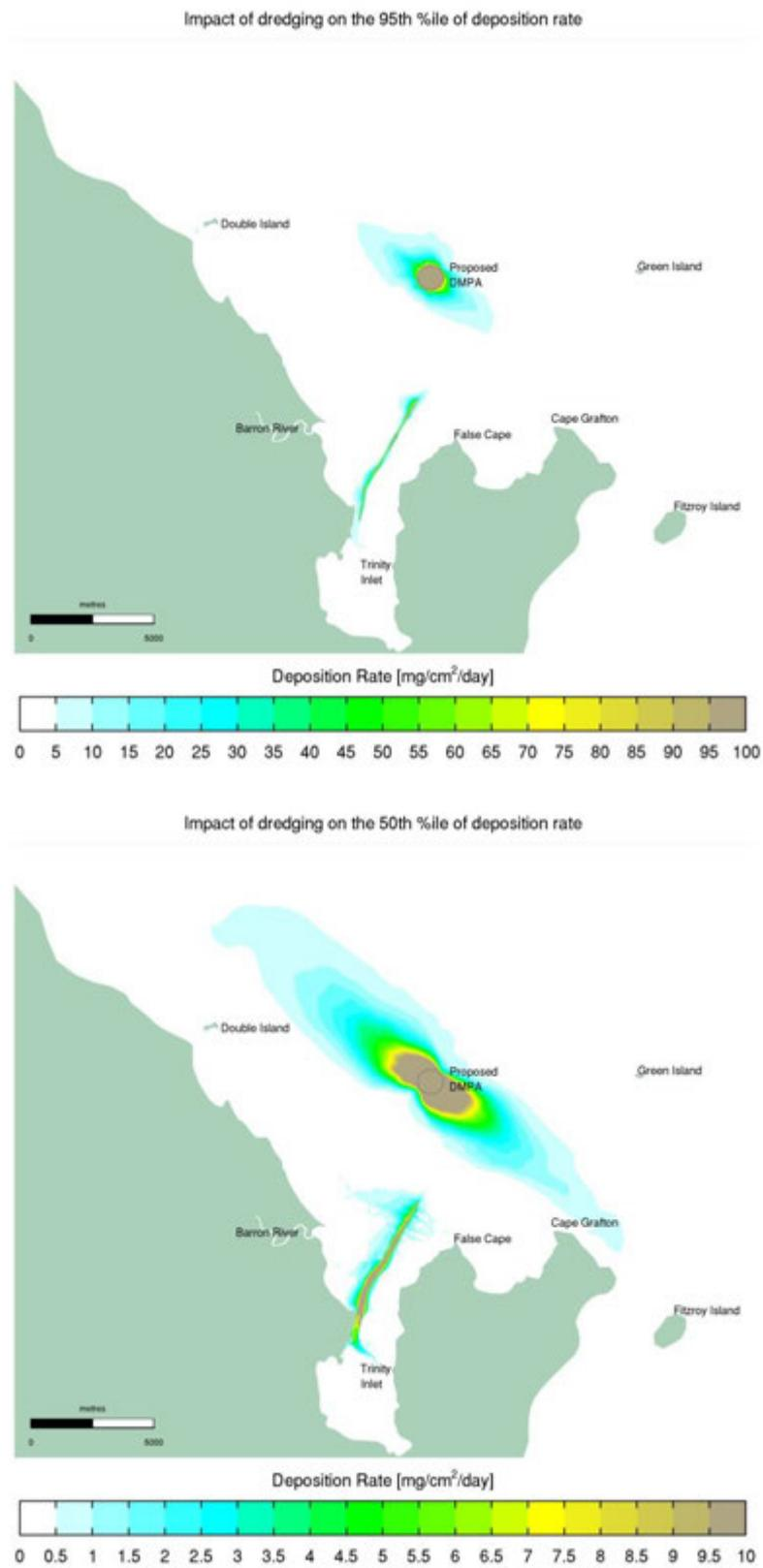
Figure 6-10 Base Case Capital Program Impact to Sediment Deposition Rate: 95th Percentile (top) and 50th Percentile (Bottom)
