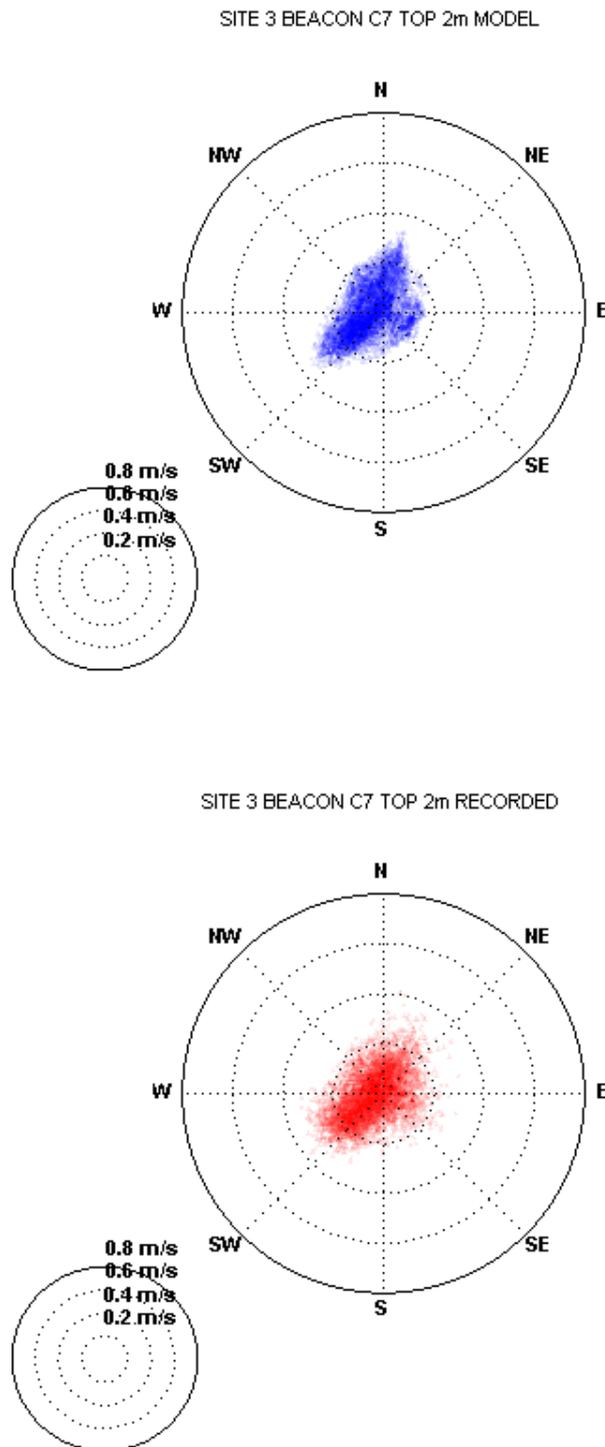
Figure D-5 Current Polar Plot Calibration – Beacon C7 Top 2m of Water Column
