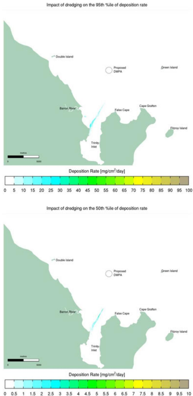
Figure 6-30 12mo Re-suspension Period Impact to Sediment Deposition Rate: 95th Percentile (top) and 50th Percentile (Bottom)
