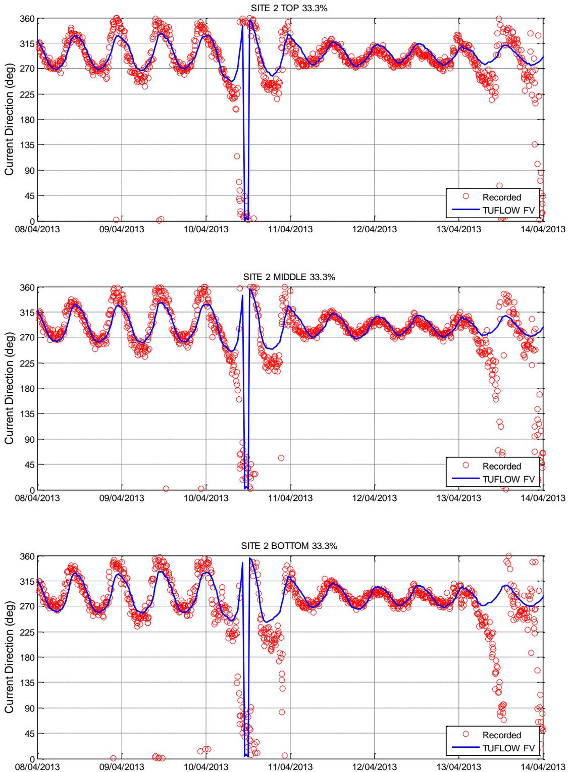
Figure 3-13 Hydrodynamic Model Calibration Current Direction Layers – Site 2
