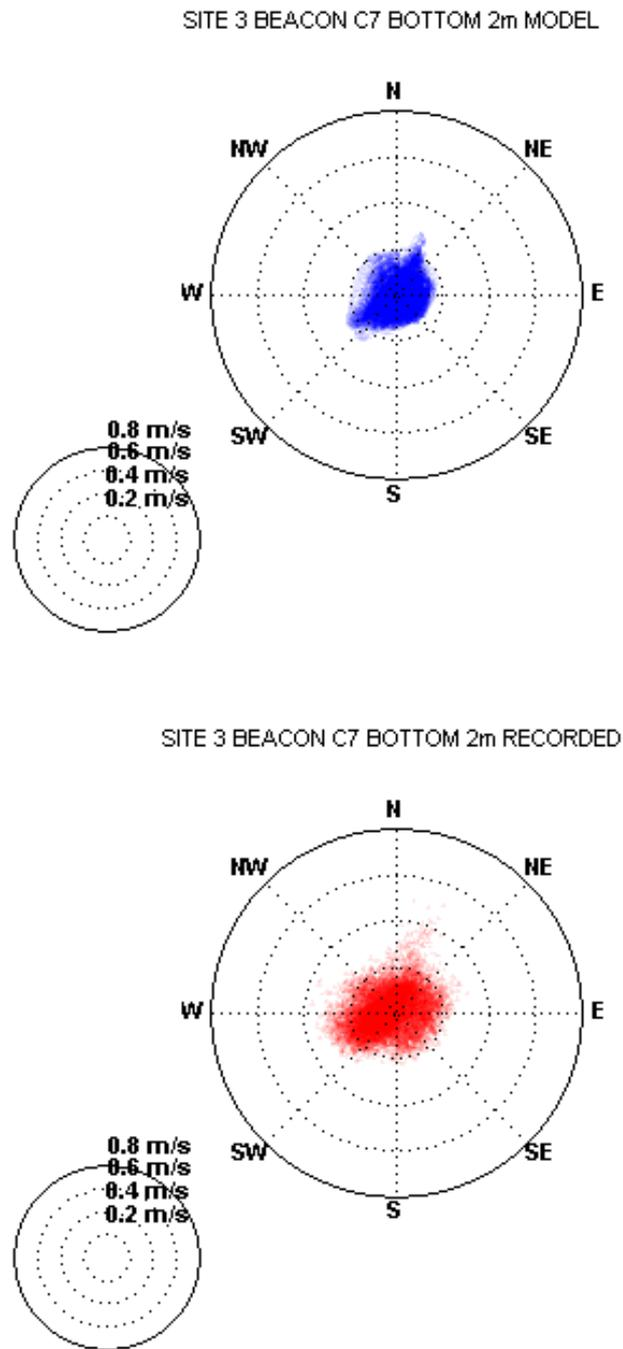
Figure G-3 Current Polar Plot Calibration – Site 3 Bottom 2m of Water Column
