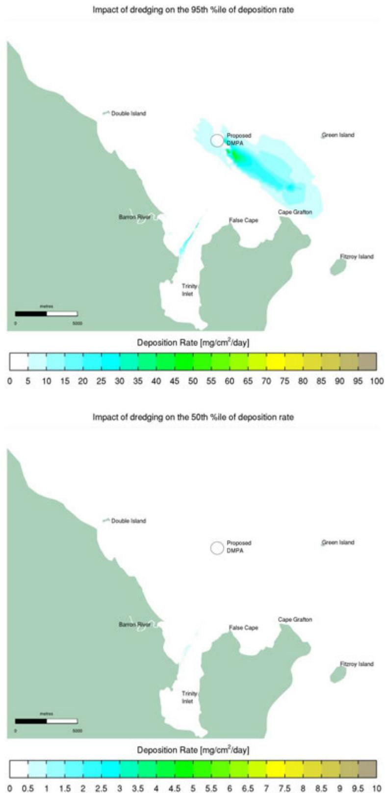
Figure 6-35 “Worst Case” Re-suspension Period Impact to Sediment Deposition Rate: 95th Percentile (top) and 50th Percentile (Bottom)
