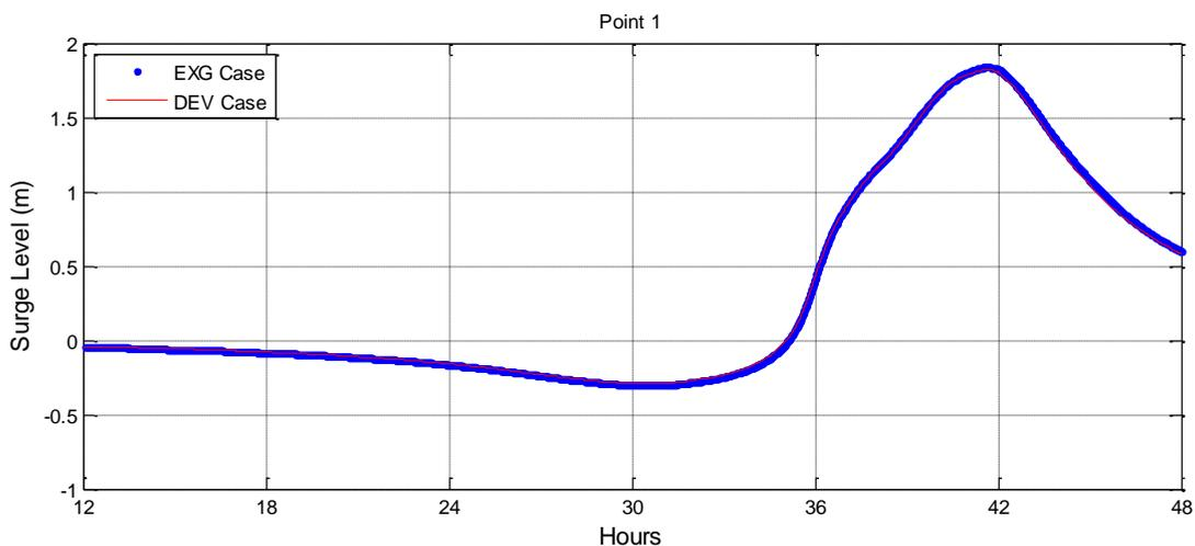
Figure 7-16 Existing and Developed Case Surge Level Timeseries (Point 1 – Inner Port).
