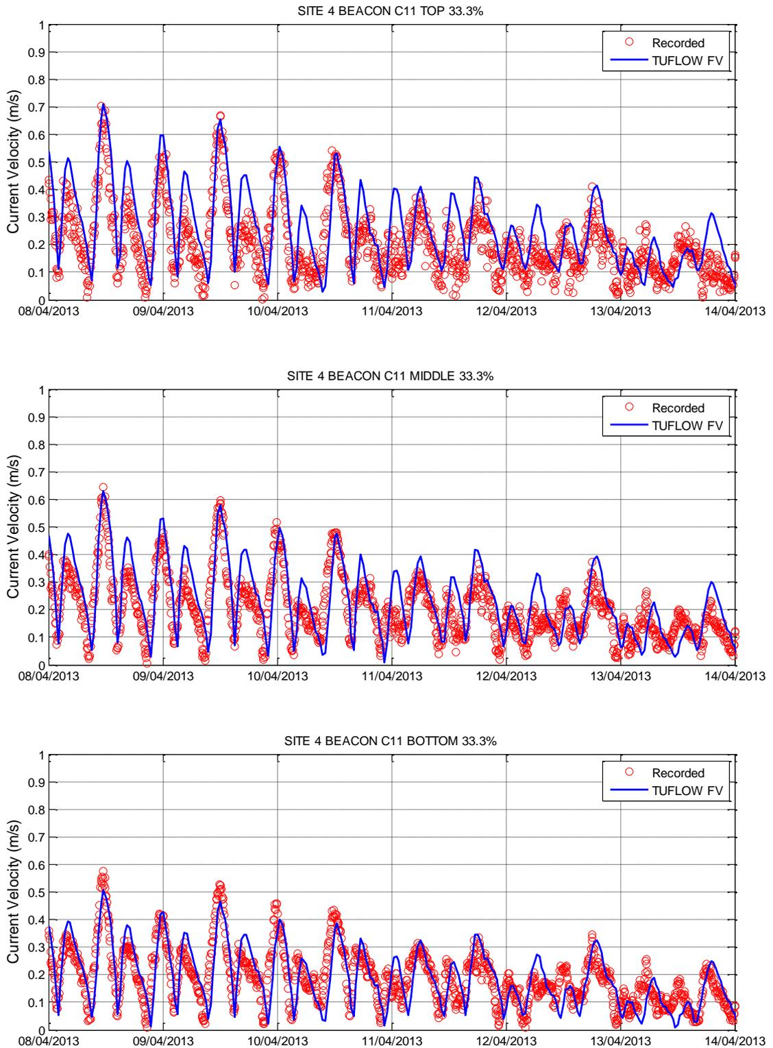
Figure 3-20 Hydrodynamic Model Calibration Current Velocity Layers – Site 4 Beacon C11
