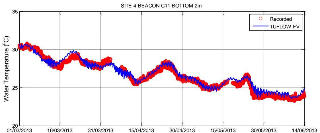
Figure 3-26 Hydrodynamic Model Calibration Near Bed Temperature – Site 4 Beacon C11
