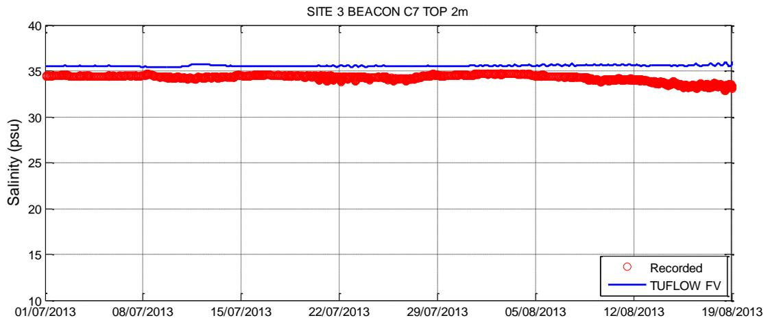
**Figure 5-16 Hydrodynamic Model Validation Surface Salinity – Site 3 Beacon C7**
