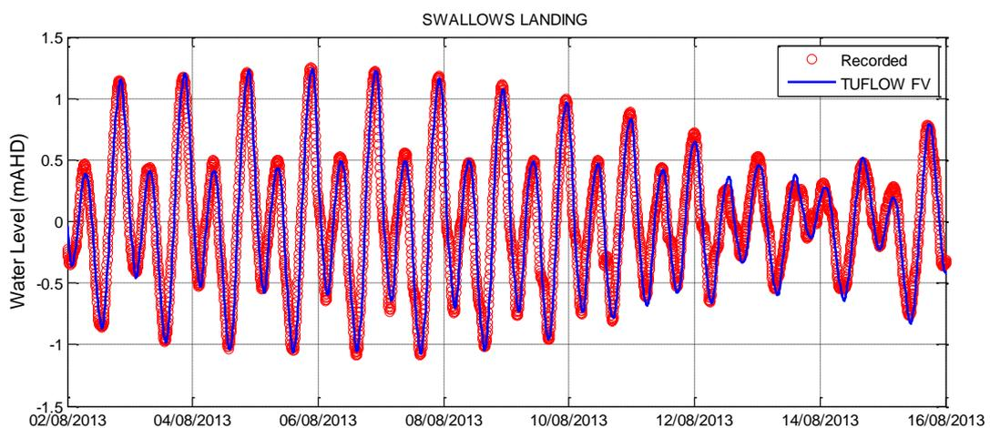
Figure 5-13 Hydrodynamic Model Validation Water Level – Swallows Landing
