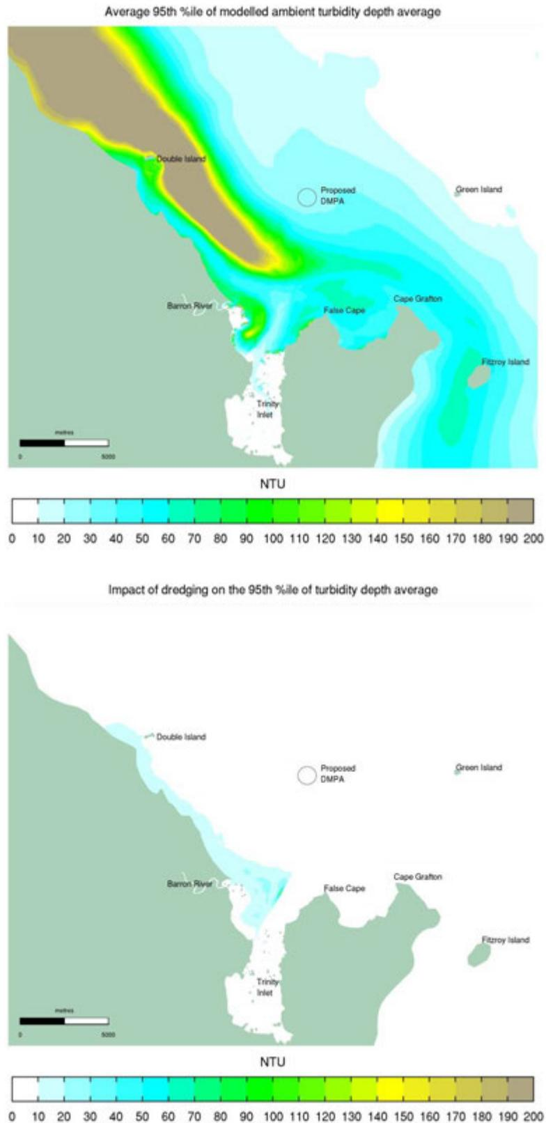
Figure 6-16 “Worst Case” Soft Material Dredging 95<sup>th</sup> Percentile Depth Average Turbidity: Average Ambient Turbidity (top), Impact of Dredging (bottom)
