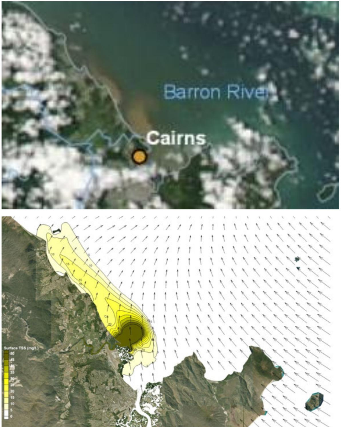
Figure 5-24 Barron River Flood Plume on 05/02/2011 - MODIS Satellite Image (top) and Predicted Surface TSS with Wind Vectors (bottom)
