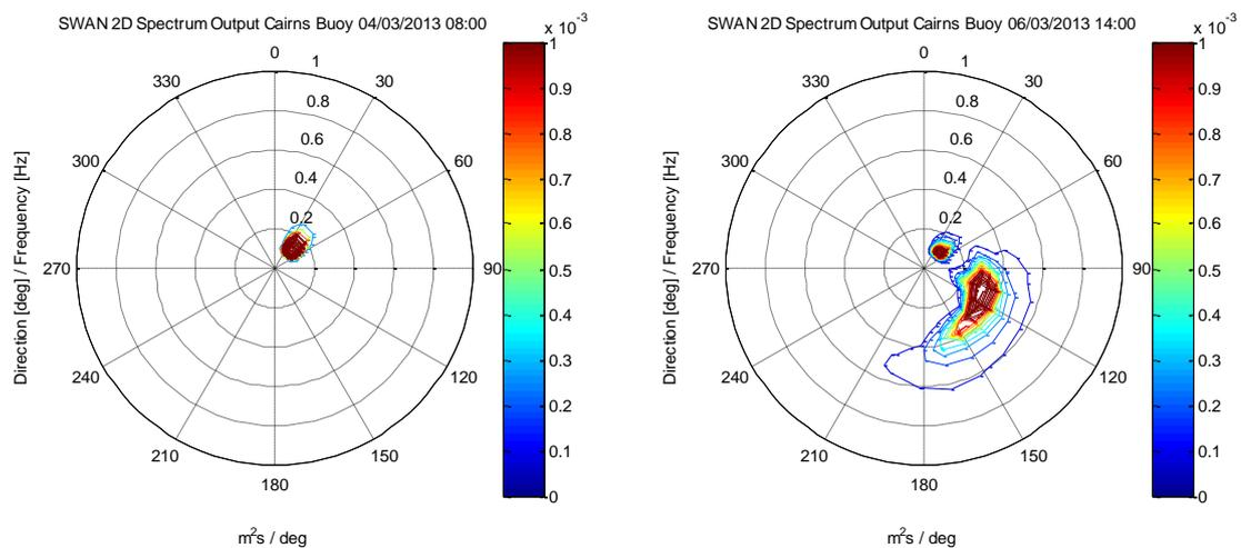
**Figure 3-27 Example Wave Energy Spectrum showing Dominant Swell (left) and Wind Generated Sea (right) States**
