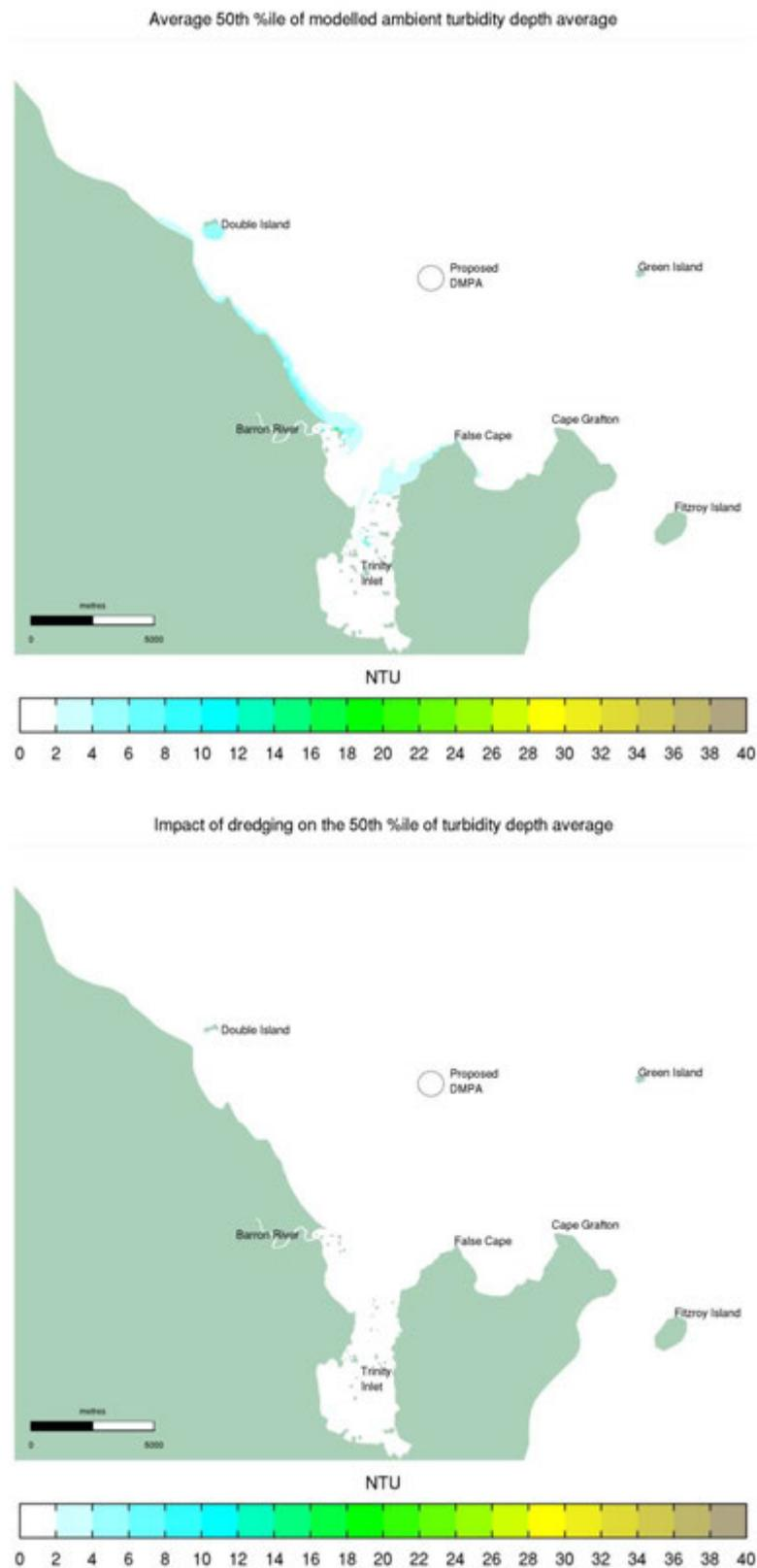
Figure 6-33 “Worst Case” Re-suspension Period 50<sup>th</sup> Percentile Depth Average Turbidity: Average Ambient Turbidity (top), Impact of Dredging (bottom)
