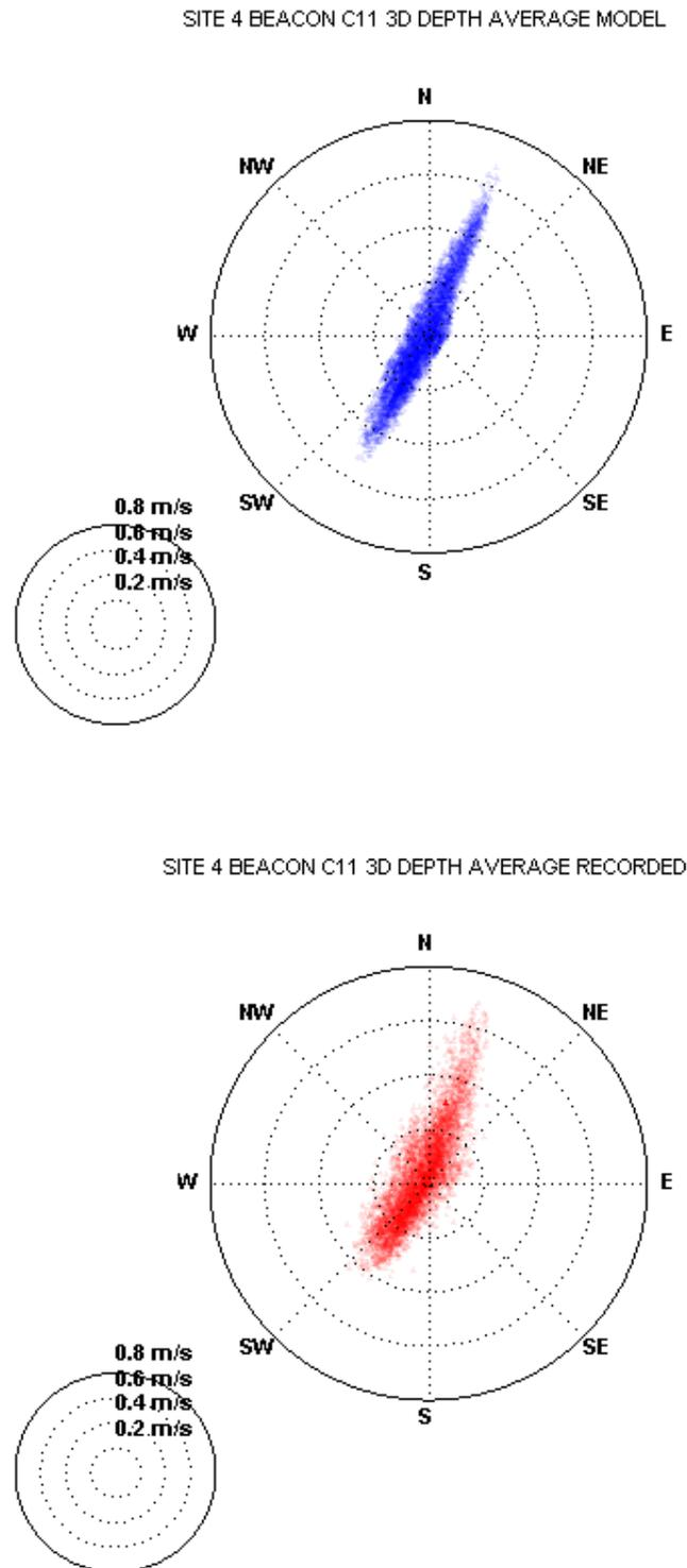
Figure 3-22 Current Polar Plot Validation – Site 4 Beacon C11
