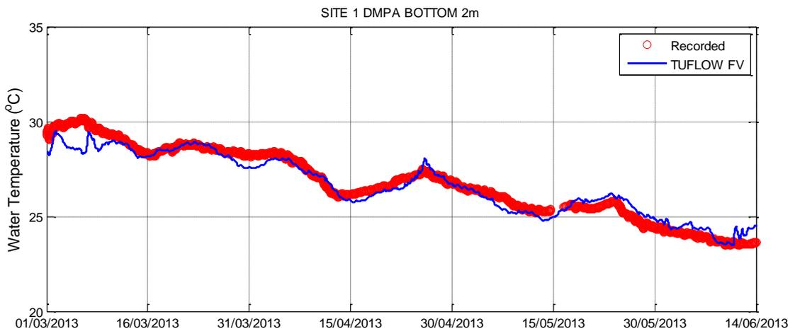
Figure 3-23 Hydrodynamic Model Calibration Near Bed Temperature – Site 1 DMPA
