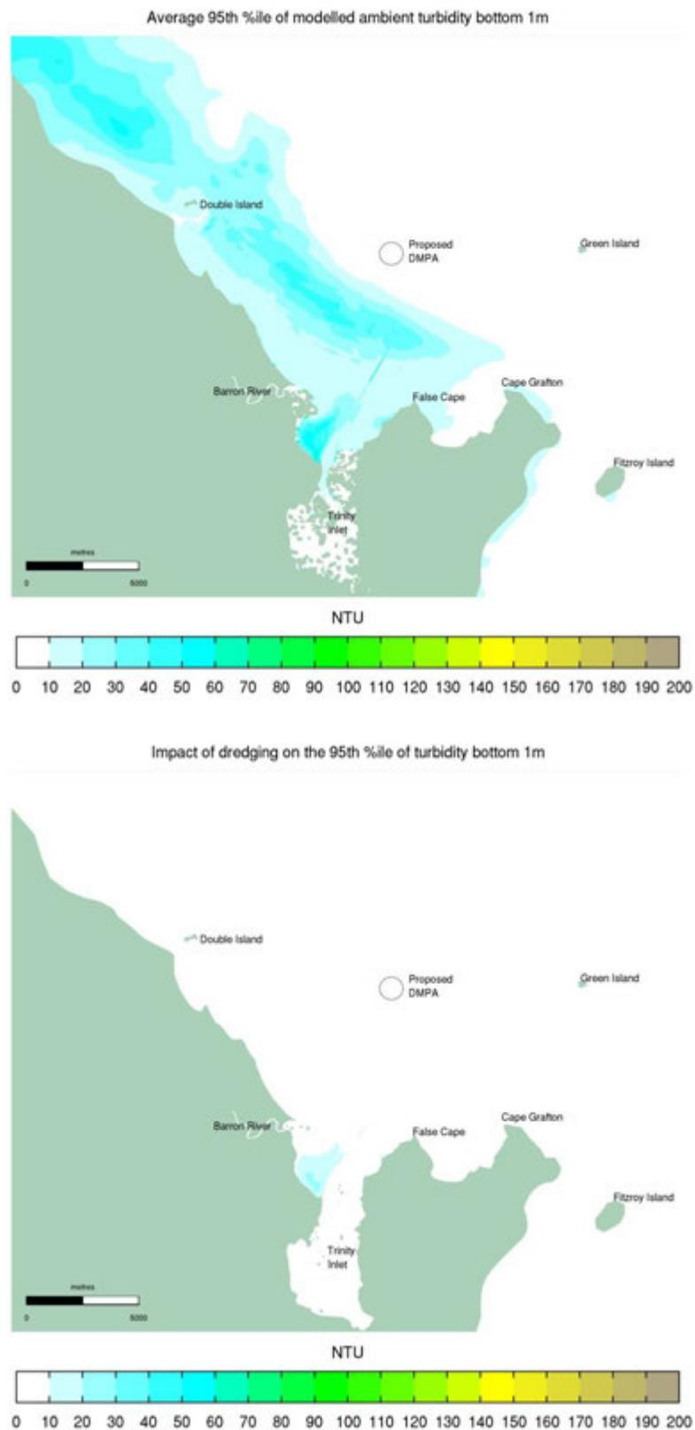
Figure 6-27 12mo Re-suspension Period 95<sup>th</sup> Percentile Bottom 1m Turbidity: Average Ambient Turbidity (top), Impact of Dredging (bottom)
