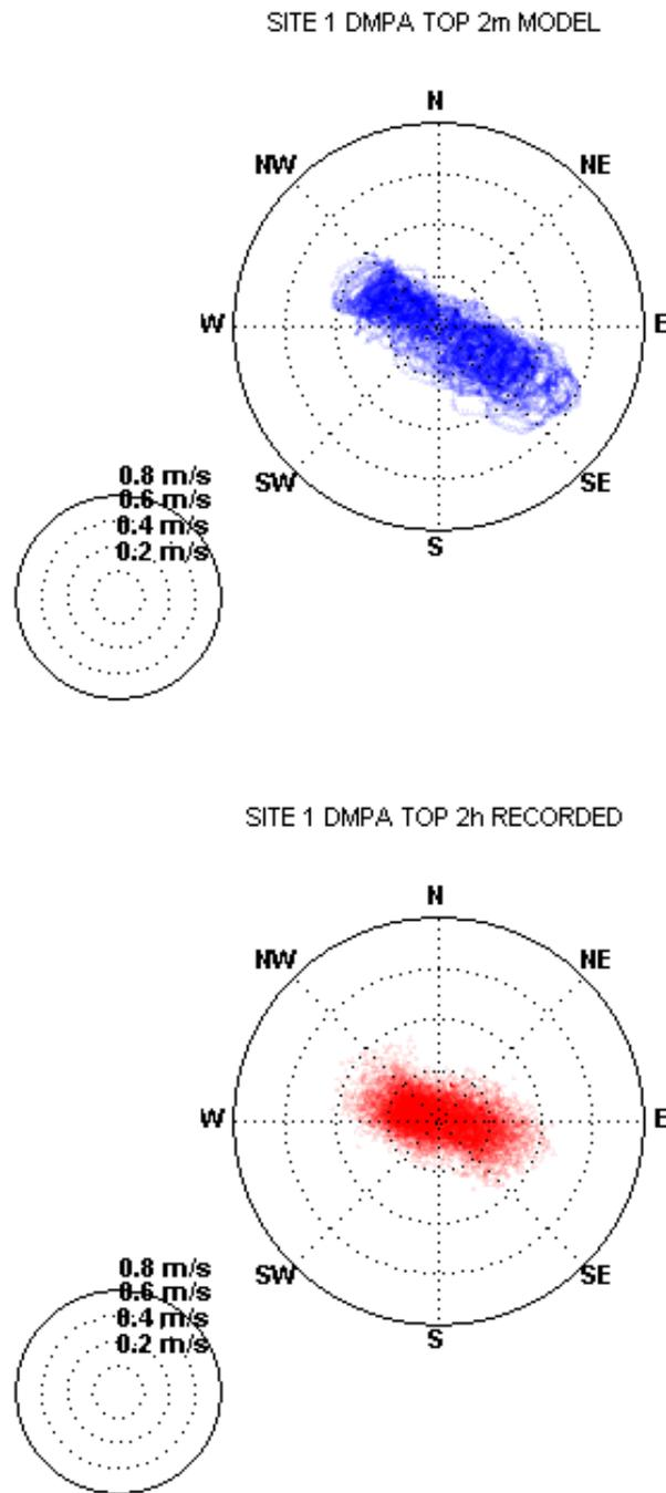
Figure G-2 Current Polar Plot Calibration – Site 1 Tom 2m of Water Column
