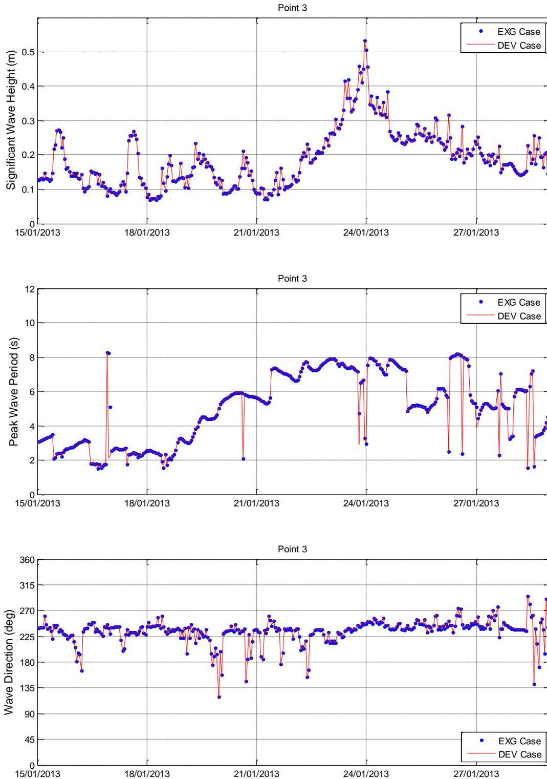
Figure 7-22 Existing Case and Developed Case Wave Parameter Timeseries Comparison (Nearshore Location Point 3 in Figure 7-2)
