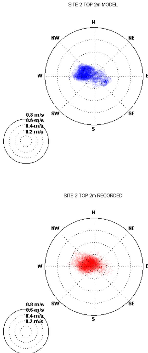
Figure D-3 Current Polar Plot Calibration – Site 2 Top 2m of Water Column
