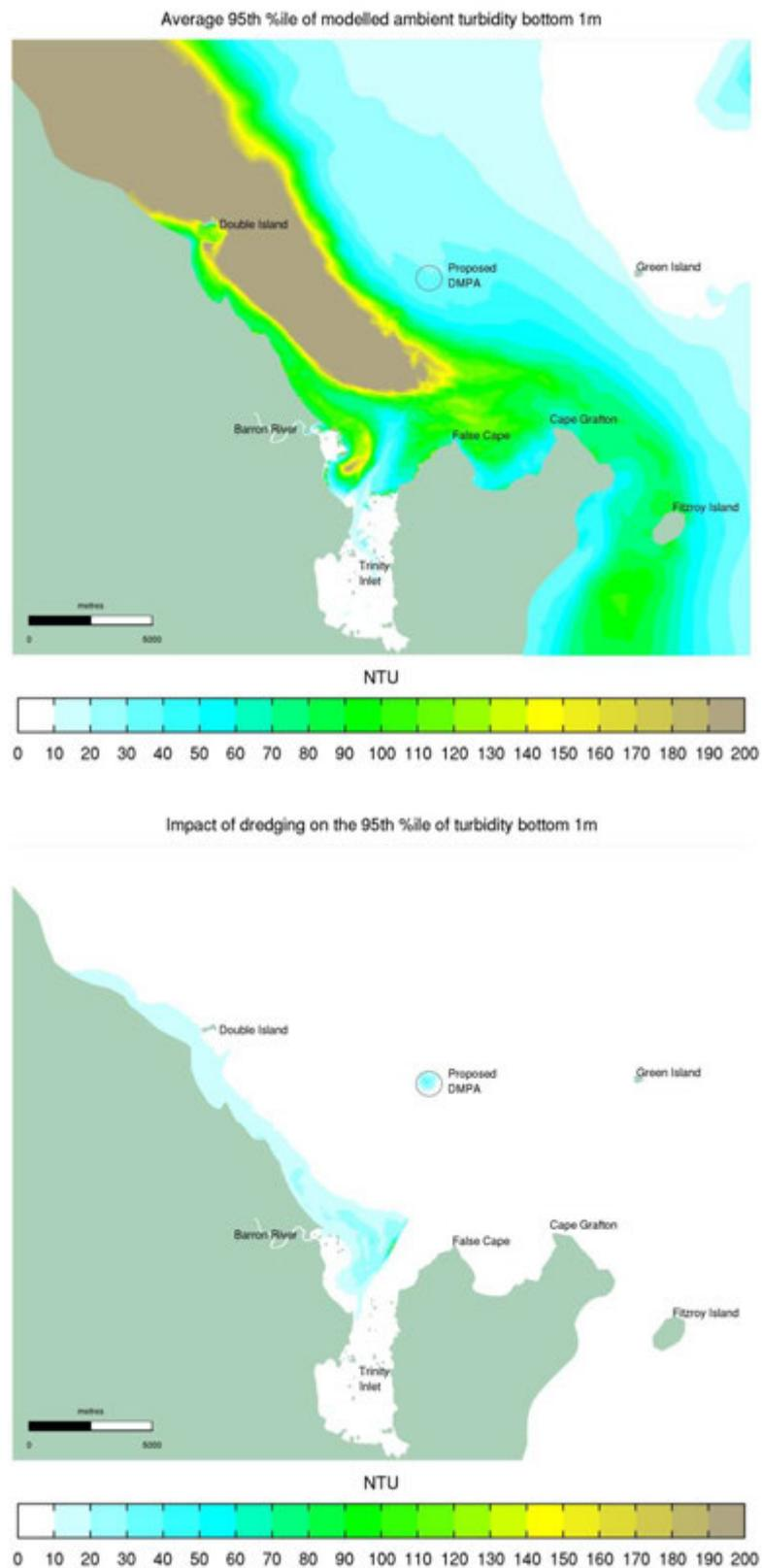
Figure 6-17 “Worst Case” Soft Material Dredging 95<sup>th</sup> Percentile Bottom 1m Turbidity: Average Ambient Turbidity (top), Impact of Dredging (bottom)
