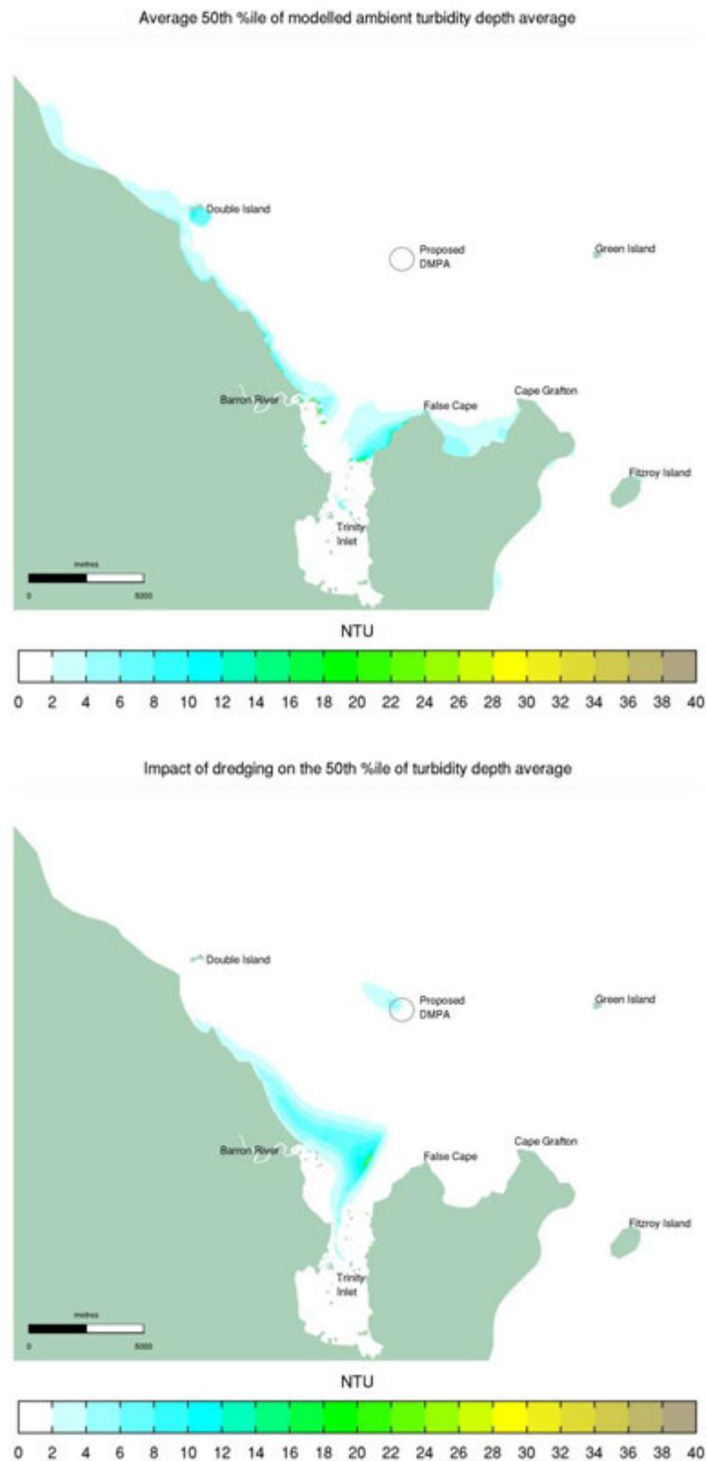
Figure 6-18 “Worst Case” Soft Material Dredging 50<sup>th</sup> Percentile Depth Average Turbidity: Average Ambient Turbidity (top), Impact of Dredging (bottom)
