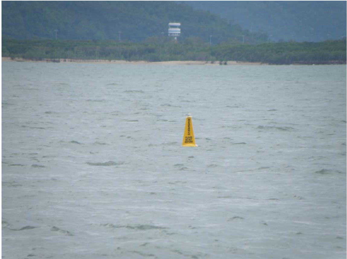
Figure A-6 Marker Buoy at Beacon C11 used to moor the Citadel CTD Instrument 1m below the water surface
