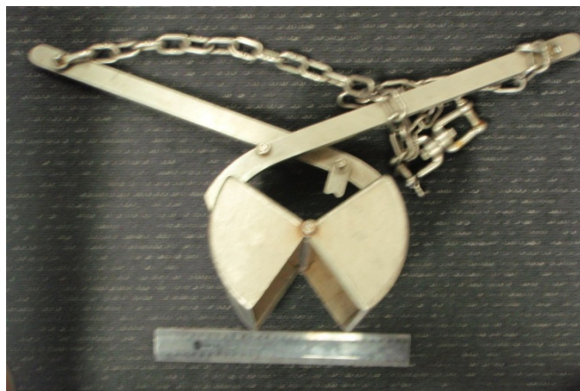
Figure A-7 Stainless Steel Van Veen Sediment Sampler used for Sediment Sample Collection
