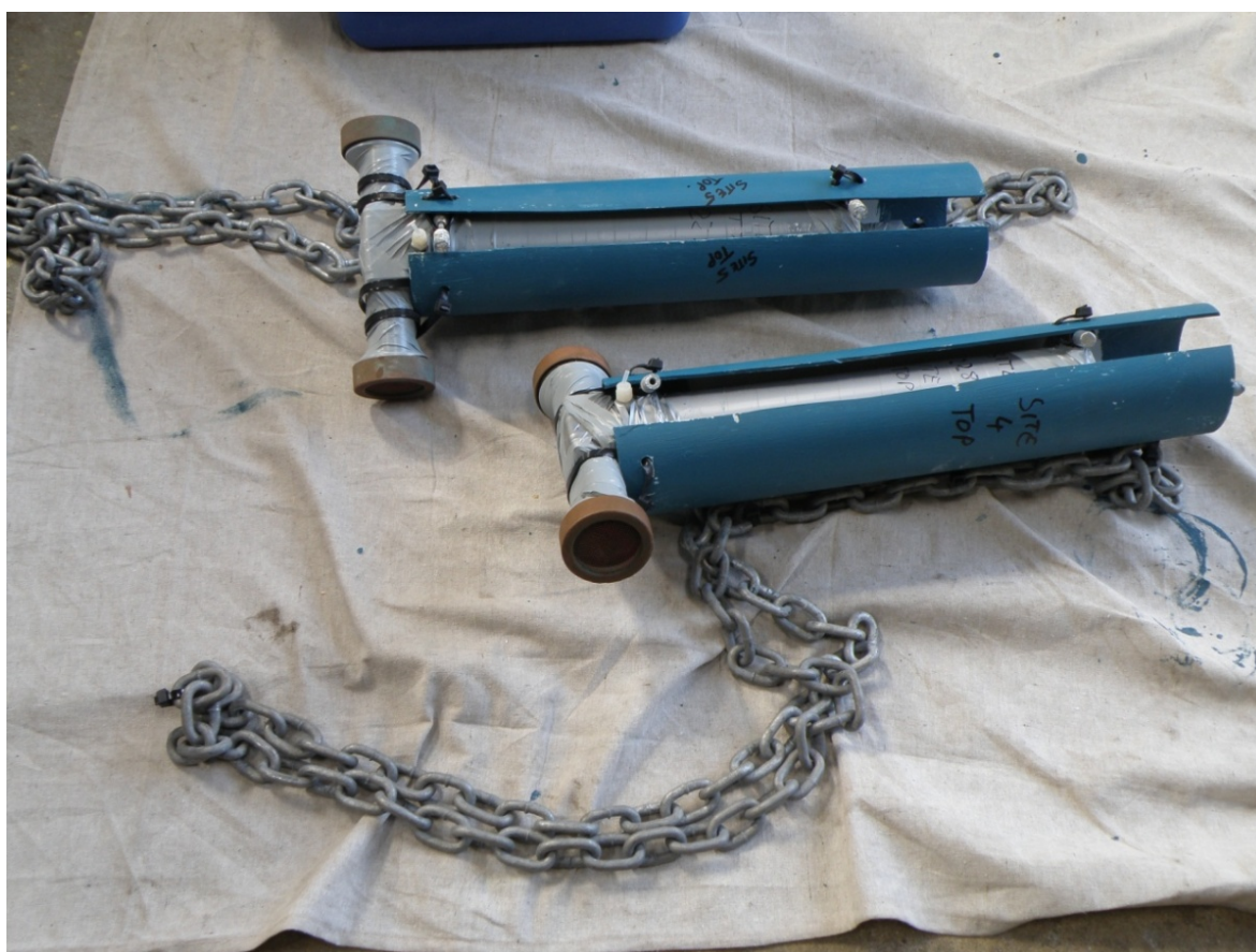
Figure A-5 Teledyne RD Instruments Citadel Model CTD-NH prepared for deployment at Beacons C7 and C11
