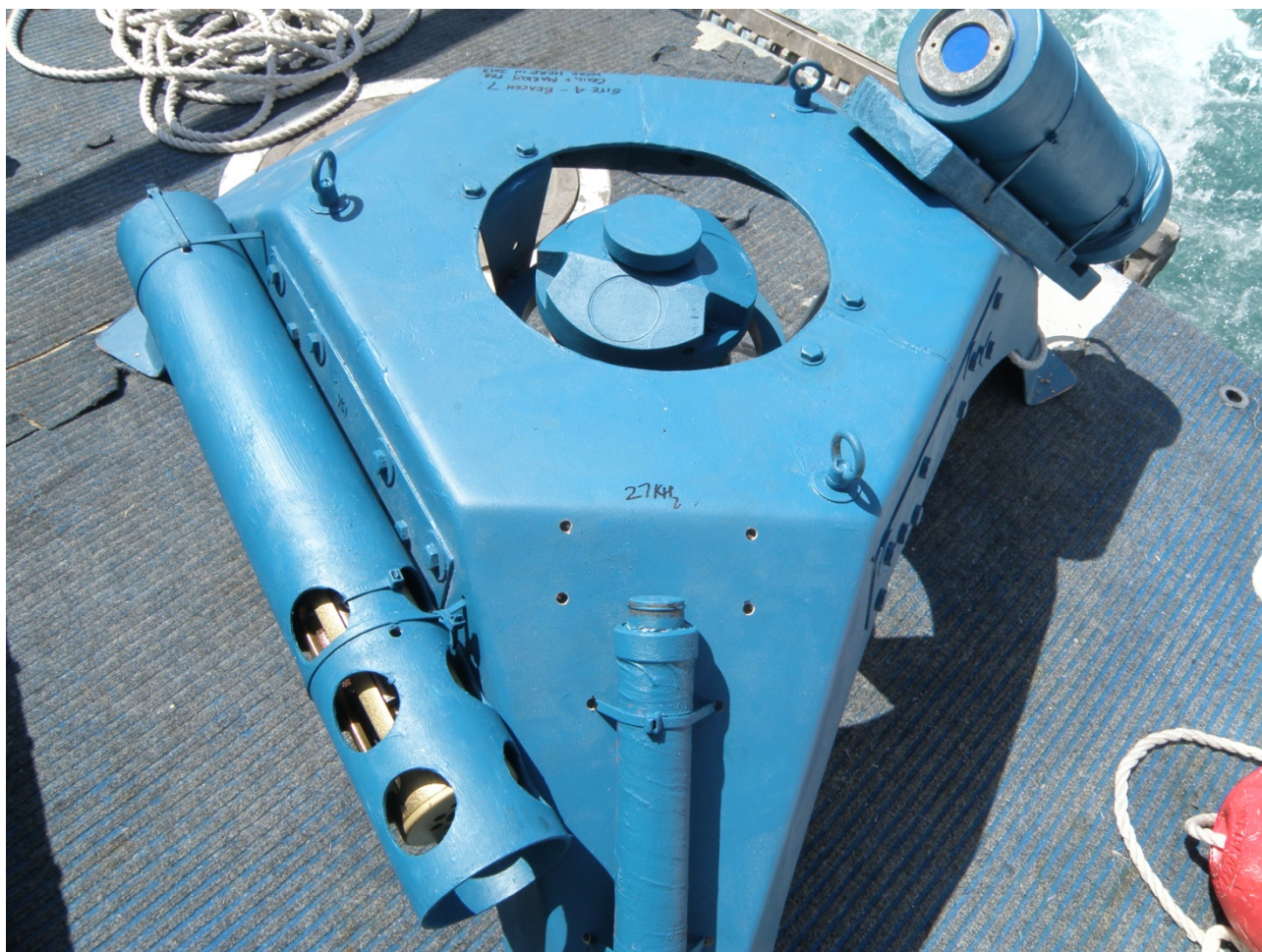
Figure A-3 Sea Spider frame equipped with 600kHz Nortek AWAC (Centre of Frame), AWAC battery cannister (right hand side) and YSI Model 6600 Water Quality Instrument (foreground left side) and acoustic transponder (foreground centre) ready for deployment at Site 4 - Beacon C7.
