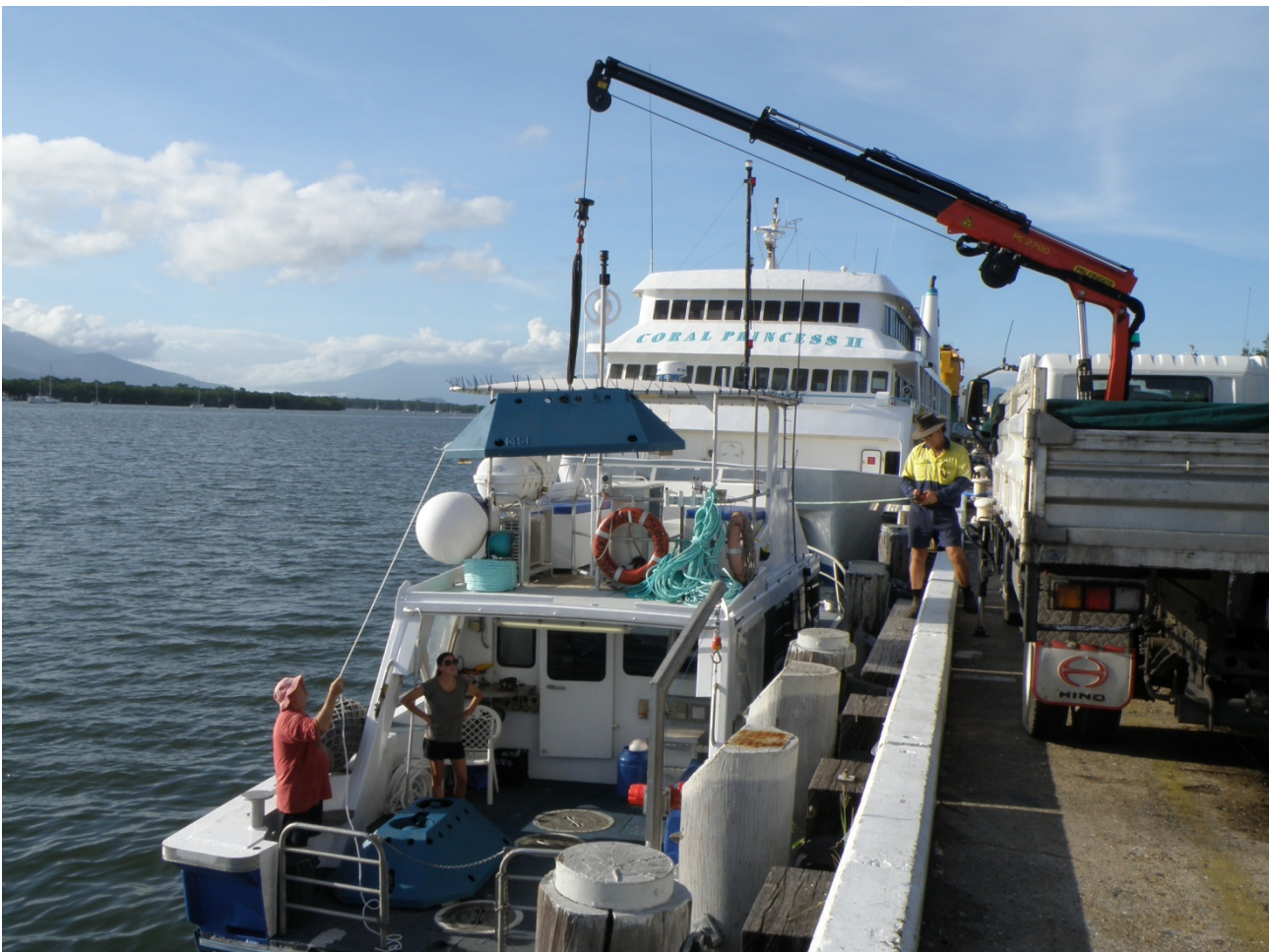
Figure A-2 Trawl Resistant Frames containing Nortek AWACs being positioned on survey vessel 'Viking' prior to deployment
