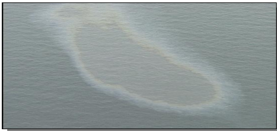
Figure 4: A photograph showing the difference between metallic appearance in the centre and the silvery and rainbow sheen oil around the edges. The thickness of the metallic is between 5 \mu\text{m} - 50 \mu\text{m} ; rainbow sheen is between 0.3 \mu\text{m} – 5.0 \mu\text{m} ; and silvery sheen is between 0.04 \mu\text{m} – 0.3 \mu\text{m} . The thickness of the (source: Bonn Agreement Aerial Surveillance Handbook, 2004 – Part 3, Annex A).
