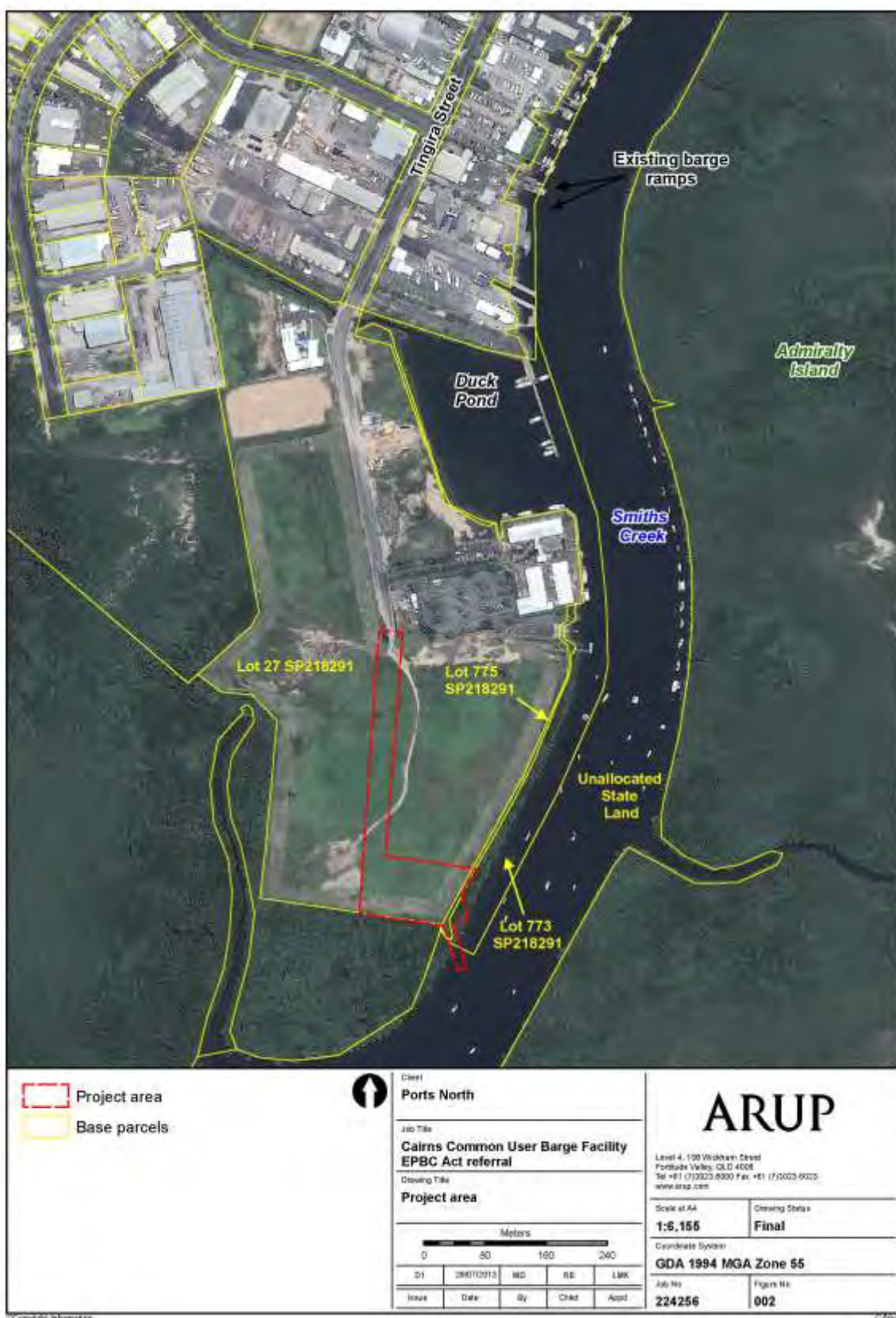
Figure 2: Extract of ARUP report showing CUBF project area (red outline, noting proposed ramp extending into Smiths Creek).
