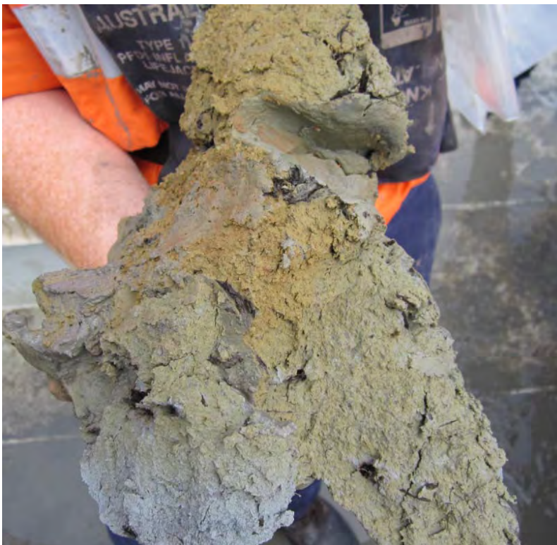
Plate 2 – Stiff Clays – non Acid Sulfate Soil
