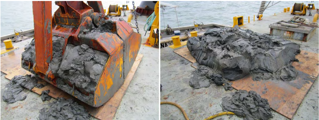
Figure 19: Photograph presenting material conditions at GS19 at 0 to 0.9 m depth
