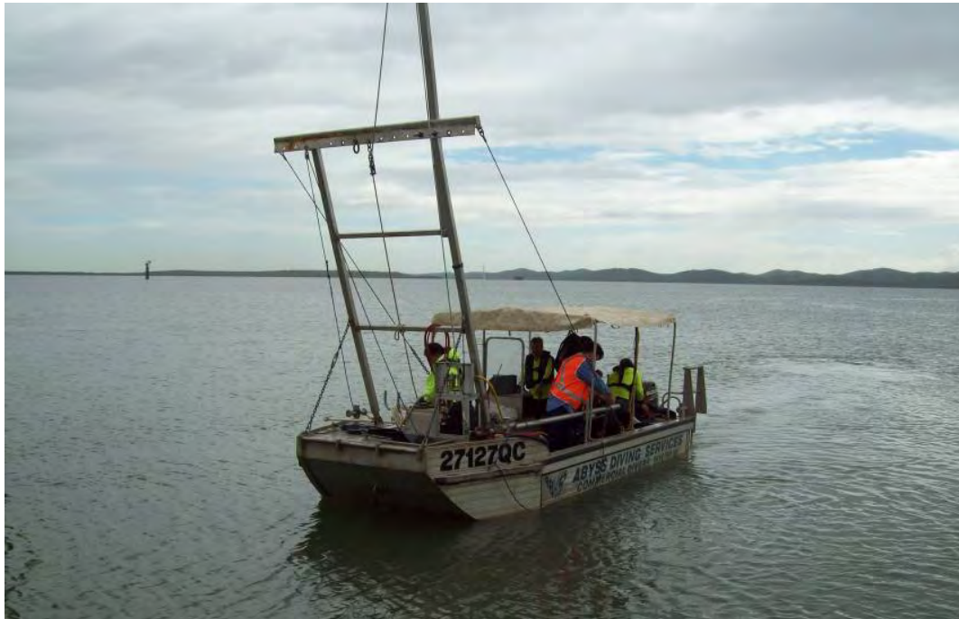
Plate 2-1 Vessel vibracore setup
