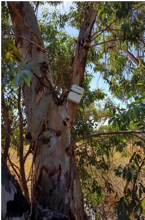
Figure 2: Song meter placement in tree
