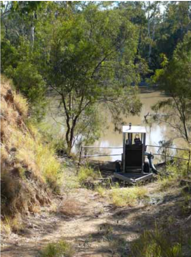
Plate 5-8. Movable irrigation pump drawing water from Glebe Weir on Lot 14 CP FT1
