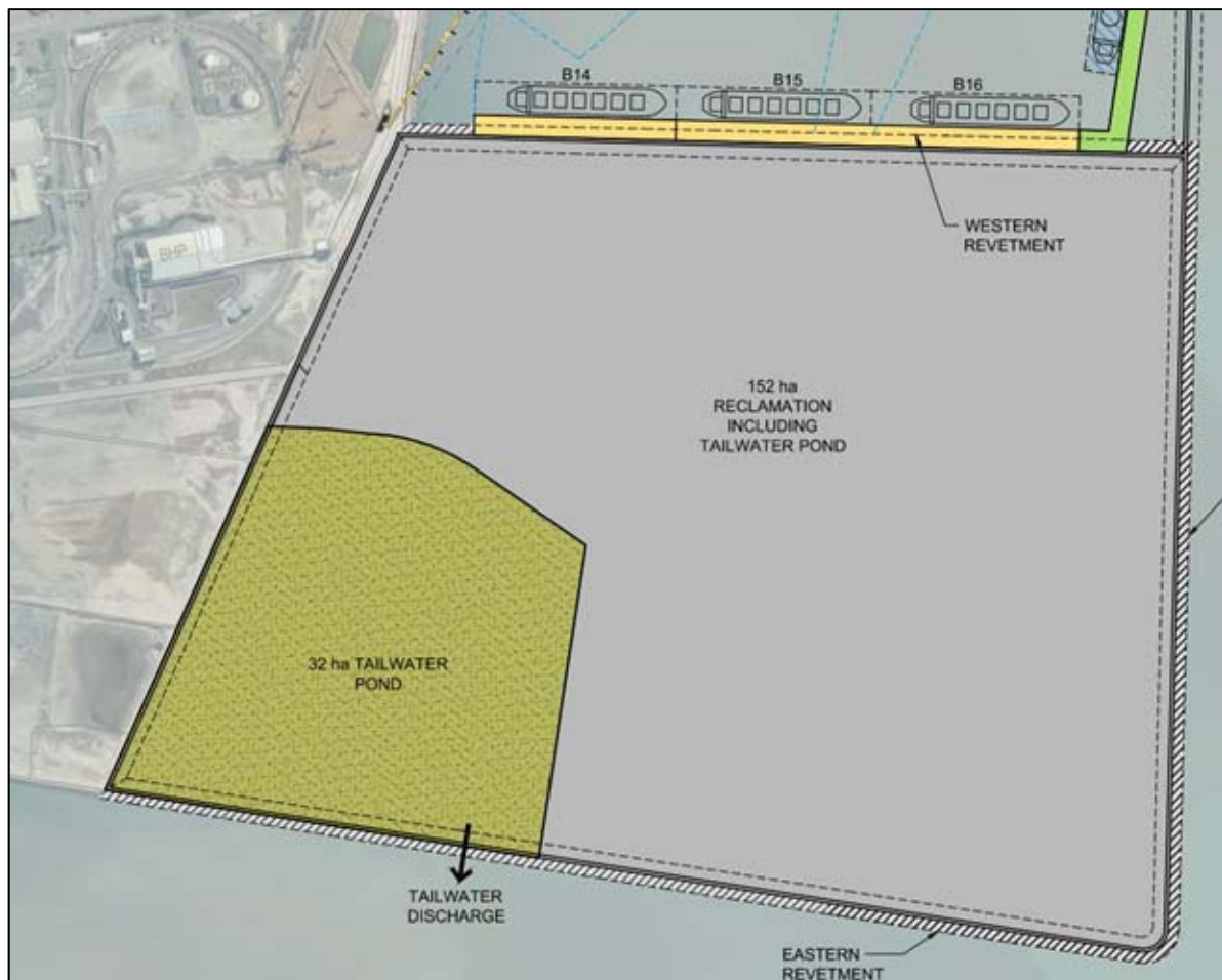
Figure 6.21 Tailwater Discharge Location from the Reclamation Area
