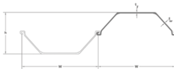
Figure 3: Sketch of the sheet piles possibly used at the TOT.
